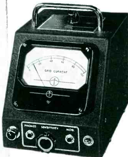
MODEL 59-LF OSCILLATOR UNIT Frequency Range: 100 Kc to 4.5 Mc. Price - Oscillator Unit (Head) only $98.50
