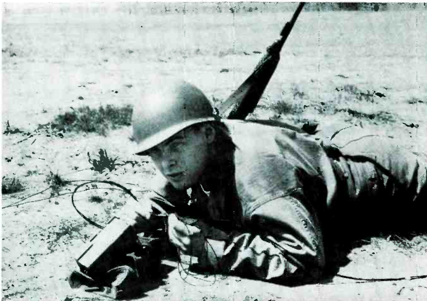
Transistorized version of telephone repeater enables a combat soldier to talk more than 30 miles. Total weight of the unit is 3.5 pounds
