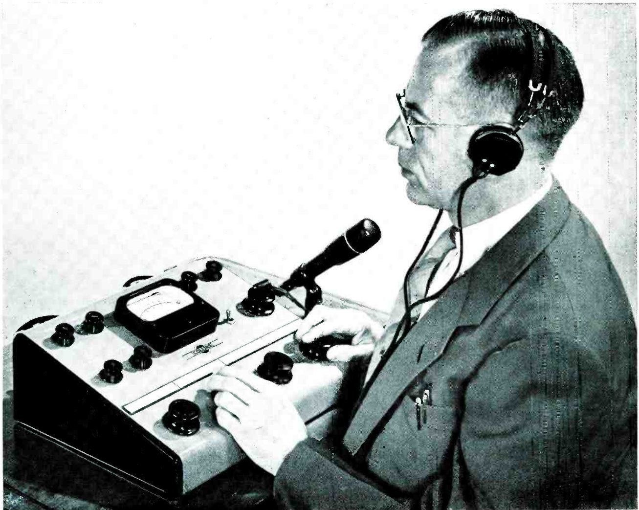
Operating engineer using the self-contained transistor remote pickup broadcast and public address amplifier
