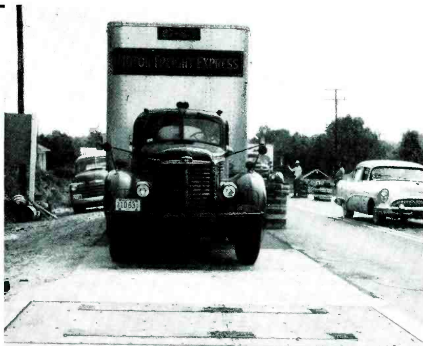
Weighing platform is set into roadway. Equipment is triggered by switch ahead of platform and shut off by another that follows. A permanent tape record shows the weight of each axle
