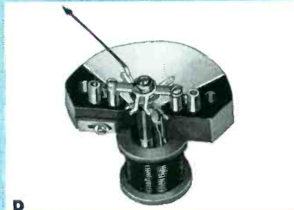
(D) MOVING VANE TYPE —The preferred movement for A-C measurement. Consumes remarkably little power. Features Simpson three-way balancing and patented balance weight locking clips.
