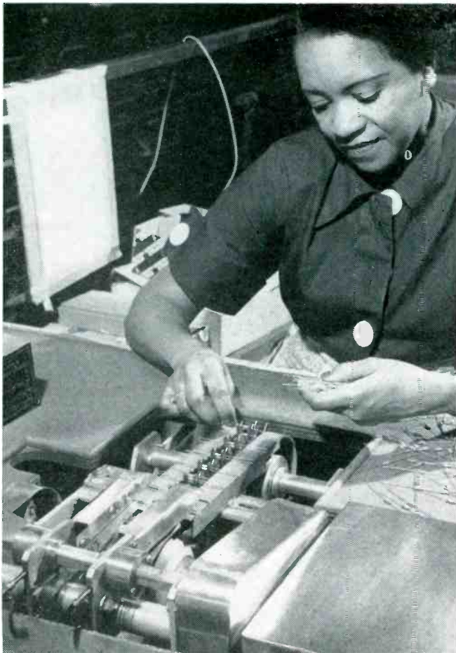
Loading resistors manually two at a time on motor-driven cutter
