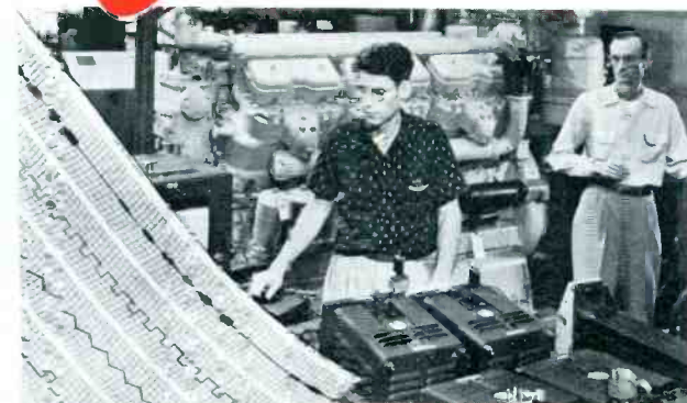
Torque of an engine balancer shaft is recorded by Brush instrumentation in this set-up at Caterpillar Tractor Co. Test data helped Caterpillar engineers reduce vibration, improve engine performance.
