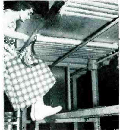
Floor-level view of under-bench wire-storing tubes
