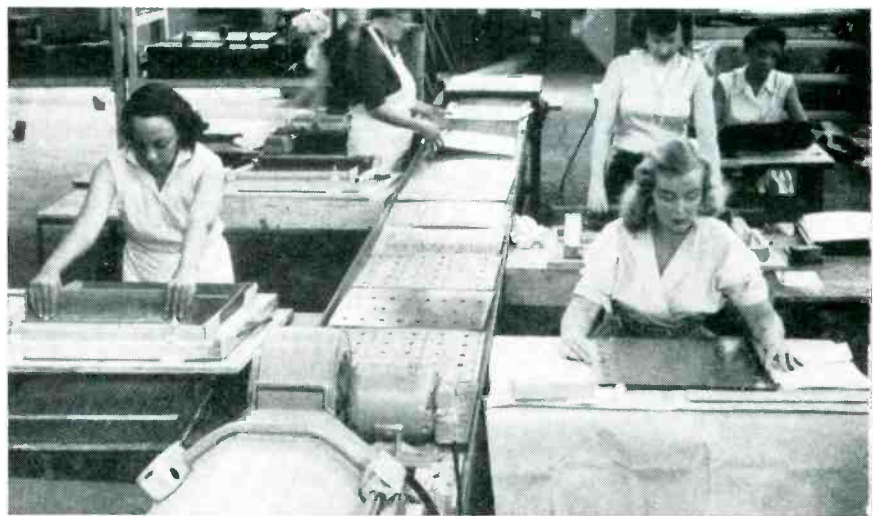
Silk-screen printing setup for etched wiring boards, with inspection position at right
