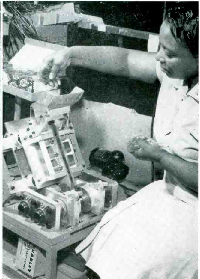
Loading resistors a handful at a time into IRC lead cutter
