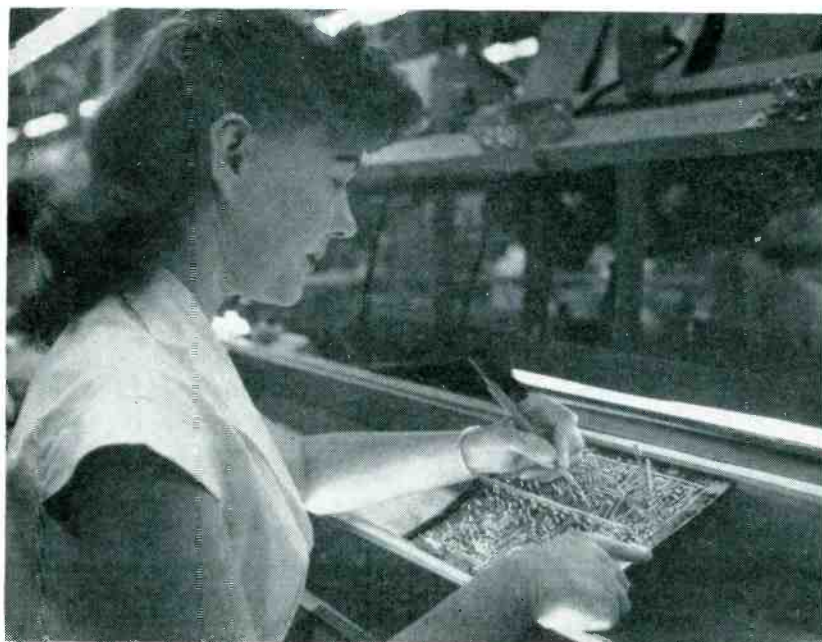
Clearing short between leads with probe tool at inspection position illuminated by fluorescent lamps above and below wiring board. Operator's right hand rests on shield of lower lamp while holding etched wiring board in pass-along line
