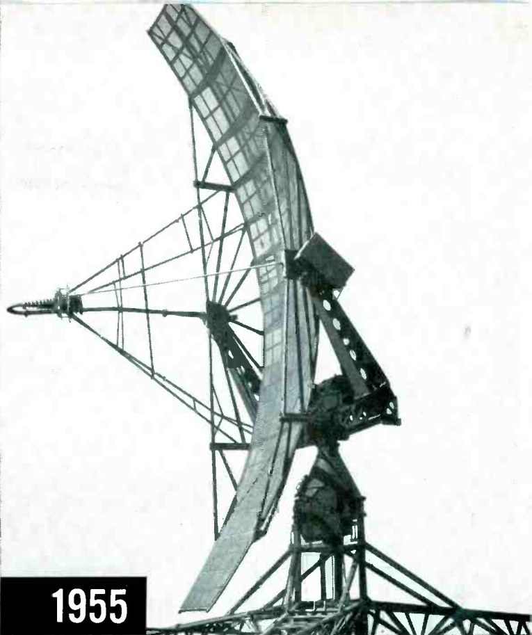
IN USE TODAY, this huge nodding height finder was designed and developed by General Electric to be used with powerful search radar systems and is a major contribution to long-range aircraft location.
