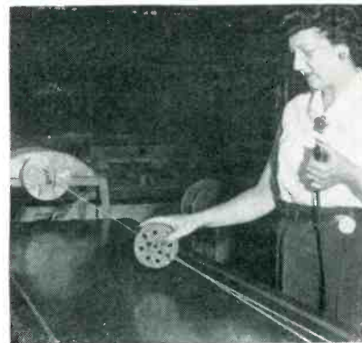
Operator holds motor switch in left hand and comb in right hand as she walks ahead of twists
