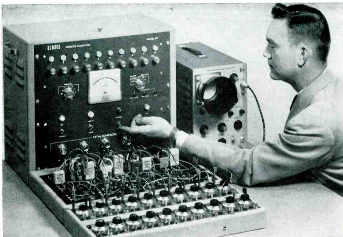
Solution of five-component chemical kinetics problem requires only five of computer's ten amplifiers
