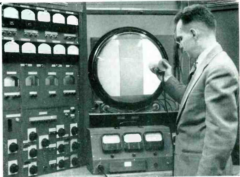
Color measurements are made by placing pickup head of colorimeter on face of operating tricolor tube and noting three meter readings
