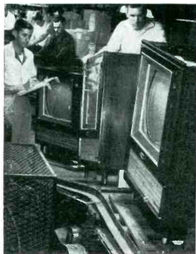
New 26-tube color-tv consoles on wood shipping pallets ride down slat conveyor at lower level and are pushed up over rollers on incline to start of next slat conveyor at higher level, for passage through screened and partially darkened final test rooms
