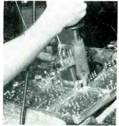
Soldering insures good ground to etched wiring by anchoring mounting screw permanently in position. The solder here doesn't reach the etched wiring itself
