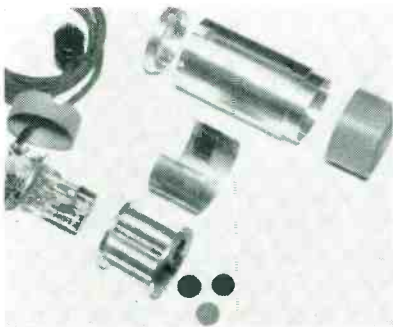
Internal construction of pickup head showing filters, phototubes and circuitry
