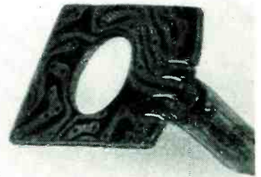
Method of soldering leads of subminiature tube to edge notches of board
