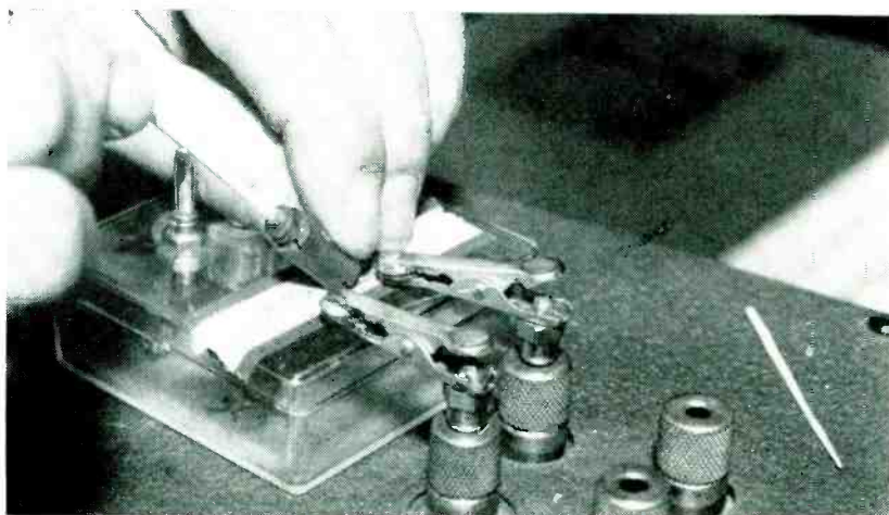
Using toothpick to adjust sintered iron core while measuring inductance at production test setups
