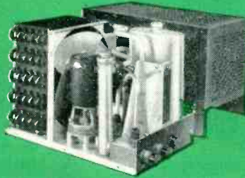
MODEL MB-175, TYPE 200 DISSIPATION: 2,000 watts. ALTITUDE RANGE: sea level to 50,000 feet. POWER REQUIRED: 28 volts D.C. WEIGHT: 25 pounds. SIZE: 10" x 15-15/16" x 10 3/4" high.
