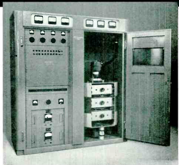
National Company two, ten and fifty kilowatt transmitters employing Eimac klystrons and circuit components are among the pace-setters in the revolutionary art of forward-scatter propagation.
