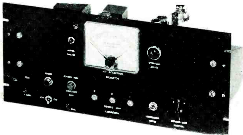
Indicating unit has provision for calibrating meter for three separate sensing units. Relay built into meter sets off alarm at preset ice-load level
