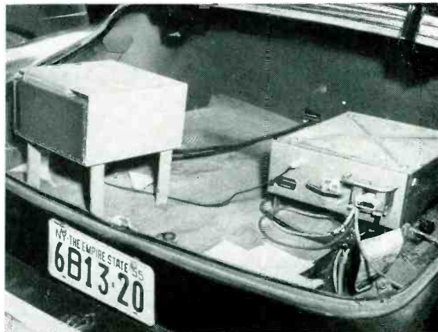
Meter on police-car dashboard records speed of passing car. Radar transmitter and receiver are mounted in trunk
