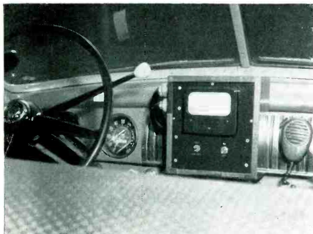
Meter on police-car dashboard records speed of passing car. Radar transmitter and receiver are mounted in trunk
