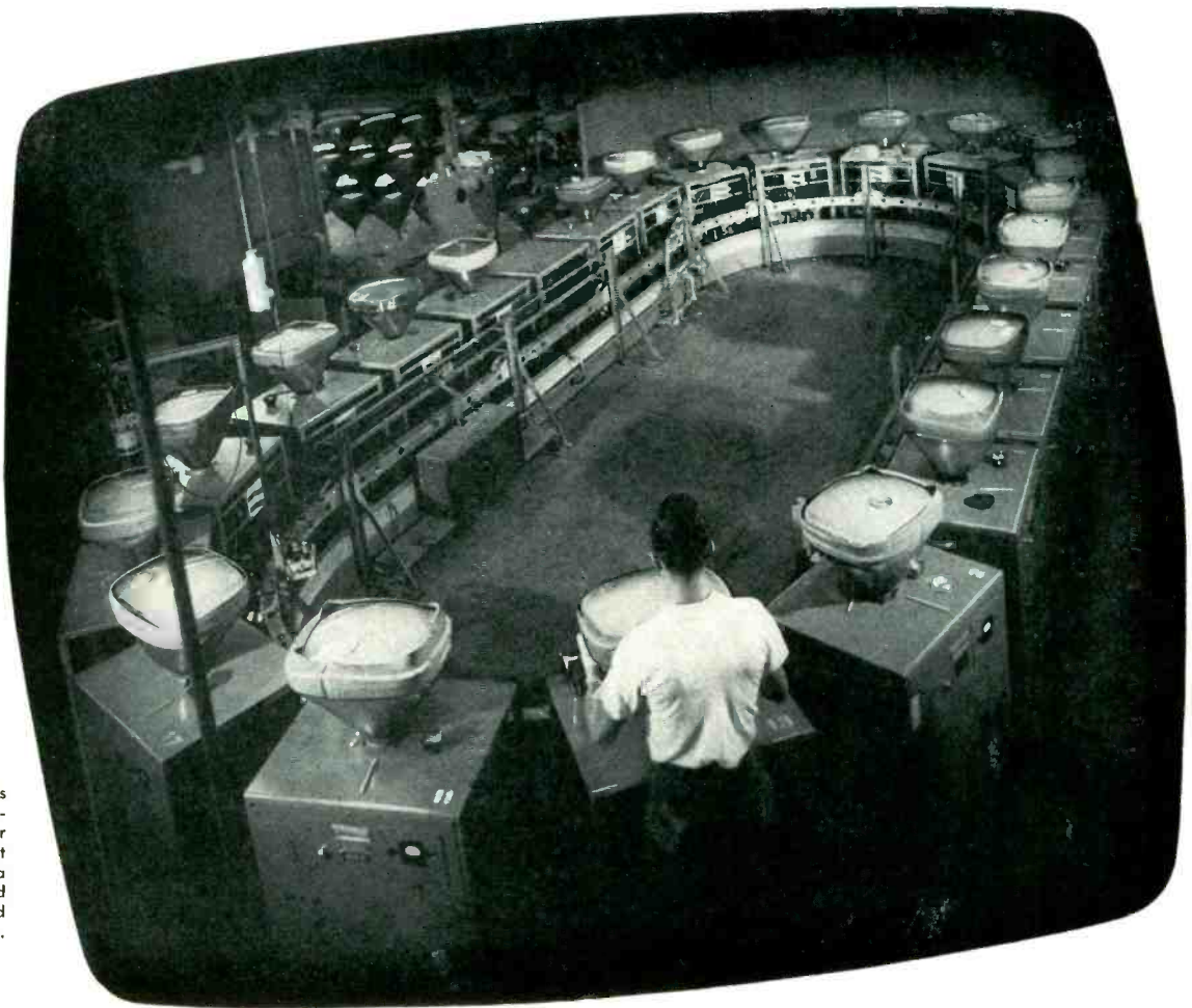
Overall view of Stokes continuous vacuum metallizing dolly system for aluminizing TV tubes at RCA's Marion, Indiana plant. Operator is required only to load and unload tubes from the 22 carts.
