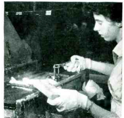
Immersing board in first soldering pot. Cake of beeswax in left hand will be wiped over next pot before transferring board to it
