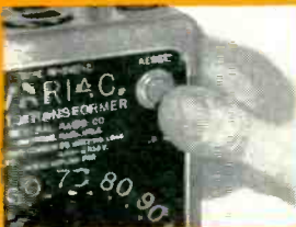
Flip-on-type manually reset thermal overload breaker provides protection from prolonged overloads
