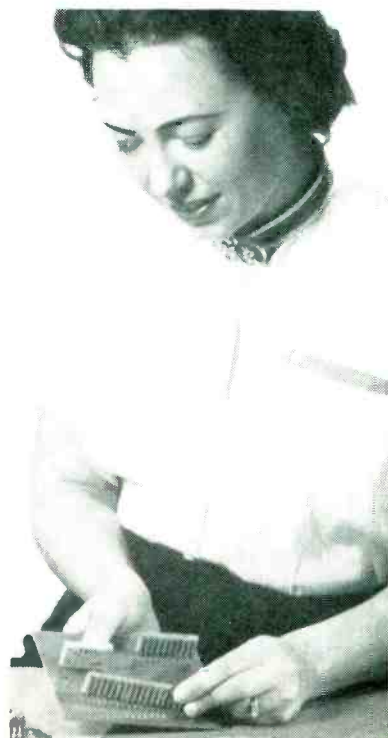
Finished modules are easily inserted in punched holes of etched wiring board
