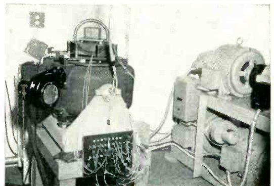
Shaker and power supply located in soundproof room has frequency range of 0 to 2000 C.P.S. Complete with automatic servo control of acceleration and frequency cyler.
