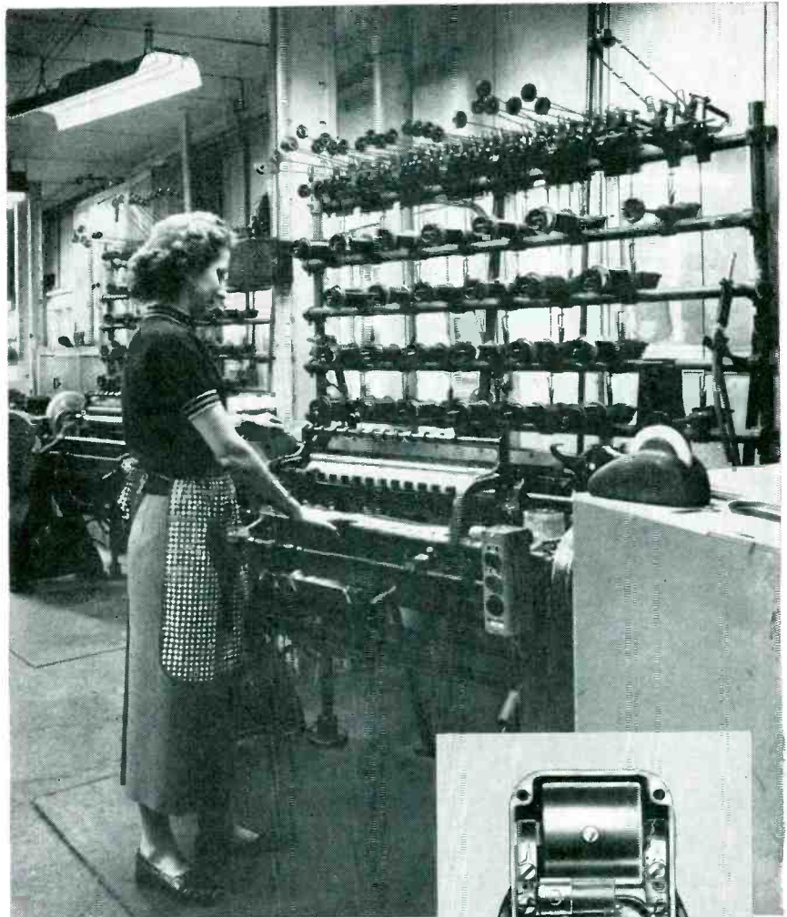
New Leesonas No. 107 Automatic Coil Winders, shown in the plant of Wico Electric Company, West Springfield, Mass., were selected because of this firm's long, satisfactory experience with Leesonas machines. Leesonas No. 107 Winders, featuring speed and accuracy in automatic winding, are enabling many plants to boost production and cut costs. Inset shows a cutaway of a Wico Model XH Magneto. Coil at top of it is precision wound on Leesonas No. 107's.
