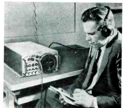
Compact adf comprises receiver and indicator dial
