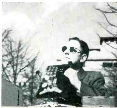
Bell Labs engineer, D. F. Ciccolella compares solar battery with Eppley pyrheliometer that measures total solar radiation available
