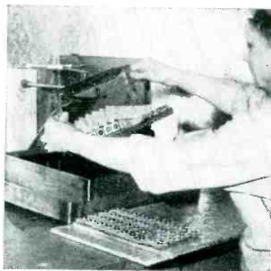
Placing basket on angle support for quick draining after dipping in clear glyptal
