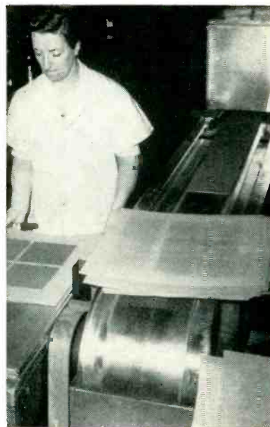
Output of sifting conveyor, showing how plates are arranged in groups of four on cardboard-covered aluminum tray in preparation for fusing the selenium powder
