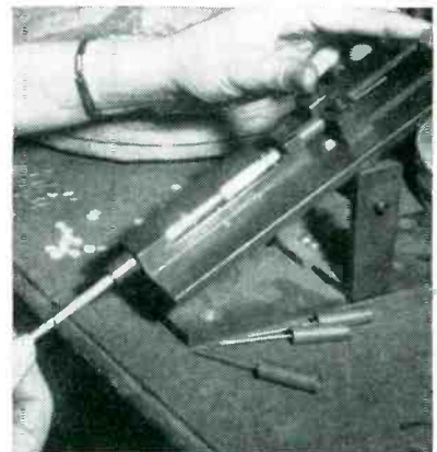
Bringing up plunger to push pellets into tubular cardboard housing. Fixture is then tipped backward so that housing can be removed without spilling
