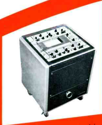
Oscillographs can be mounted in a mobile instrument cart or used on a test bench. Oscillograph has 7" x 19" panel, 10½" overall depth.
