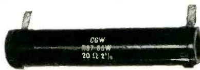
Corning Type R High-Power Resistors—Range from 25 to 1,000,000 ohms, ratings from 7 to 115 W, are non-inductive. Exceptionally good noise and frequency characteristics. Excellent moisture resistance and overload capacity recommend them for stable long-life service under adverse conditions. Meet MIL-R-11804A Specs.
