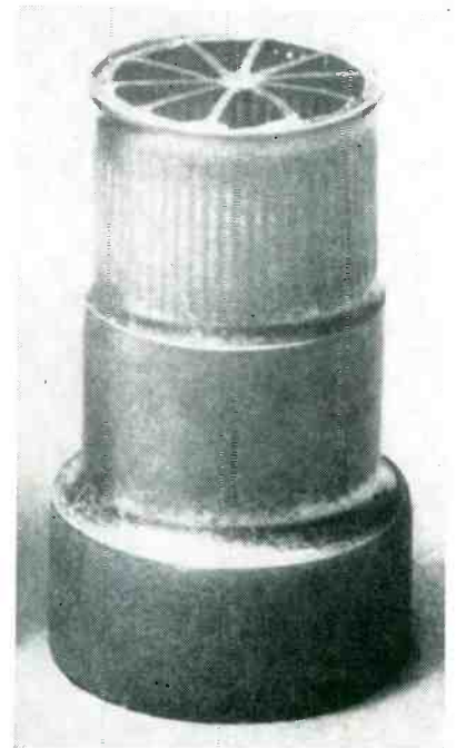
Partially completed grid is foil-like cylinder having thicker longitudinal ribs along inner surface. Ribs become grid strands when web is etched out
