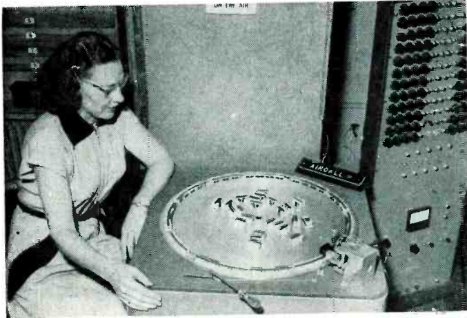
Announcing machine for one-way radio paging uses magnetic tape affixed to numbered Nylon block. Experimental tone-coded keyer at upper right
