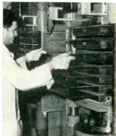
Inserting tray of rectifier plates in hot press
