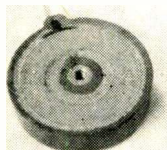
FIG. 1—Center-threaded brass insert of toroid allows coils to be stacked without applying mounting pressure to plastic case or coil assembly
