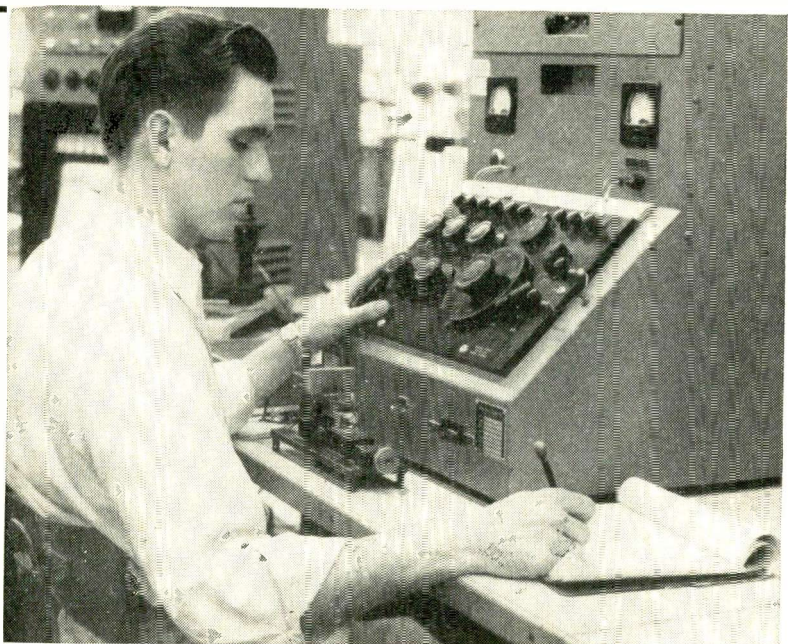
FIG. 3—Checking grown crystal for width of p-layer and resistivity of n-regions. Operator is performing a four-probe resistivity measurement
