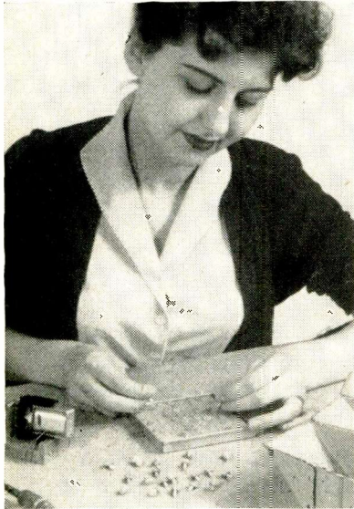
Placing washers on bolts two at a time with aid of sponge rubber pad
