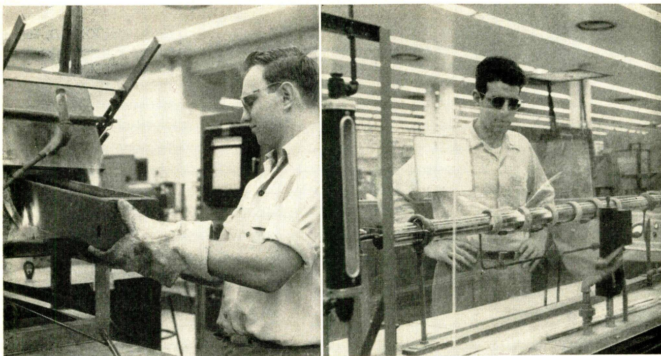
FIG. 1—Reduction of germanium dioxide is accomplished under hydrogen atmosphere in 600-C electric furnace (left). Temperature is then raised to 1,000 C to produce ingot. Zone melting (right) provides high-purity germanium. Six induction-heating coils melt germanium in long graphite boat
