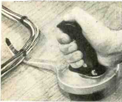
Third, operator presses button on grip to actuate spring steel cutting blade that cuts tape, then pulls gun out
