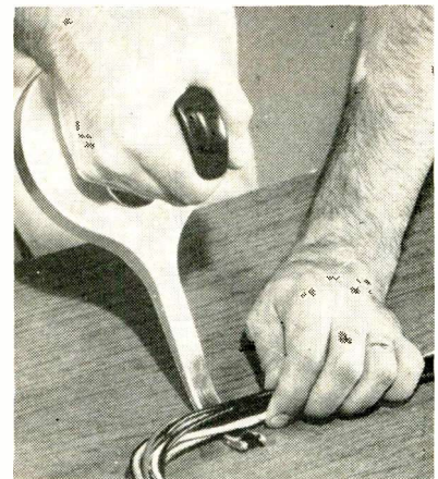
Second, tip of gun is pushed under cable to draw tape underneath
