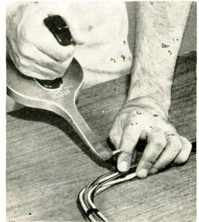
As first step in using gun, end of tape protruding from curved tip is pressed over wiring
