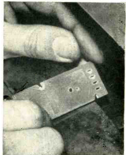
Loading sheet on machine in preparation for attachment of leads through rectangular slots at right on copper-clad plastic strip
