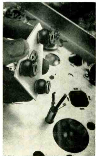
Collet-type tool in position for pulling shock mount through chassis hole for socket plate held in hand
