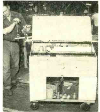
Plumber's maintenance dolly in picture tube plant
