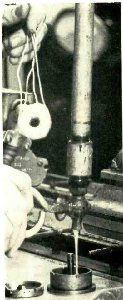
As first step in plastic coating, operator removes preheated mold from conveyor and preheated toroid from oven. Toroid is dipped in plastic and permitted to drain while mold is filled with plastic to the three-quarter mark
