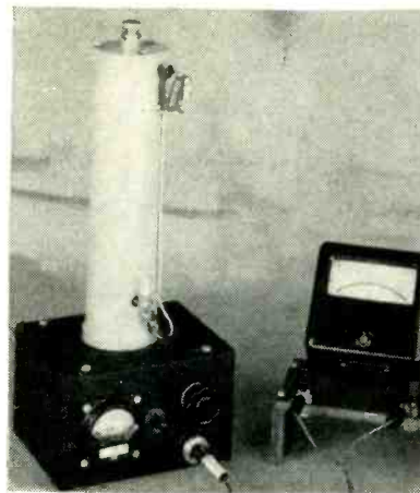
FIG. 2—Cavity resonator transistor oscillator operates at frequencies as high as 350 mc
