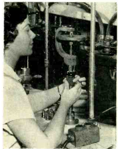
Rotating knurled sleeve to move pulse plug up and down during sealing to glass section of magnetron by induction heating
