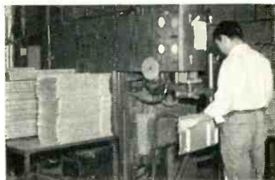
PRODUCTION FACILITIES include such modern equipment as this 100 KVA spot welder, accurately timed for welding aluminum.
