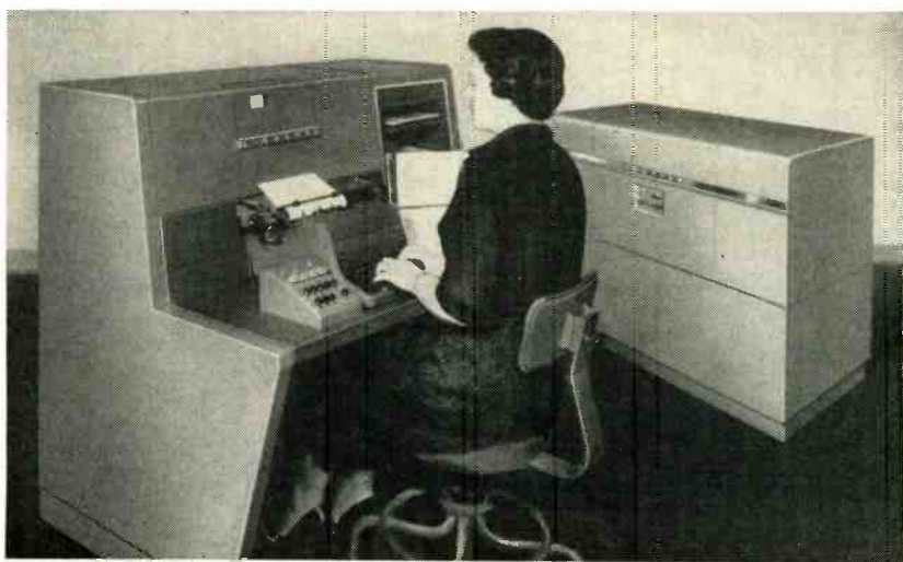
Two-unit typesetter uses electric-typewriter keyboard to punch paper tape for controlling photographic unit at rear. Control panel at side of typewriter is for selecting style of type and word spacing
