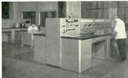
Rotating and indicating standards test benches with test lead storage cabinets at each end.
