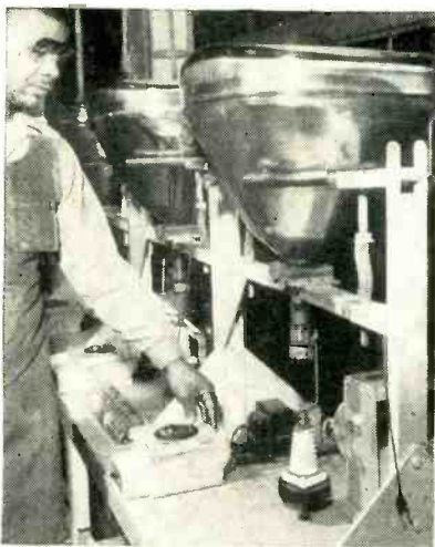
Pushing start button of timer to initiate automatic sparking during final processing of picture tubes
