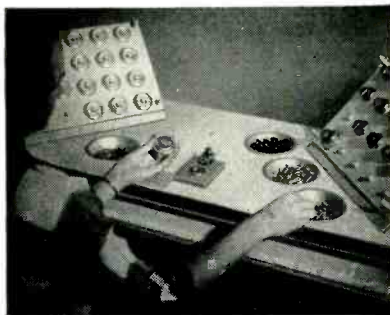
Bench setup having recesses for parts pans. Assembly jig is fastened to bench
