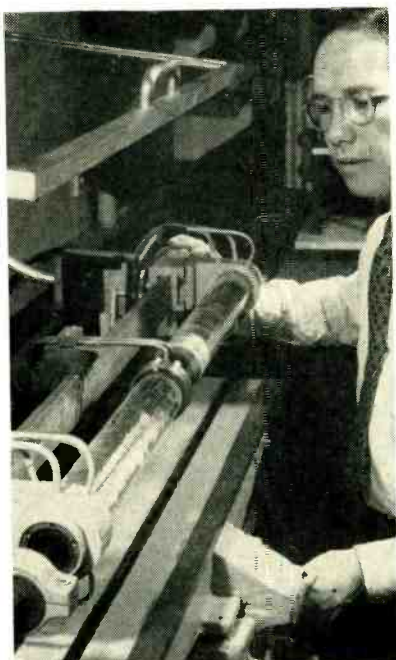
Zone-melting setup for refining germanium
