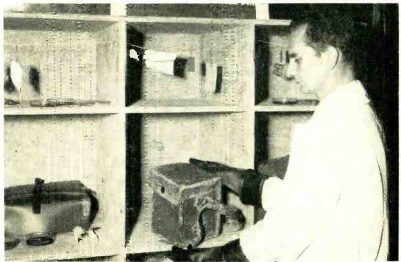
Two-week exposure in tropic test chamber at Signal Corps Engineering Labs, Fort Monmouth, N. J. has left untreated leather case covered with fungus. Specifications for manufactured equipment now reflect experience of tests.
