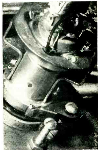
Finished turret in holder, showing how indentations in top plate provide clearance for grounding terminal lugs of socket. The entire holder is mounted on shaft going through slanting base, for rotation past detent spring in foreground
