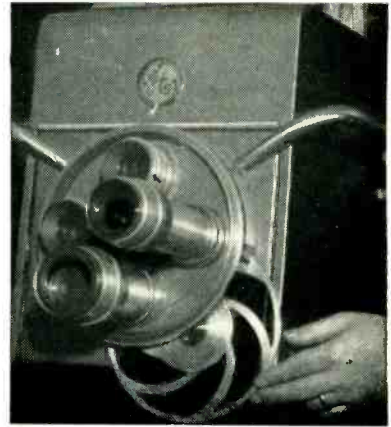
CBS-type color tv camera built by GE uses field-sequential disk. Chromacoder converts signal to NTSC color.
