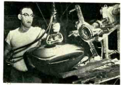
Lifting aid using air motor hoist and two ordinary vacuum cups that do not require a vacuum line. The three hoses control the air-type hoist motor overhead. At right is the vacuum-type spinning chuck
