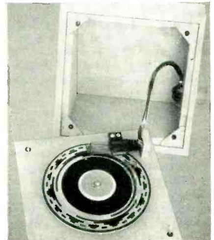
FIG. 3—Shaft-position coding switch and tone oscillator assembly. Open view of switch (right) shows binary-coding commutator rings
