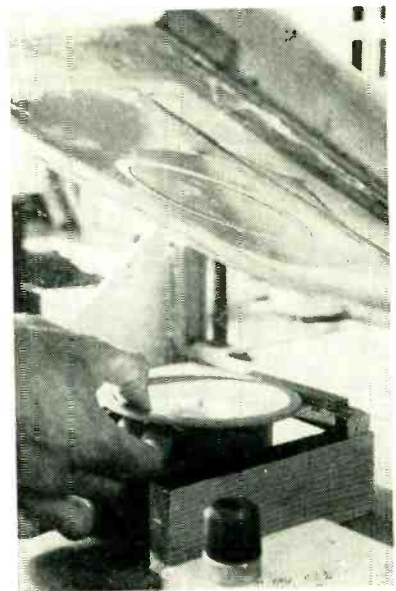
Silk screen permits quick, even application of green kitchen enamel as flocking base on bottom of waveguide stand. Enamel works well in silk screen, gives rich color to the green flock
