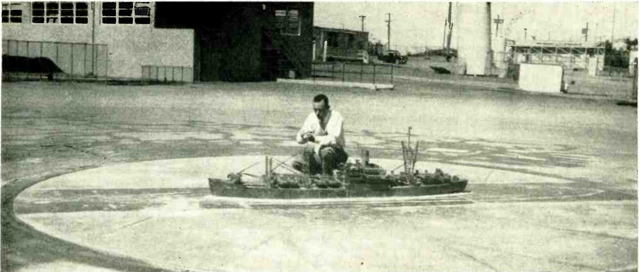
Scale model of USS Mount McKinley being tested at scale radio frequencies to determine directivity effects caused by ship's structure
