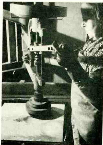
Polishing copper-clad plastic sheet with rotary scrub brush in drill press arrangement that is free to move horizontally as well as vertically
