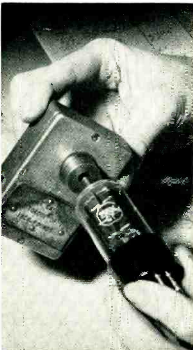
Top-cap torque-tester used on production line. Cap is rotated counterclockwise while inserting in hole, then rotated clockwise. This causes an off-center roller inside, spring-pushed in a clockwise direction, to wedge between the cap and the hub for gripping the cap
