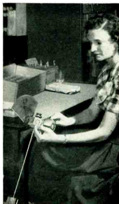
Setup for torque-testing tube bases to determine adhesive qualities of cement. Brass block on tester has hole arrangements for six different types of bases
