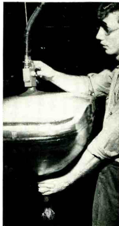
Lifting aid employing single vacuum-powered suction cup in conjunction with counterbalancing system employing motor-driven fluid transmission. Thumb of operator is on trigger button which is pushed to release vacuum after picture tube has been transferred to a rack or a conveyor cradle
