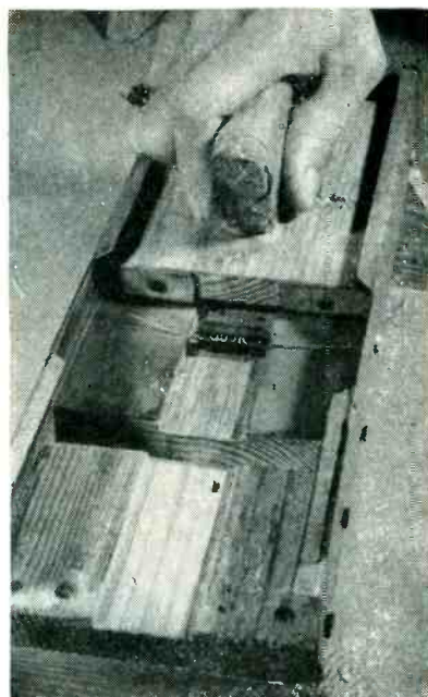
Resistor in straightening device just before operator rolls slide over its leads to straighten them
