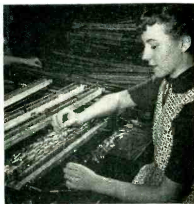
Capacitor bodies are inserted in tubes and ends of leads bent over rods to insure proper centering
