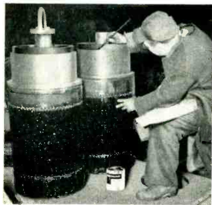
No. 32 Red Enamel is brushed on windings to protect them from oil
