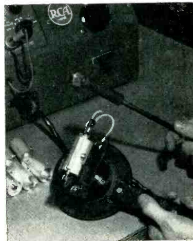
Tapping completed cavity unit with rubber hammer as part of final test
