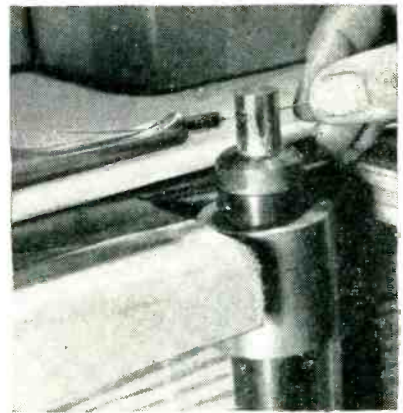
Closeup view of final flaring operation
