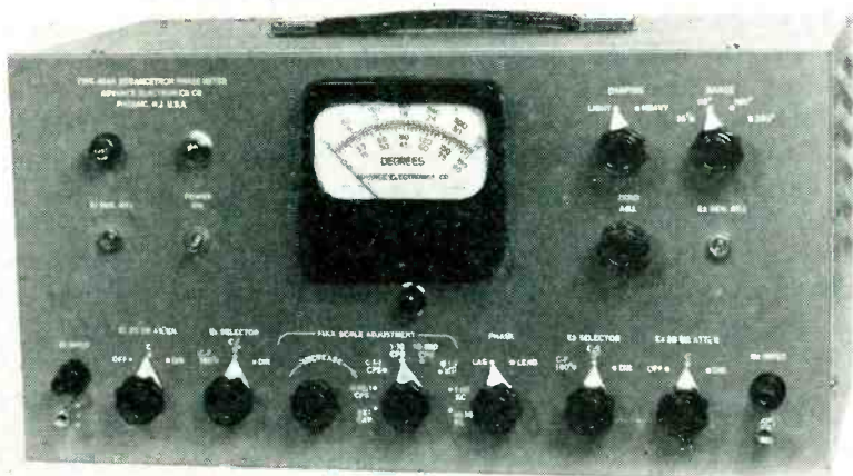
Front panel of type 404A Advancetron phase meter. Input jacks for waveforms being compared are at either end of panel. Controls next to each input provide for inserting 20-db attenuation and 180-degree phase shift. Indicator is 200- \mu a meter movement with 0.36, 0.90, 0.180 and 0.360 deg ranges
