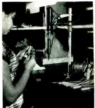
Pulling r-f filter assembly into housing. Soldering iron holder on bench is made from pipe and pipe fittings. Holder for solder spool is U-shaped piece of scrap iron screwed to bench, with spun-on terminals projecting inward from ends to serve as shaft. Solder spool is removed by spreading end supports apart
