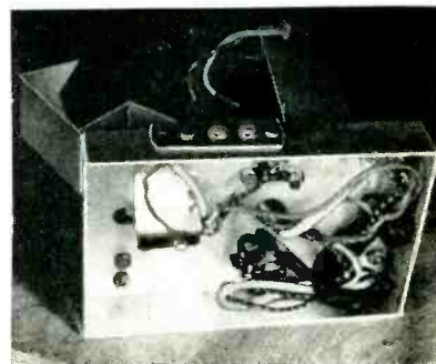
Bottom view of chassis for soldering iron holder
