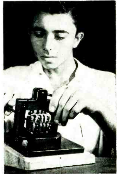
Relay holding fixture, designed to provide optimum working angle for tightening alignment screws
