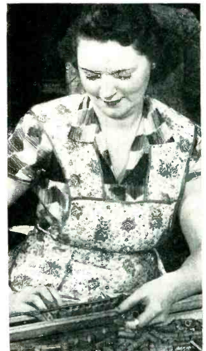
Placing capacitor tubes in jig. A wooden strip on the table beneath the rack keeps all the tubes at the proper height until thumbscrews are tightened
