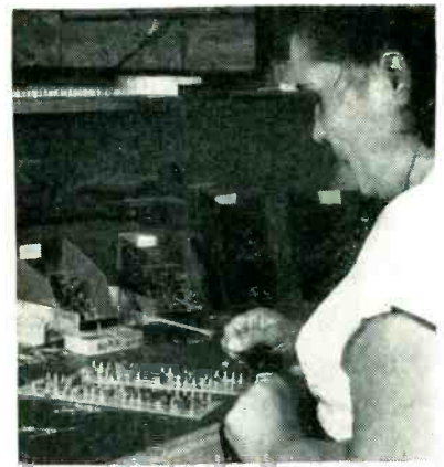
Operator can drop components quickly over terminals on board when leads have preformed loops
