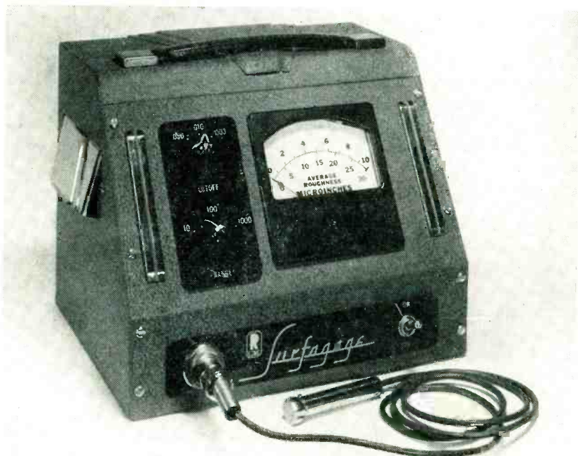
Roughness gage provides five roughness ranges and three cutoff frequencies
