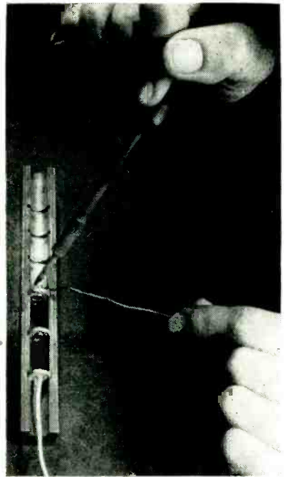
Fixture used for holding disc capacitors in position while soldering to spiral coils. Empty grooves at top are for another type of filter
