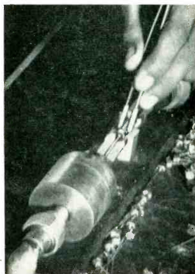
Removing capped resistor from fixture at air-vise setup, using tweezers having jaws wrapped with adhesive tape to prevent scratching of deposited carbon coating on ceramic body
