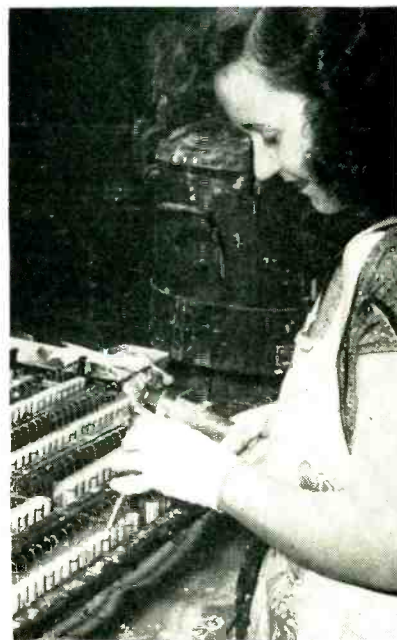
Squirting cement into ends of tubular paper capacitors with high-pressure cement gun. Racks are inverted for filling other ends of units
