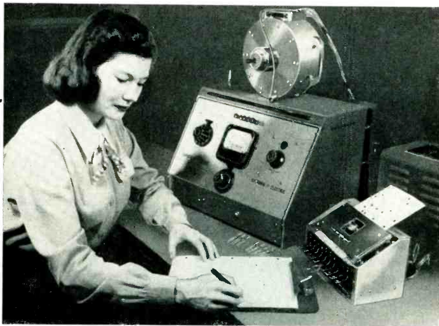
Punch-card controlled bridge being used to measure interelectrode capacitances in subminiature tubes. Variety of adapter units permit measurements on all types of tubes
