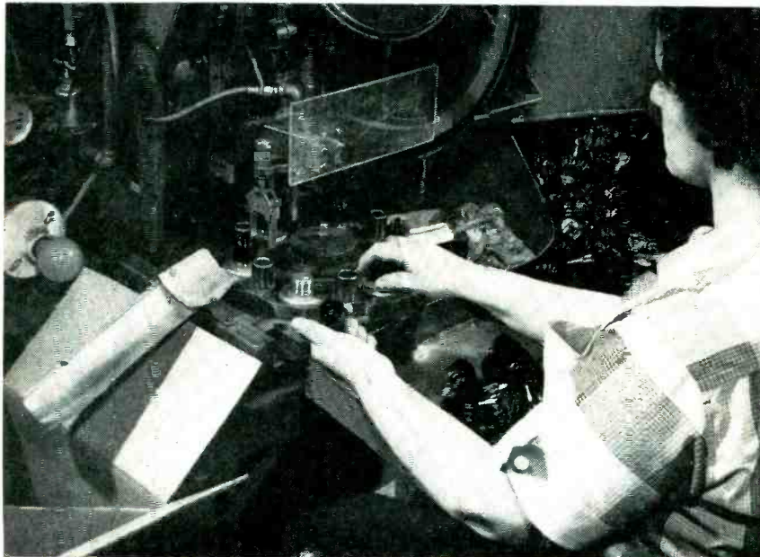
Loading tube base upside down onto tapered die of automatic inspecting machine
