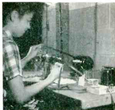
Voltage of pencil-type soldering iron is automatically reduced 1.3 v when iron is placed in holder on bench, thereby minimizing pitting of soldering iron tip when not in use. Operator uses iron here for soldering Nichrome resistance wire to terminals on ceramic bobbins for precision resistors
