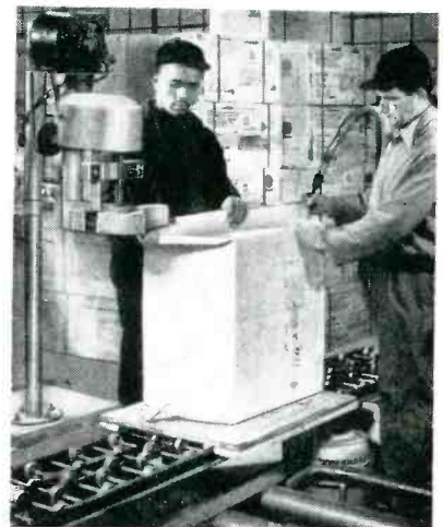
Removing air and moisture from carton bag before final heat-sealing on machine standing over conveyor. Vacuum cleaner is under conveyor
