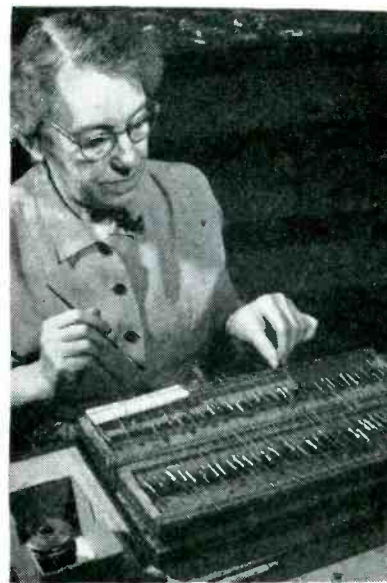
Springs on edges of rack prevent capacitors from coming in contact with each other while varnish coating is drying
