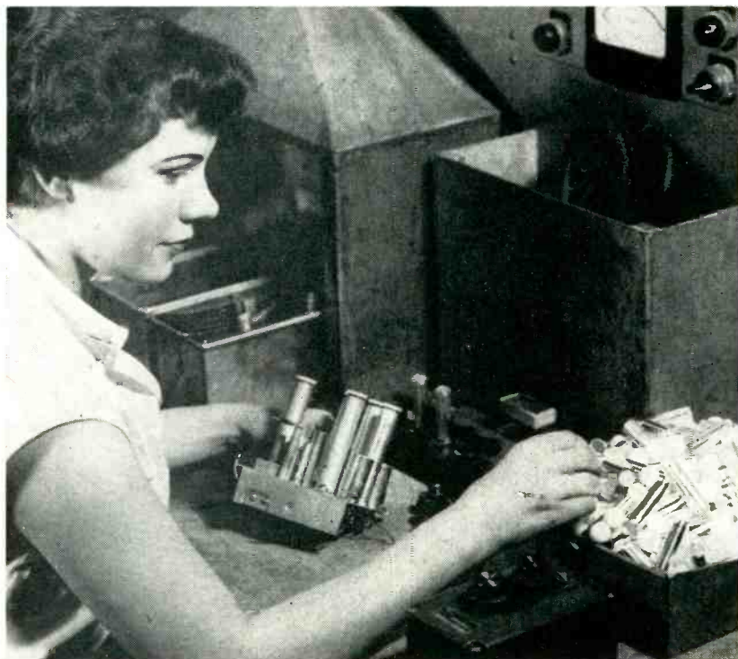
Transferring silver-plated cavities from moth balls to soldering fixture built around work coils of induction heater controlled from pushbutton station at right on bench. Finished units go into vhf two-way radio tuner in operator's left hand
