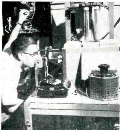
GROWING of single germanium crystals comprises final step in germanium preparation. Subsequent process is sawing
