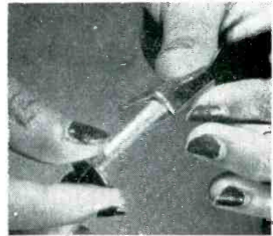
Applying split acetate sleeve to iron core-bobbin
