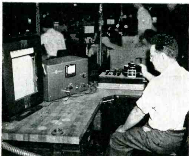
As a Null Detector The d-c Amplifier is being used above for factory checking and calibration of instruments.
