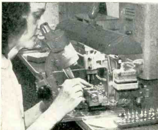
ASSEMBLY of point-contact transistors is accomplished using high-power microscope and micromanipulator to set contacts at a tolerance of 0.00025 in.
