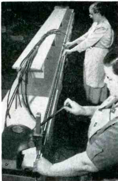
Cutting multiple-conductor cable with arbor press while second operator holds end of cable against stop in precision length-measuring trough
