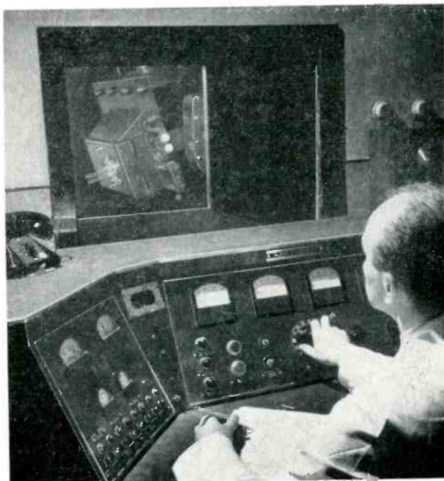
Betatron control room has water window through which operator can watch patient under radiation. High-energy x-ray beam makes possible treatment of deep-seated tumors with minimum damage to surrounding tissue
