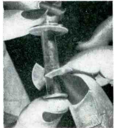
Placing split laminated washer over insulated core
