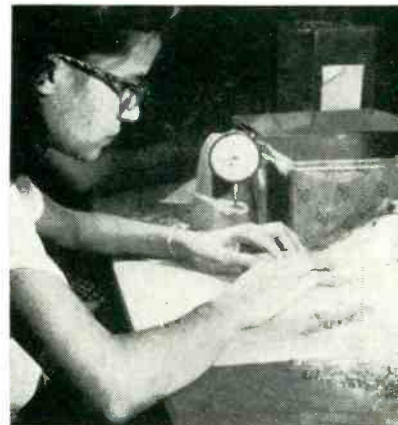
Frosted glass illuminated from below permits inspection for defects just as fast as operator can separate mica spacers with her nimble fingers
