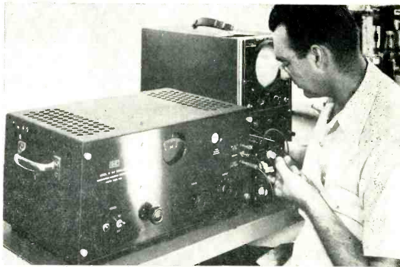
Test setup, with R-C oscillator at left. Frequency ranges are so chosen that readings of single 1-120 scale on tuning dial are multiplied by powers of 10
