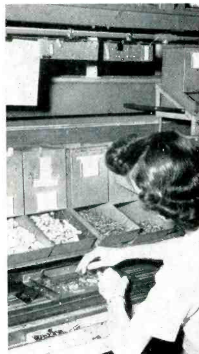
Inserting small parts in panel set into metal carrier on moving conveyor line. Sample panels hang from overhead wire. After all parts have been inserted, conveyor brings panel over pool of molten solder, and air cylinders bring up solder pot to solder all joints simultaneously
