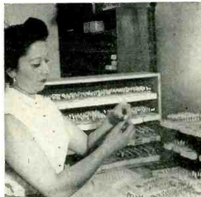
PLASTIC ENCASEMENT completes junction transistor manufacture. Junction is first dipped in polystyrene and then covered with black paint and Araldite
