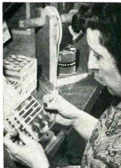
Applying masking tape to prevent sprayed molten metal from entirely covering ends of metallized paper capacitor units. Simple wood stand on bench, anchored by weight of solder spool, supports rolls of tape
