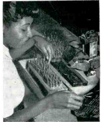
Motor-stirred varnish dispenser for applying protective coatings to resistors. Boards with drilled holes, raised above the bench by end blocks, serve as self-counting trays for uncoated resistors
