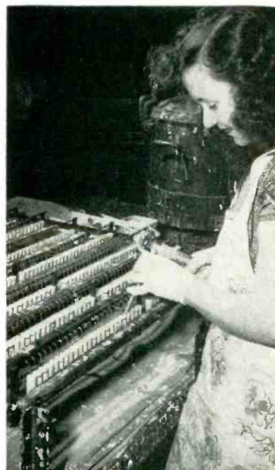
Squirting cement into ends of tubular paper capacitors with high-pressure cement gun. Racks are inverted for filling other ends of units
