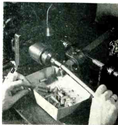
Improvised lathe for cutting metal tubing to size for capacitor housings. Pressure of cutting tool makes arbor rotate tubing which is loosely held by right hand of operator
