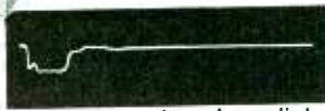
0.06 μ sec complex pulse applied directly to oscilloscope plates. Rise time approx. 0.001 μ sec.
