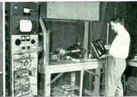
A physicist using a Rauland-developed radiation meter in checking X-ray radiations from cathode ray apparatus.
