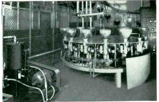
Kinney Vacuum Pump Case History #4 — The Rauland Corporation aluminizes television picture tubes on this high speed vacuum production machine.
