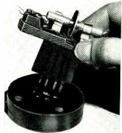
Pencil triode adapter using fuse clips for anode and cathode sleeve contacts
