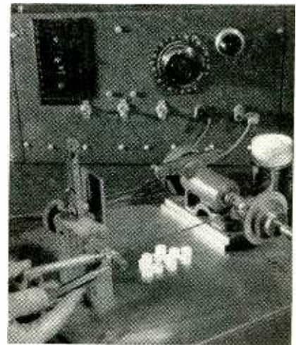
Setup for winding five-turn core of \frac{1}{4} -mil Orthonik on small ceramic spool. Test leads connected to welder in background are used to anchor last turn on core by spot welding. For small cores, winding mandrel is turned by hand with knurled knob at left. Motor drive is available for large cores. Welding points on vertical arm over winding fixture are used in place of test prods for welding larger cores
