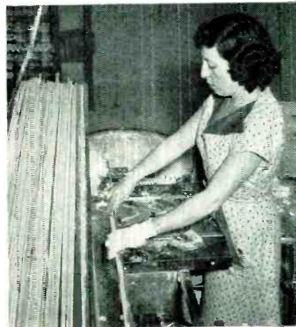
Prior to firing, tubular ceramic cores are being cut to exact size by Ann Trotta. A continuous check is made to maintain close dimensional tolerances.
