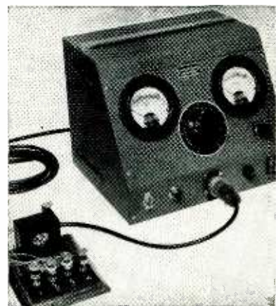
Miniature 400-cps motor is placed in fixture at left for quick check of performance
