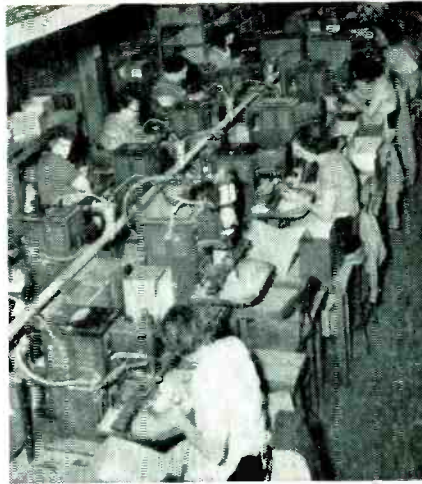
Skilled operators spot weld terminals to Vitrohm resistor ceramic cores. Welding assures permanent anchorage to the cores.
