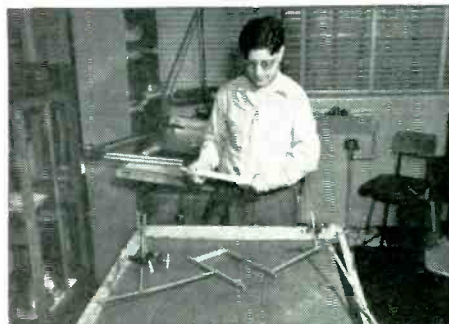
Rubber model for studying electron optical designing—basis for Rauland's exclusive Indicator Ion Trap.
