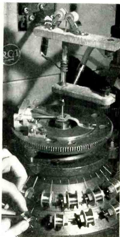
Machine for winding tiny grids used in pencil triodes
