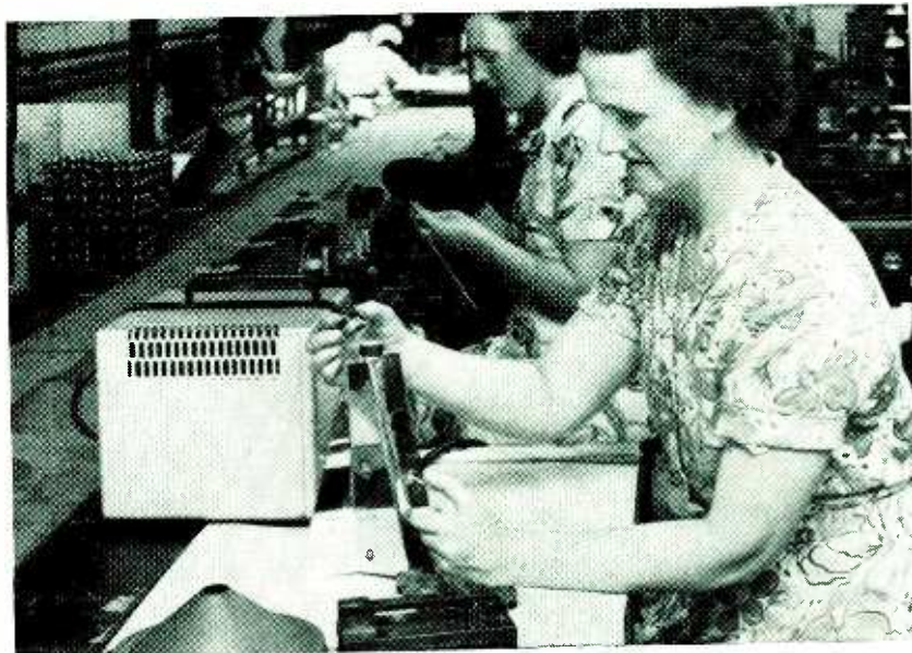
Production-line setup for tinning aluminum voice-coil leads for loudspeakers with ultrasonic tinning bath. Solder pot is at top, replacing pointed tip of soldering iron. Ultrasonic generator (about 20 kc) is in cabinet at left
