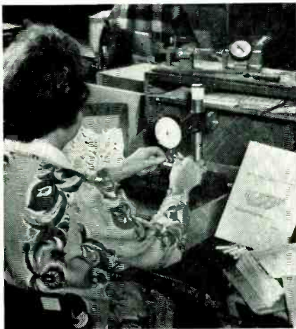
O.D. and concentricity of finished ceramic cores is checked by Minna M. Henderson, who has had 12 years experience with Ward Leonard.
