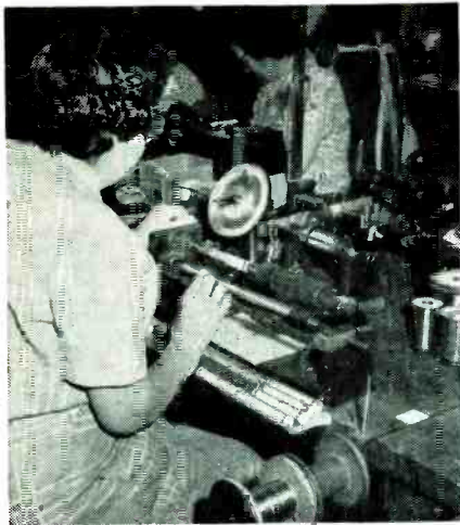
Special alloy resistance wire is being wound on Vitrohm cores by Caroline Jervisa, for 17 years an employee of the company.
