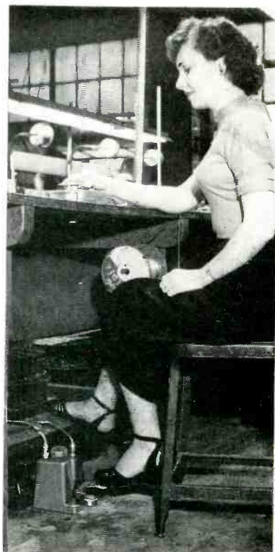
Method of using foot-operated air valve to actuate terminal twister
