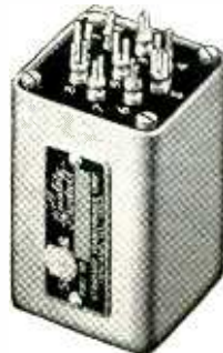
HIGH-FIDELITY INPUT TRANSFORMER, WF-20 , for low impedance microphone, pickup or line to grid. Primary impedance 50, 125/150, 200, 250, 333, 500/600 ohms. Secondary impedance 50,000 ohms. Frequency response 30-20,000 cps, \pm 2 db. Negligible harmonic and intermodulation distortion. Grey enamel cast case with phenolic terminal board and tapped holes for flush mounting. 2" high by 1\frac{1}{2} " square.
