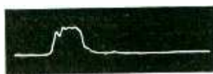
Pulse through Model 202P Wide Band Chain Amplifier and Model 214 Chain Pulse Amplifier (50 db gain). Note reproduction of fine detail.
