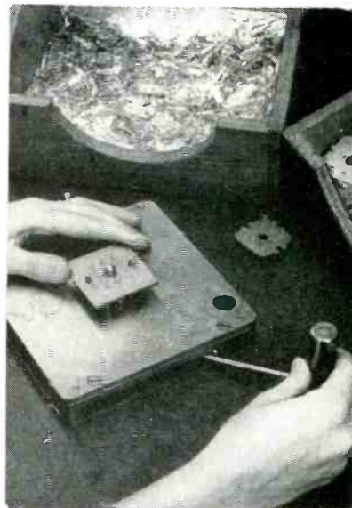
Manually-operated terminal twister. Parts bins used here are made from 1/2-inch plywood
