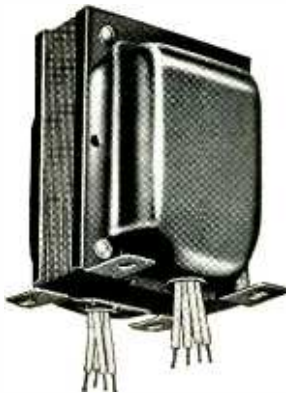
CATHODE RAY TUBE POWER TRANSFORMER, P-8151 , for use with type 2X2 rectifier tubes in a conventional half-wave high voltage supply. Plate supply 2,400 AC volts, half wave, 5.0 DCMA. Rectifier filament 2.5 volts at 2.0 amps. Other windings, 2.5 volts at 2.0 amps. Height 4\frac{3}{16} " , base area 3\frac{1}{16} " x 3\frac{7}{8} ".
