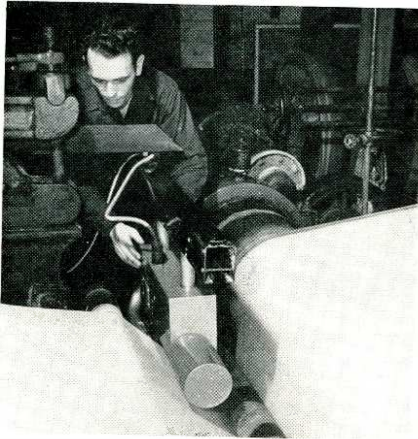
Thickness gage as installed in a paper mill. Paper passes through space between large chamber shown on top and smaller chamber partially visible beneath
