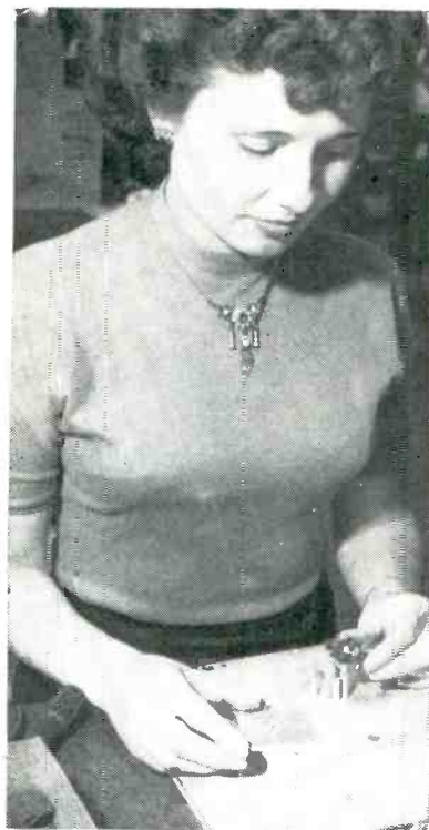
New air-operated fixture used in Crosley Division's Cincinnati plant to twist terminals of i-f transformer base after assembly
