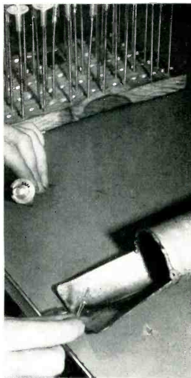
Holding heater assembly in air blast prior to insertion in cathode sleeve of type 5876 pencil triode. Air blast comes out of flattened copper tubing that is bent over edge of bench. Holes in board at rear are drilled in several diameters, so one board can be used for storing and transporting different sizes of assemblies
