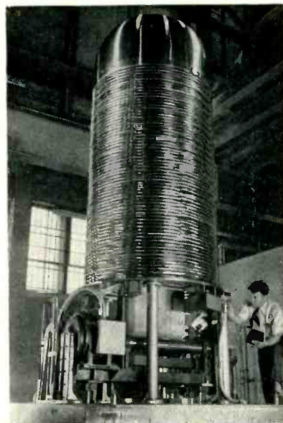
High-intensity 3,000,000-volt electron sterilizer with three charging belts and two acceleration tubes. Electron power is 12 kw
