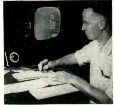
Industrial television enables this B&O yard clerk to record freight car numbers without walking among the cars and tracks. Unattended camera set up alongside the tracks does all the work as the trains pass in front of it
