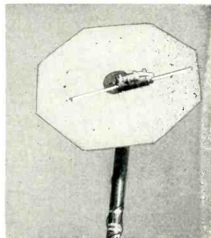
Turntable ground plane permits use of stationary measuring equipment
