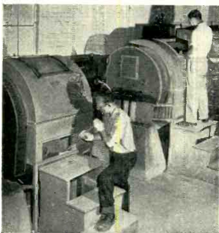
VITREOUS ENAMEL for coating is fritted, then ground to exact fineness in these revolving "ball mills."
