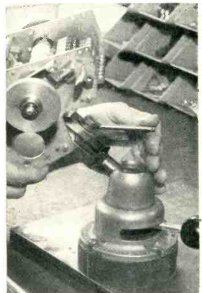
Vise-type holding fixture grips wide variety of subassemblies
