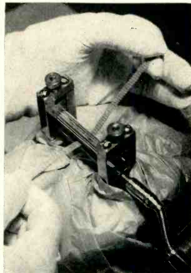
Gloved hands and paper under crimping machine insure cleanliness of crimped mesh ribbon
