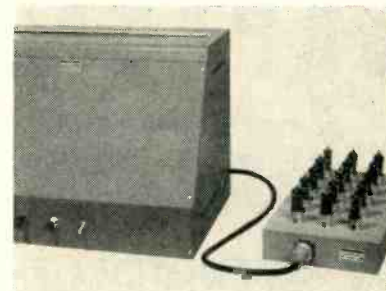
Burn-in setup for 15 type 6005 tubes
