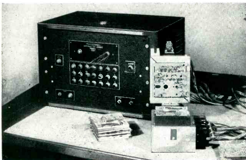
Finished cut-apart bases are checked in two seconds by a stepped test set that picks up leakage, shorts and opens
