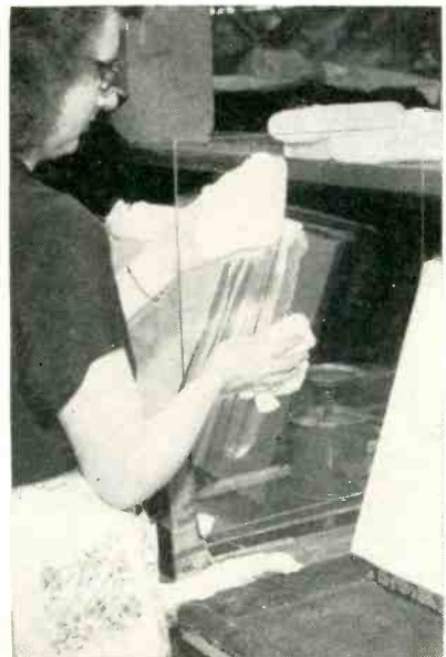
Window-cleaning rack. Safety dispenser for cleaning fluid can be seen on other side of glass
