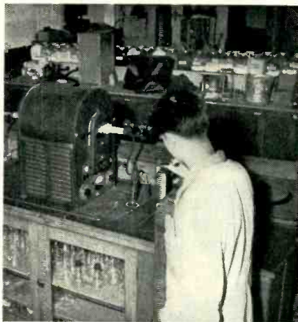
RESISTANCE WIRE sample is being processed in the combustion furnace to insure accuracy of alloy formula.
