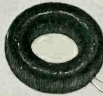
1-1/8" O.D. x 3/4" I.D. Wire—44 AWG Winding Speed—800 rpm
