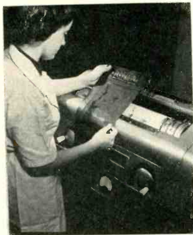
New photoelectric machine by Roneo Ltd., London, produces a ready-to-use stencil in a few minutes from almost any typewritten, drawn, printed or photographic copy. As a phototube scans the original line by line, an electric spark cuts a facsimile design spot by spot on the stencil
