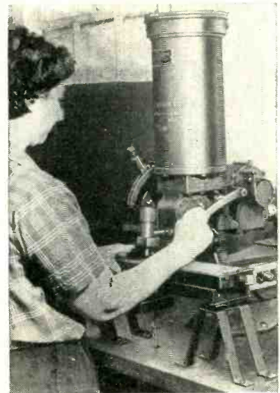
Method of using metering pump for filling large number of Vee-D-X television divider network molds one after another. Molds are held rigidly in metal frame having locking nut at one end
