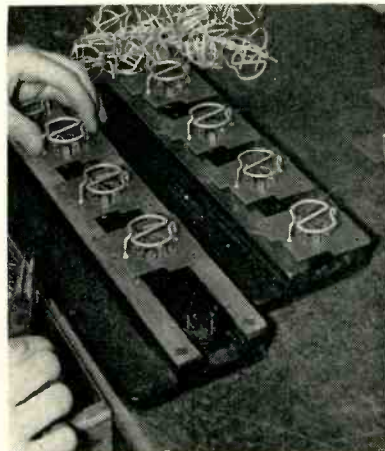
Socket subassemblies plug into up-ended tube bases on these holding fixtures
