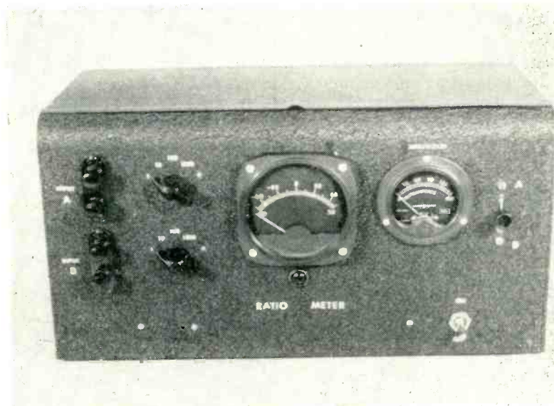
Front-panel view of the experimental model of the ratio meter. Meter indication may be calibrated in reflection coefficient or vswr
