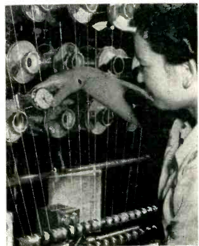
Saxl tension meter in use on coil winder in plant of New England Transformer Co.
