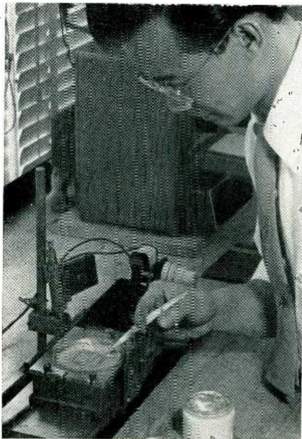
Applying silver mix to screen for producing terminal areas. Techniques for resistor mixes are identical
