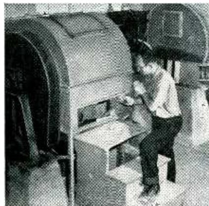
REVOLVING BALL MILLS grind the frit to the exact fineness needed to produce the perfect vitreous enamel used in the manufacture of the VITROHM rheostat.
