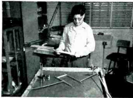
Rubber model for studying electron optical designing—basis for Rauland's exclusive Indicator Ion Trap.
