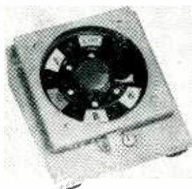
Bell System wire alerting network proposed for hospitals, factories and other large centers. Alerts and clear signals are sent from defense control point by special dial impulse to light appropriate indicator. Dial shown is under glass cover locked with key to prevent unauthorized tampering
