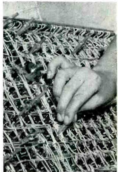
Alligator clips hold long leads in position temporarily until enough additional wires have been added to give effect of weaving that locks all wires in position
