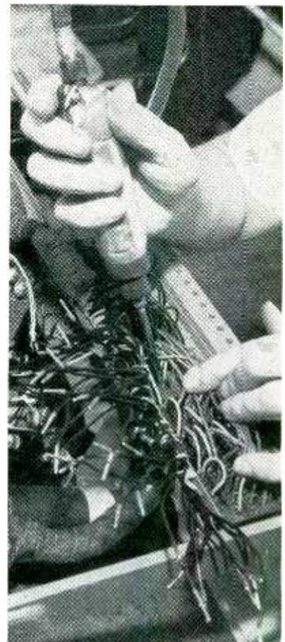
Using air-operated tool to push plug-tipped wires into tiny jacks
