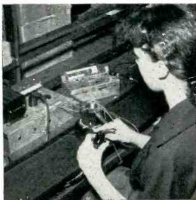
Plugging deflection yoke unit into test set socket, cable for which runs under metal pass-along trough on bench
