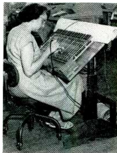
Use of inexpensive drafting table for assembly work
