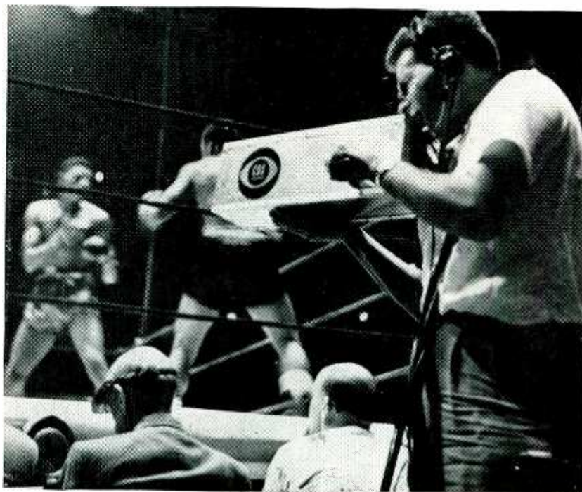
Designed for closeups during fight telecasts, this new portable tv camera developed by Robert Sammon of CBS contains only an image orthicon tube and controls. It is connected by cable to sweep and video circuits in a standard studio camera some 15 feet away. Equipped with a bullseye view finder, it weighs 22 pounds
