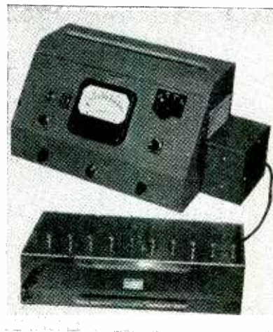
Capacitor tester; hinged box for ten capacitor units, in foreground, is connected to cut off high voltage automatically when cover is raised, to protect operator
