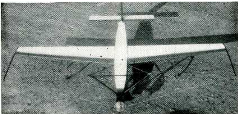
Two examples of firing error indicator installations. When used in 16-foot target glider, antenna wires run from plastic sphere back to outriggers on wing tips. Antennas for towing-sleeve installation are woven into cloth. In both uses, the receiving station is located in the tow plane, and error information is relayed on a command set to each fighter pilot in turn as he makes passes at the target
