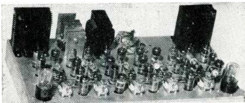
Electronic timer using binary counters. Input phototubes are at extreme ends of chassis
