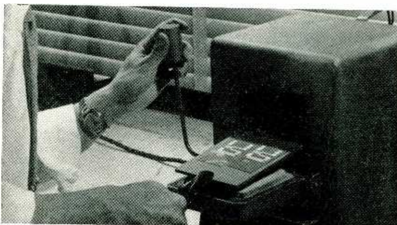
Placing coated glass plates in small furnace for curing of silver. Resistor printing with silk screen is next operation
