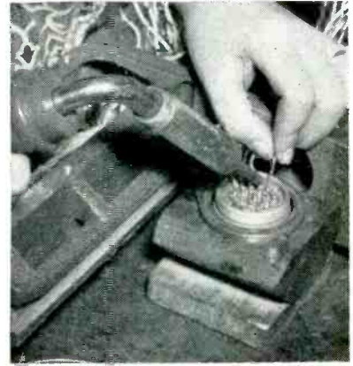
Method of soldering wire to cable connector without softening plastic insulation. Wood block serves as fixture for holding connector outside of transmitter housing during assembly
