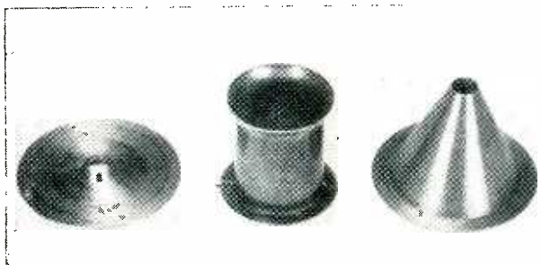
Later internal pole piece uses flat-plate front pole to reduce shielding of focus lens and allow shifting of field for centering
