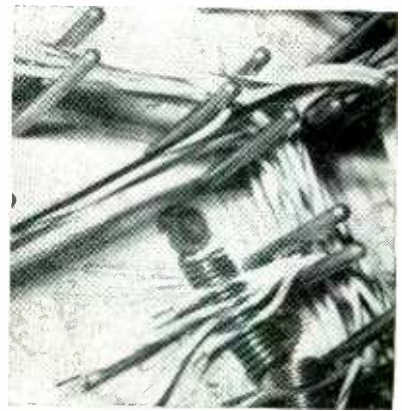
Use of springs to anchor ends of wires
