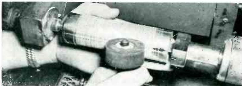
Creasing heater wire by running rubber roller over projecting insert in mandrel
