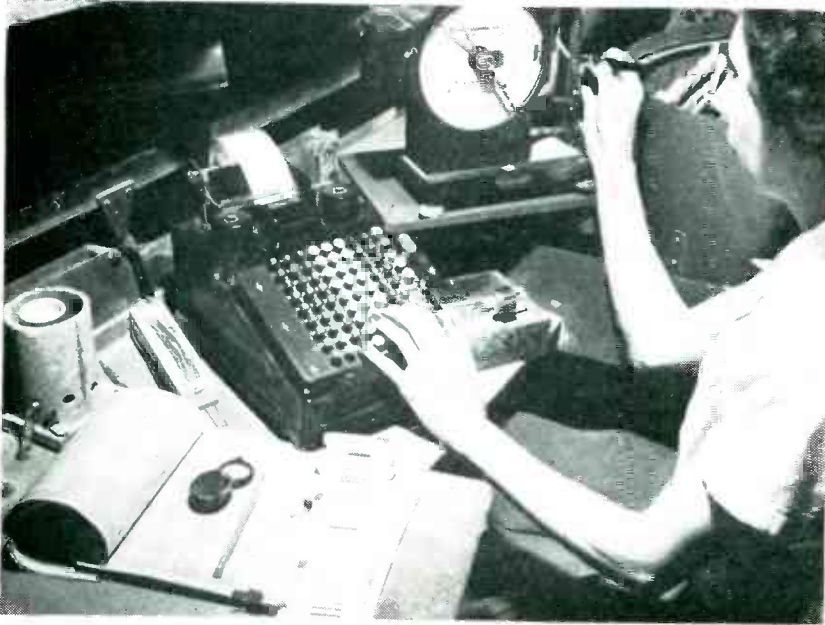
Using adding machine to get weight of oxide coating during sampling inspection of sprayed cathodes
