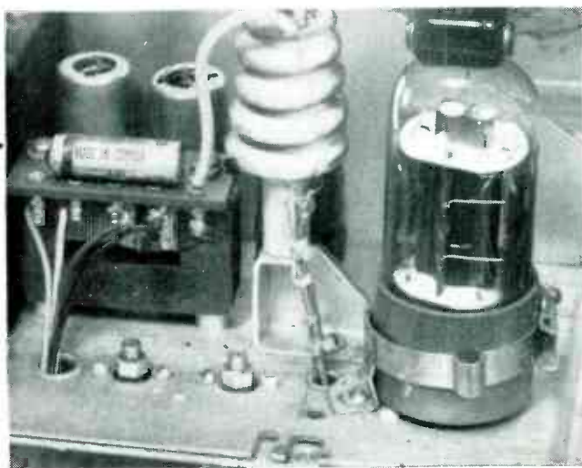
Photograph of marine 12-watt transmitter using saturable reactor tuning inductances shows ferrite core impedance step-down transformer (left). Ferrite core transmitter tank coil has Q of 200 at 3 mc
