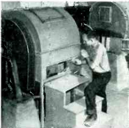
REVOLVING BALL MILLS grind the frit to the exact fineness needed to produce the perfect vitreous enamel used in the manufacture of the VITROHM rheostat.
