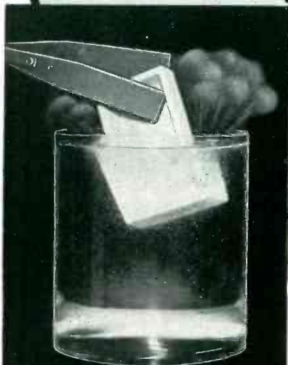
BOAT AT 2000° F. PLUNGED INTO ICE WATER DOES NOT CRACK
