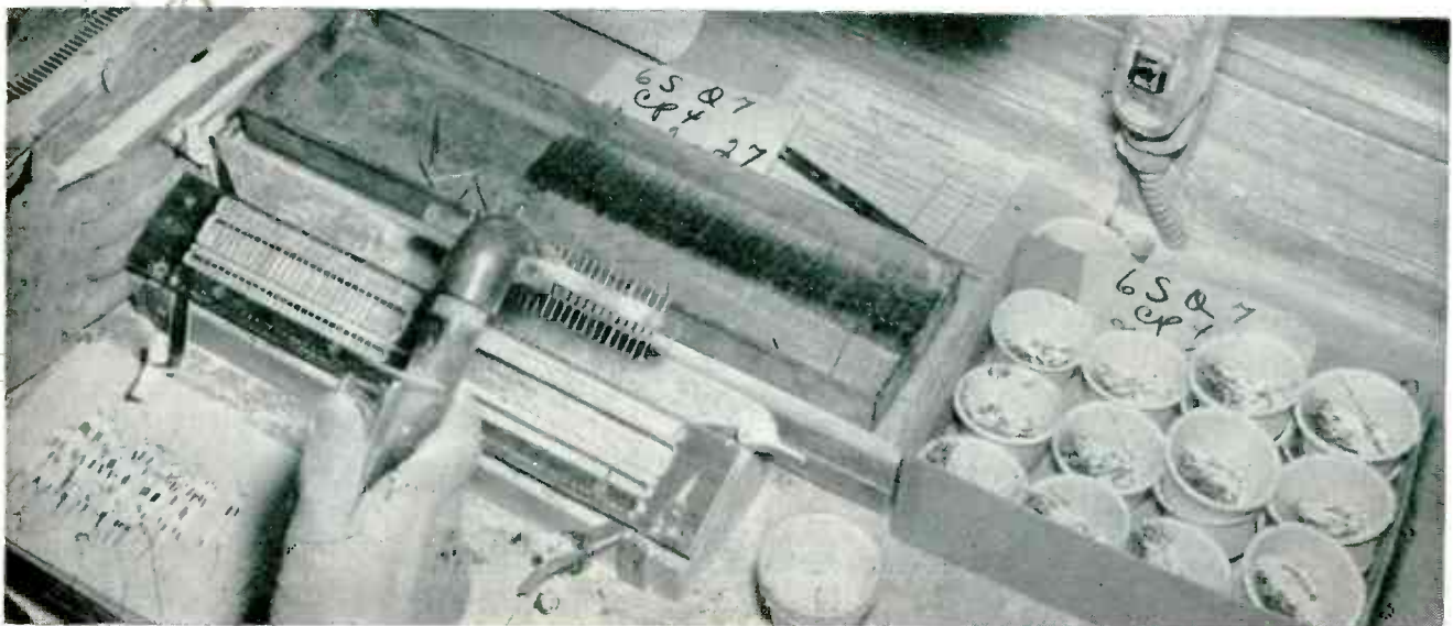
Transferring uncoated cathode sleeves from metal tray to spray rack with vacuum lifter. Unloading of sprayed racks is done here also, and finished cathodes are placed in paper cups, as at right. Cups can be reused about ten times before replacement
