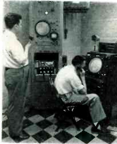
Improvement brought about by new CAA-developed radar presentation system is vividly illustrated by photograph showing the old (right) and the new (left)
