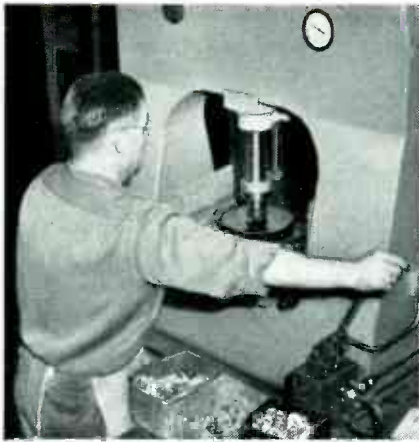
ERICK SCHNEIDER, a company employee for over 23 years, operates a hydraulic press for securing the bushing assembly to the rheostat base plate.
