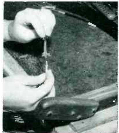
Inserting metal sleeve between flared-out shield and dielectric of coax
