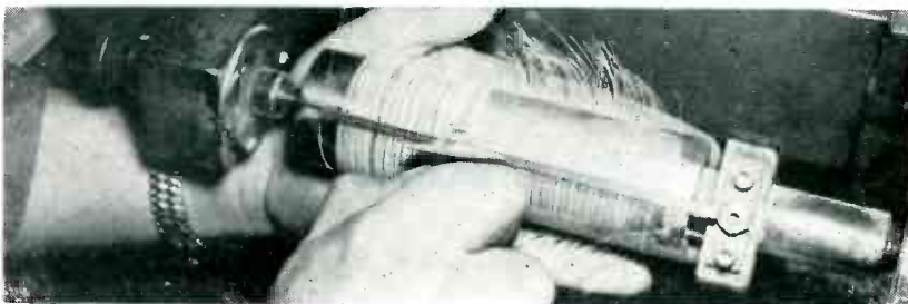
Cutting heaters apart by running steel disk in slot of cutoff anvil
