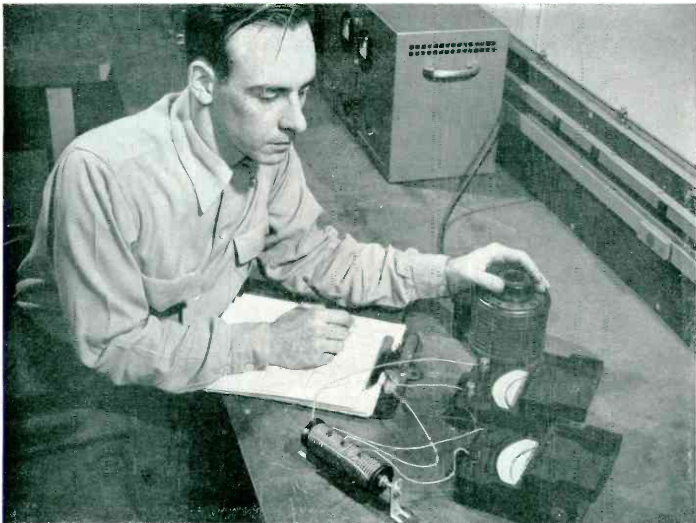
THE TEST FOR FORWARD VOLTAGE DROP OF RECTIFIER REQUIRES ONLY VARIABLE A-C SUPPLY, A-C VOLTMETER AND D-C AMMETER
