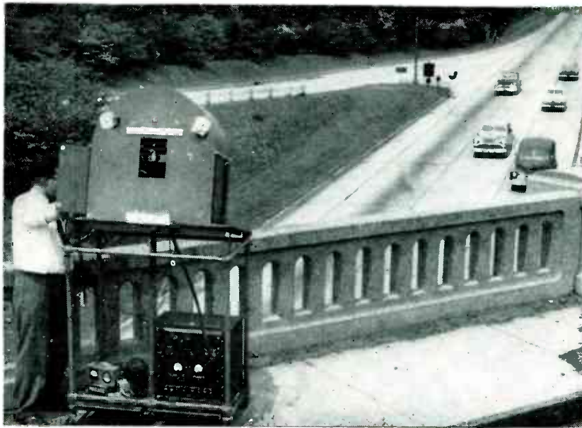
Radar-controlled camera overlooking New Jersey's busy Route 4 photographs license plate of any New York-bound car doing 55 mph or more
