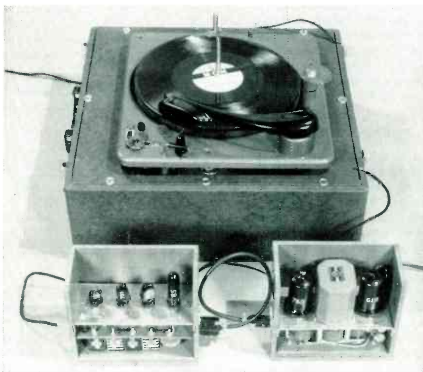
Phonograph amplifier using single-ended class-A amplifier chassis on left and push-pull class-A amplifier on right
