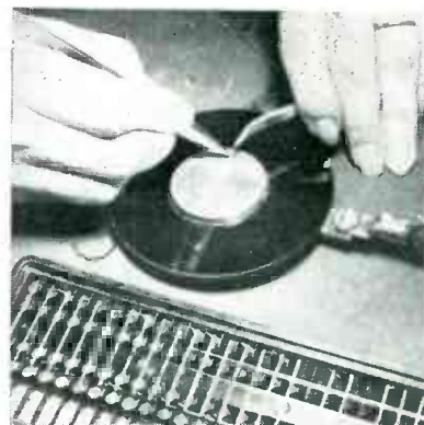
Setup for welding extremely small tabs to coiled heaters of tubes
