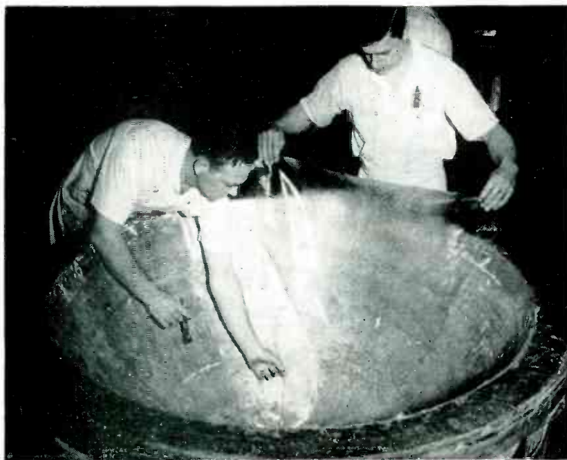
Lay-up of impregnated cloth. The brush is used to aid in smoothing out the cloth and removing air bubbles
