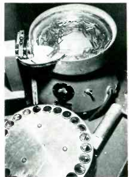
Two rubber rollers driven by small electric motor can be seen at left of bowl feed. Cathodes drop into glass cups on table actuated by air cylinder at lower right
