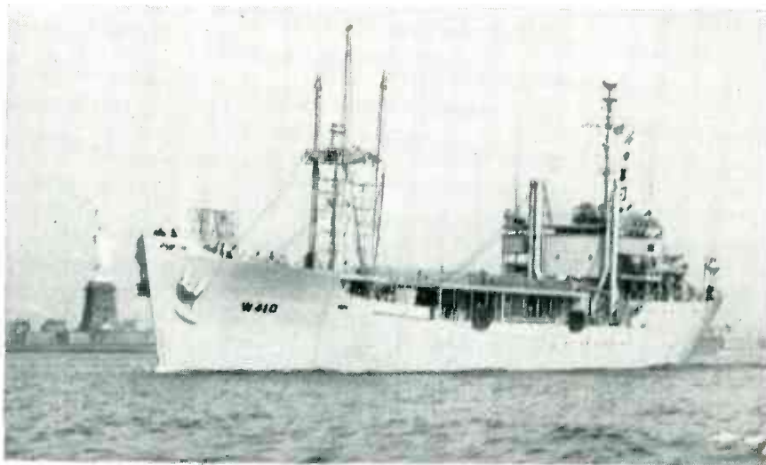
Coast Guard cutter "Courier" assigned to Project Vagabond can broadcast on short waves from inverted pyramid antennas forward. Receiving whips are aft
