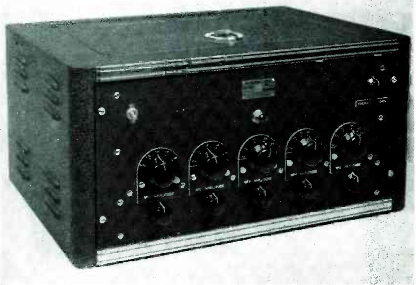
Ten knobs across front of generator control frequency and amplitude of gated signals. Knob in upper right-hand corner sets overall gain
