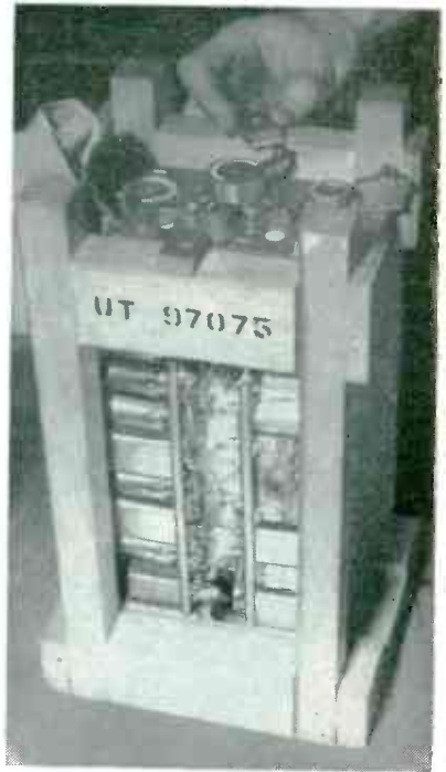
Wood blocks on top of protective wood frame are turned to lock chassis in position. Open sides give access to parts
