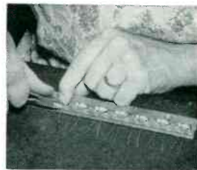
Cutting leads precisely to length, using edge of holding fixture as guide
