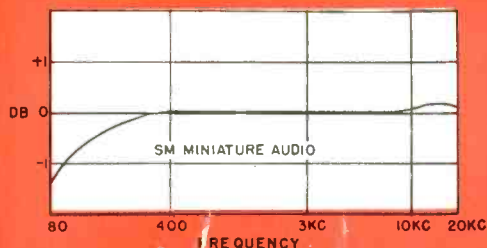
SM sub-miniature audio components, \frac{7}{16} " x \frac{1}{2} " x \frac{7}{16} " height. Weight — .009 lbs.
