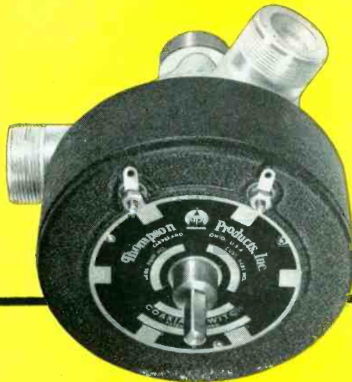
Model CA-36, 1P3T manually-actuated RG-17/U Coaxial Switch with electrical and mechanical interlock.
