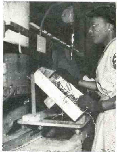
Three-purpose chassis cart for television receiver assembly line
