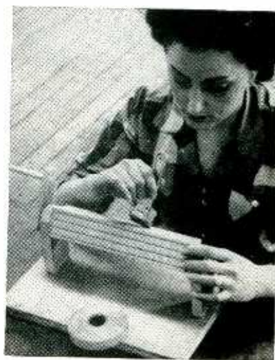
Wood fixture used at Utility Electronics for cutting tape into tabs
