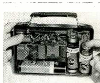
Rear view of the new RCA personal portable, showing the new alkaline B battery at the left
