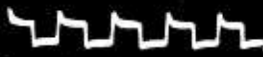
Forward resistance of a bad diode under dynamic conditions showing excessive overshoot.
