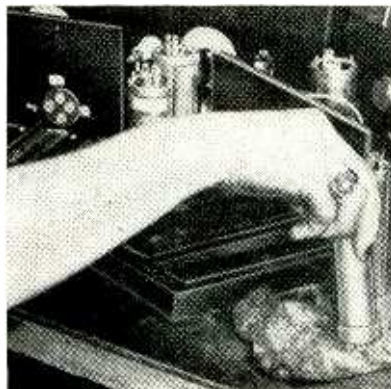
Discharging electrolytic capacitor in steel wool after leakage test
