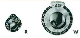
MODELS R AND W DUODIALS Each model available in standard turns-ratios of 10, 15, 25 and 40 to 1. Inner scale indicates angular position of HELIPOT sliding contact, and outer scale the helical turn on which it is located. Can be driven from knob or shaft end. R—2" diameter, exclusive of index. W—4-3/4" diameter, exclusive of index. Features finger hole in knob to speed rotation.
