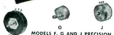
MODELS F, G AND J PRECISION SINGLE-TURN POTENTIOMETERS Feature both continuous and limited mechanical rotation, with maximum effective electrical rotation. Versatility of designs permit a wide variety of special features. F—3-5/16" dia., 5 watts, electrical rotation 359°—resistances 10 to 100,000 ohms. G—1-5/16" dia., 2 watts, electrical rotation 356°—resistances 5 to 20,000 ohms. J—2" dia., 5 watts, electrical rotation 357°—resistances 50 to 50,000 ohms.
