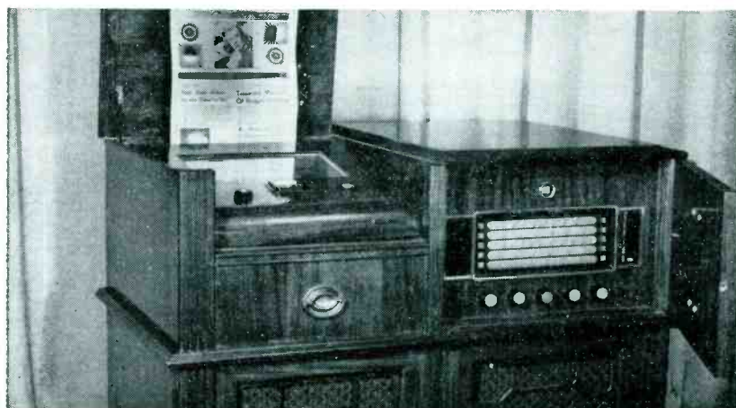
General Electric type 417A radio receiver used in the type FR-1 combination for sound and facsimile
