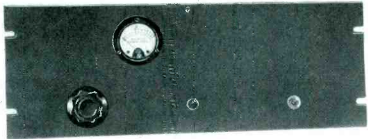
Panel of complete delay limiter showing single control. Linear compression scale is obtained by using expanded meter scale
