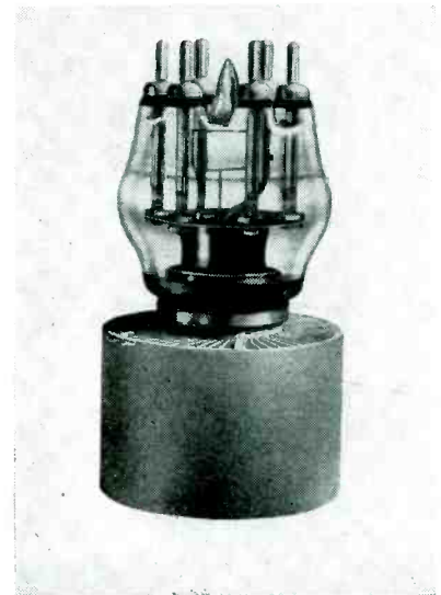
One of the oscillator tubes used in a 5-kw 450-cycle r-f induction heating generator
