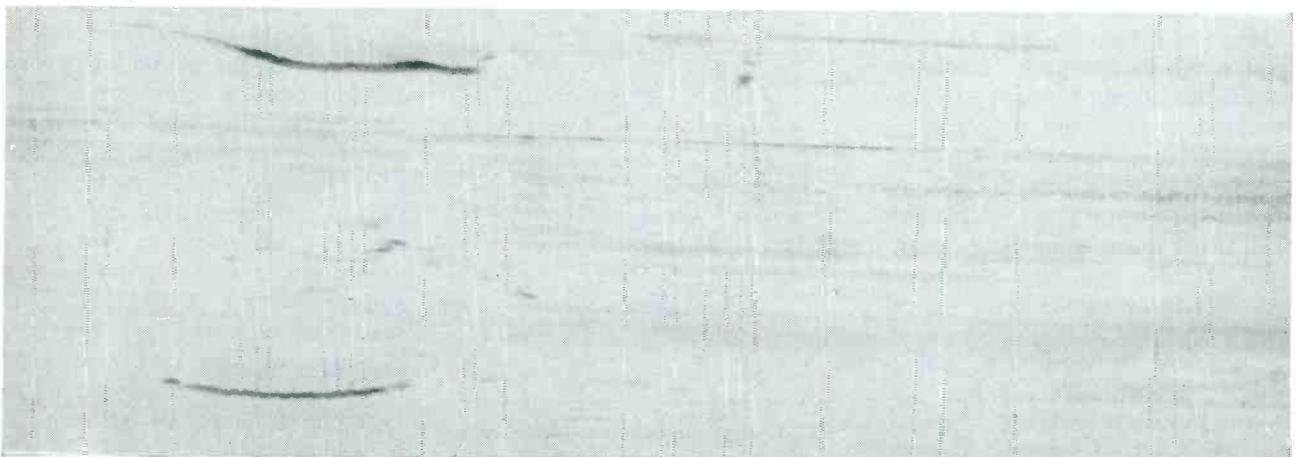
Example of record obtained, showing cracks in a two-foot length of gun barrel
