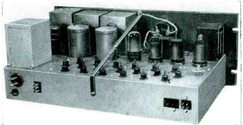
Chassis layout of complete delay limiter. Delay line coils can be seen projecting through the chassis
