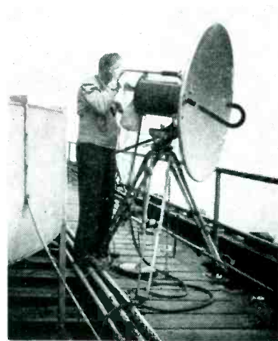
FIG. 8—Microwave receiver antenna. Note the use of a telescope sighted through four-foot parabolic reflector and sand bag for balance while tracking
