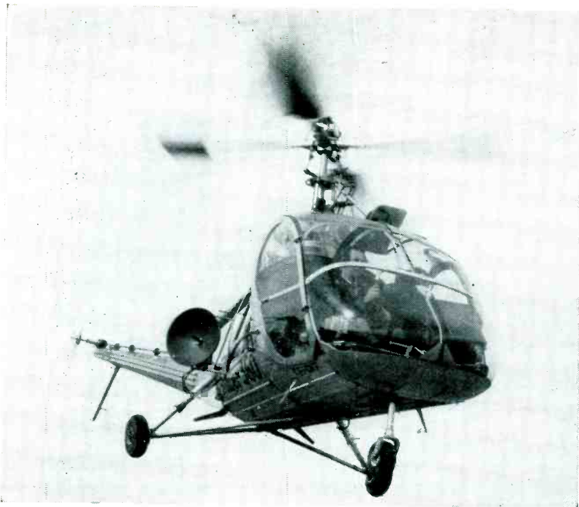
Airborne helicopter, showing location of receiving parabola on side. A similar antenna on the other side of the plane permits 360-degree azimuth coverage
