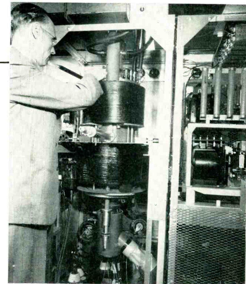
Adjustments are made by the author to the 5-kw klystron mounted in the cubicle of a developmental transmitter. The tube cooling system requires six gallons per minute of water and approximately 200 cu ft of air, practically at atmospheric pressure
