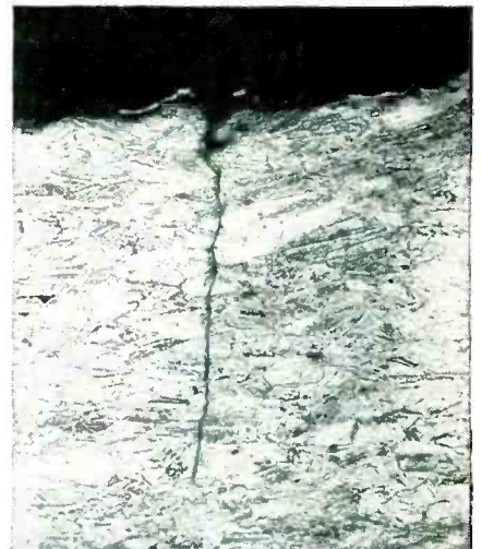
Micrograph illustrates cracking of stressed tubing after testing with ammonia, moisture and air.
