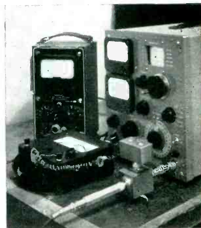
FIG. 2—Micropotentiometer is shown in set-up for calibrating millivoltmeter
