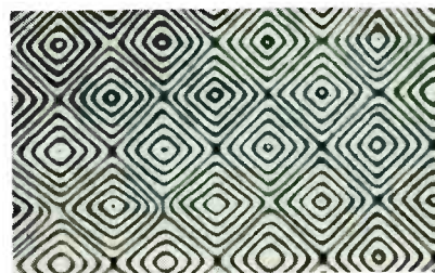
FIG. 11—Square-net domain pattern of single barium titanate crystal, visible because crystal is transparent
