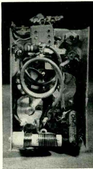
Closeup of underside of exciter chassis shows close fitting of components required. Authors advise a 12AU7 provides greater output than the 7F8
