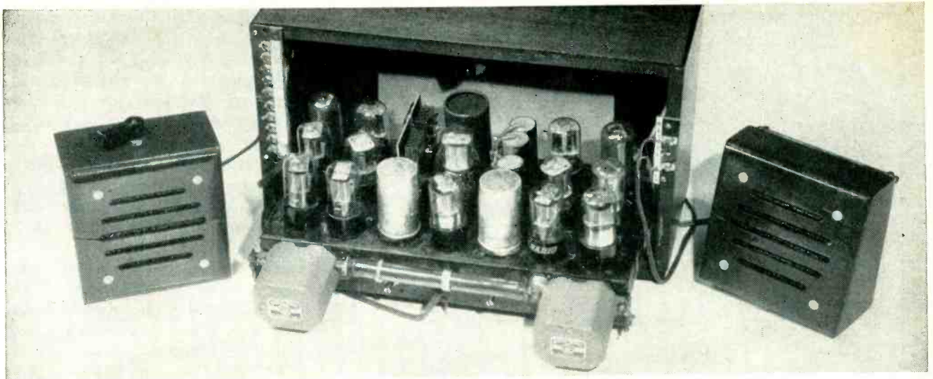
Complete automatically switched intercommunicator. Remote stations contain only speaker and annunciator pushbutton for signaling master station to originate a call. Pushbutton switches are used to insert 14-tube voice-switched master unit between desired calling and called stations
