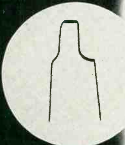
Horizontal sync-pulse as displayed on WO-57A screen
