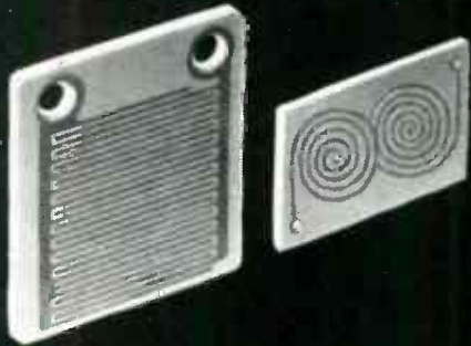
10 Examples of special "printed circuit" parts. Left — a fixed value capacitor. Right — an inductance coil.
