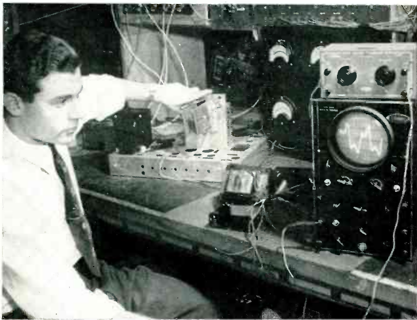
FIG. 17—Chassis fixture for measuring stray magnetic field of power transformers at neck position of picture tube as part of power transformer acceptance test
