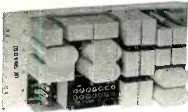
Line Terminal and composite panel W.E. Co. X-61823C for terminating composited open wire and cable circuits using 1000 cycle signaling.
