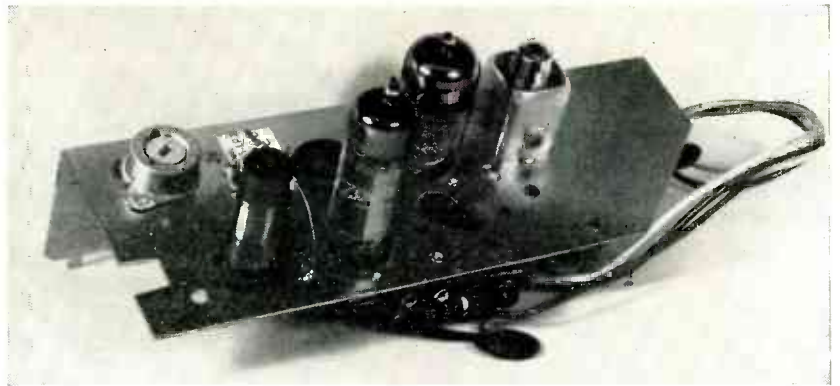
Subassembly chassis of the sound channel having the simplified circuit arrangement
