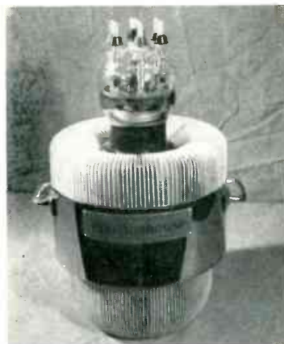
This 25,000-watt Westinghouse radio transmitting tube with a laboratory-built aluminum radiator weighs 98 pounds, which is 56 percent less than conventional 225-pound copper-radiator tubes
