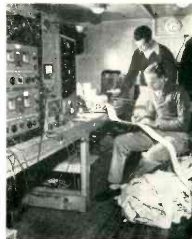
Continuous-wave meteor recording apparatus permits study of swarms of meteors too small for photographic recording
