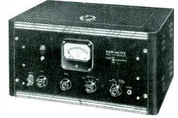
Newly developed direct-reading instrument simplifies measurements of wow and flutter in speed of phonograph turntables, wire recorders, motion picture projectors and similar recording or reproducing mechanisms. It is the only meter in existence giving direct steady indication of meter pointer on scale.
