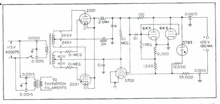
FIG. 1—Example of miniature thyratron regulated power supply circuit used with potted subassemblies to decrease size, weight and heating. Thorough shielding is necessary to avoid radiated noise from thyratrons. All 0.0015-µf capacitors are ceramic feed-through units to prevent conducted noise
