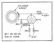
FIG. 2-Circuit of the cylinder oscillator
