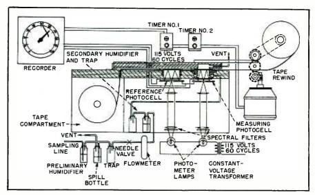
FIG. 1—Schematic diagram of hydrogen sulfide analyzer. The sensitized fabric tape passes through one chamber unchanged but turns brown in the one at right
