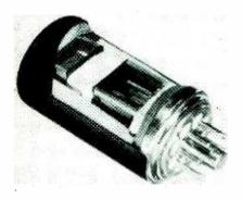
It can be used to convert small d-c values to a-c, and can then rectify the amplified signal to produce d-c again whose polarity and level vary directly as the source.
