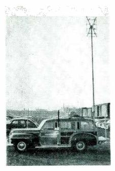
Photograph of the mobile receiving station used. The 8-element array is shown in place 23 feet above ground
