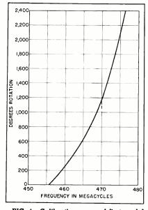
FIG. 4—Calibration curve of first model constructed
