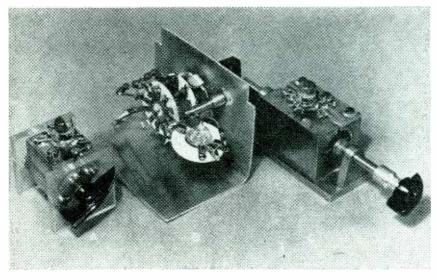
FIG. 1—A semi-butterfly oscillator is shown at A, a tap-switch oscillator at B and a cylinder oscillator at C
