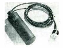
810 counts per minute from 5 micrograms of radium filtered through  $\frac{1}{2}$  in. of lead 12 inches from the end; has a maximum recovery time of 800 microseconds; a maximum dead time of 100 microseconds; is suitable for an input circuit impedance of 5 megohms; and has an ambient temperature rating of +40 to -70 C.
