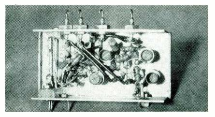
FIG. 9—Bottom view of 205-mc i-f amplifier. Chassis is approximately 2 inches wide and 4¾ inches long
