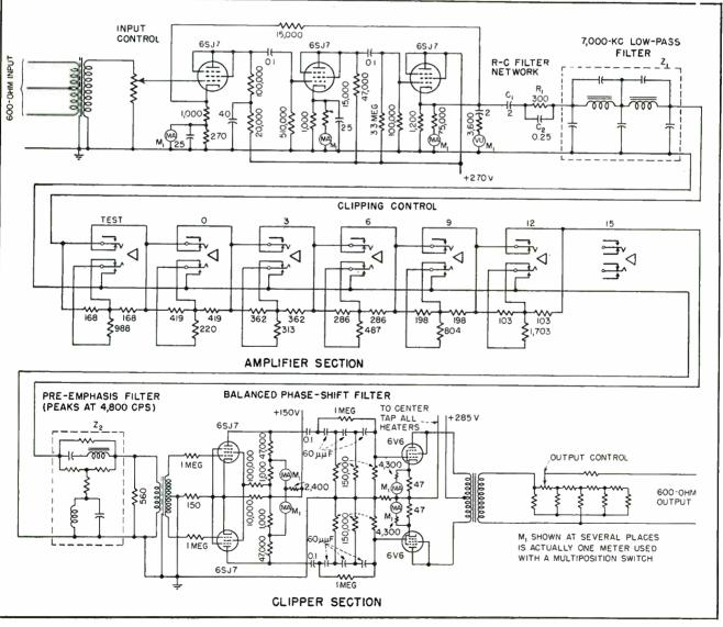
FIG. 1—Schematic circuit diagram of the audio peak clipping amplifier
