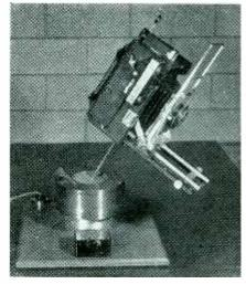
Demonstration of use of magnetic fluid as universal positioning device for heavy camera. Fluid in nonferrous metal cup solidifies around camera support rod when coil surrounding cup is energized with d-c. Current is interrupted with switch in foreground whenever camera needs repositioning
