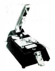
recording tape without scraping, cementing, use of adhesives or loss of tape material. A plastic weld is obtained by a combination of electrically produced heat and precise pressure applied within an accurately controlled time cycle. The equipment is self-timing, operates on 115-v 50 or 60-cycle a-c, with automatic line-voltage compensation. Each splice takes from 4 to 5 seconds with 5 seconds required after splice to permit tape to cool off.
