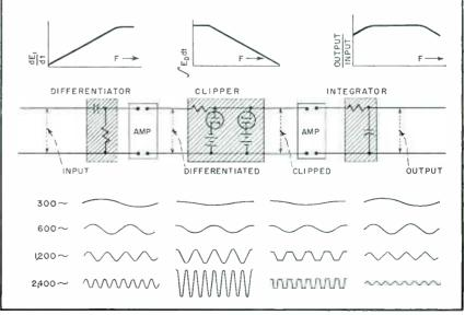
FIG. 1-Basic circuits illustrating the fundamental principle
