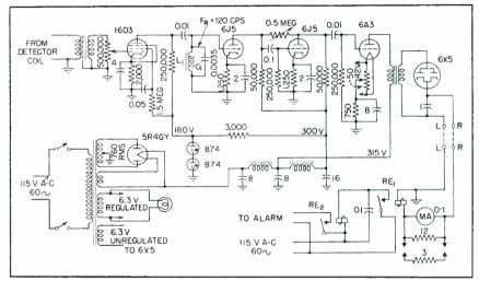
FIG. 4-Schematic diagram of metal detector amplifier and null detector
