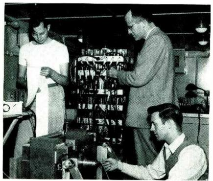
The equipment above, installed in a trailer, was recently taken by University of California scientists to a mountain top in the high Sierra for investigation of the behavior of cosmic rays under controlled conditions. It counts and identifies negative and positive mesotrons in the cosmic radiation. Cloud chambers in another trailer were used to measure momentum and mass of particles
