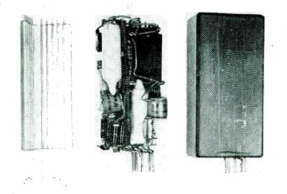
Steps in potting a three-tube strain gage amplifier. Left—casting-resin chassis with imbedded silver-clad beryllium-copper wires serving as stiffeners, tie points, plug prongs and lead wires. Center—assembled chassis with built-in limiter and voltag gain of 20,000, adjusted in production so all units have same gain within 1 percent. Right—complete plug-in unit as potted in casting resin. Other examples of potted plug-in units are shown in color on the front cover of this issue
