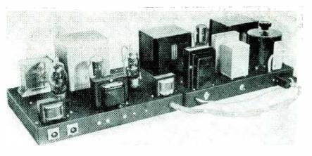
Since space conservation is of no importance at lumber mills, no crowding of components was felt necessary, as may be seen from the above photograph of the metal detector oscillator chassis and power supply
