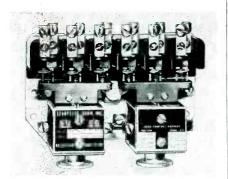
175KXX contactor comprises two 3-pole solenoids for forward and reverse operation mounted on a common frame and mechanically interlocked to prevent simultaneous closure. Designed particularly for service in the control of single horsepower motors, the use of the contactor is completely described in bulletin 7100.
