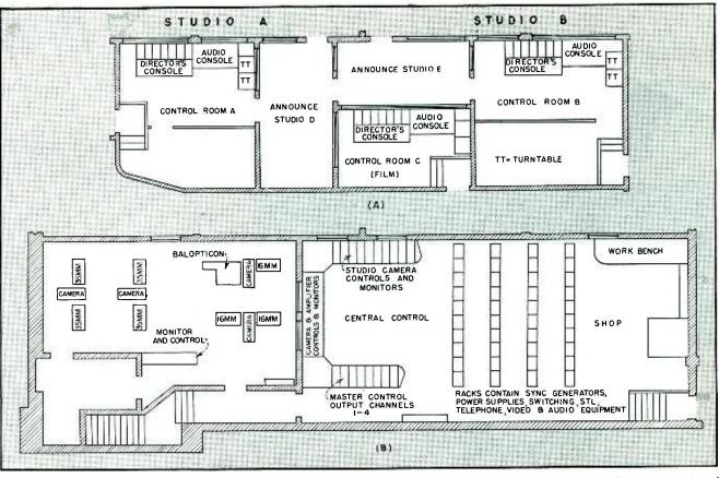
FIG. 9—Control areas in the studios. Program control rooms (A) are located at approximately studio floor level. Camera control and equipment (B) are located on floor above looking out over studios
