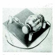
Photograph of a vacuum capacitor voltage divider. The values of the capacitors shown are 5 and 500  $\mu\mu f$  with 17,500-volt ratings—Official Photograph U. S. Navy
