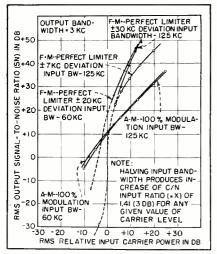
Comparison of theoretical a-m and f-m range performance with decrease of input bandwidth and different frequency deviations
