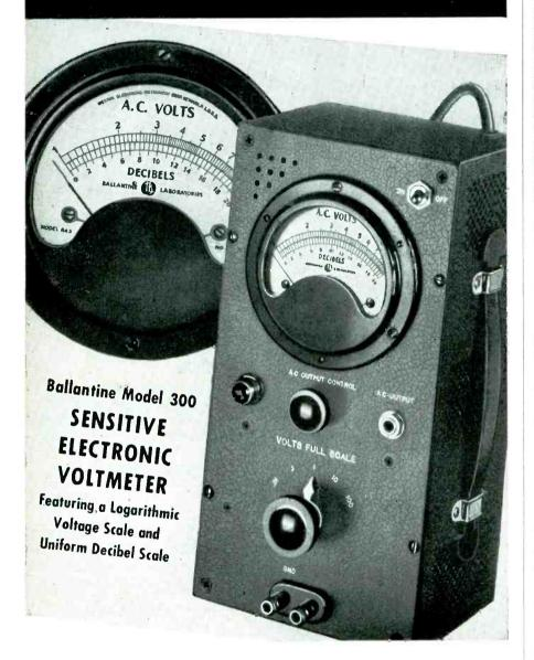
Designed for the measurement of AC Voltages from .001 Volt to 100 Volts over a frequency range of 10 to 150,000 cycles. ● Accuracy of readings is ±2% at any point on the scale. ● Very stable calibration—unaffected by changes in line voltage, tubes or circuit constants.
