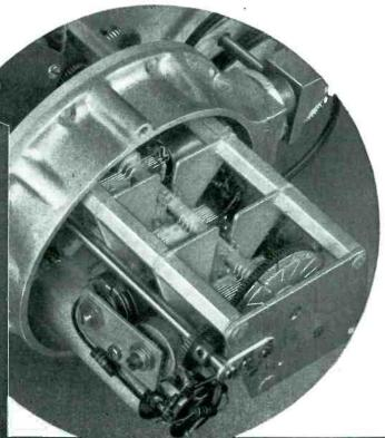
Shown above is an interior view of the 202-B Signal Generator RF assembly with shield cover removed. Heavy aluminum castings form the mounting base of this RF unit resulting in a compact and highly rigid structure. Girder type condenser frame construction, multiple rotor shaft grounding contacts, and welded interstage shield plates are but a few of the many design features of this unit which give added circuit stability.
