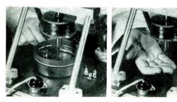
Test setup for demonstrating solidification of magnetic fluid by a steady magnetic field. With coll deenergized at left, fluid flows into pan under pipe. When direct current is sent through coil, flow is cut off instantly and even fluid in air below pipe has hardened
