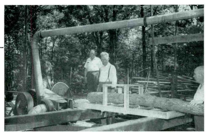
The photograph shows a typical metal detector setup with the coils mounted to inspect the logs on their way to the saw
