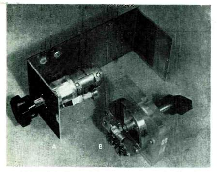
FIG. 4—A rolled-up line mixer is shown at A and a semi-butterfly mixer at B
