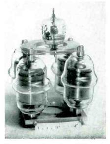
Vacuum capacitor voltage divider using tube plate-to-filament capacitance in series with four 50- $\mu\mu$ f vacuum capacitors connected in parallel-Official Photograph U. S. Navy
