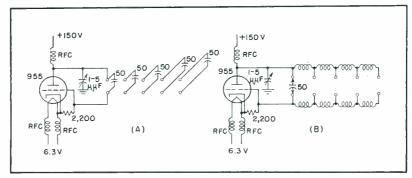
FIG. 3-Tap-switch oscillator circuits similar to that shown in Fig. 1B
