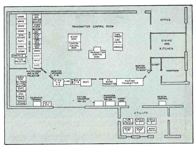
FIG. 4-Layout of equipment and facilities in the transmitter building
