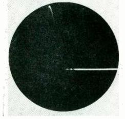
At low operating voltages the cathode-ray tube will respond to a high-speed transient signal, but—only at high voltages is the light output sufficient to SEE and RECORD it.
