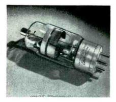
and inverse is 1,500 v; peak cathode current, 40 amp; average cathode current, 3.2 amp; current averaging time, 15 seconds; ambient temperature range, minus 55 to plus 70 C.
