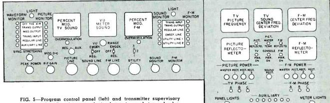
FIG. 5—Program control panel (left) and transmitter supervisory control right. Complete console is shown in a photograph elsewhere in these pages
