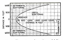
FIG. 3—Plan view of receiver vicinity showing areas of useful and detrimental scattering
