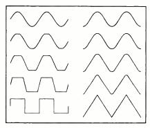
FIG. 2—Sine waves with various degrees of clipping, before and after integrating
