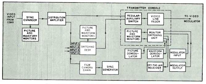
FIG. 8—Video signal switching and check points at the transmitter plant
