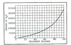
FIG. 3-Basic calibration of the analyzer
