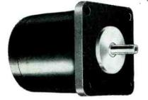
TELETORQUE UNITS: precision synchros for transmitting angular movements to remote points. Accurate within ±1°, May be actuated by mechanisms that produce only 4 gm. cm. (.056 oz. in.) of torque.
