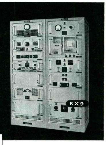
Type DS9 Single Sideband Radio Transmitter Frequency Range 4-22 Mc/s. Power Output 300 watts. Two independent sidebands with reduced carrier. Total sideband width adequate for 3 telephone channels, many teleprinter channels or various combinations of telephone and teleprinter. Sideband generating equipment built into transmitter. Compact design and rugged construction with maximum accessibility from the front only.
