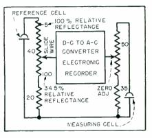
FIG. 4-Slide-wire photometer bridge circult
