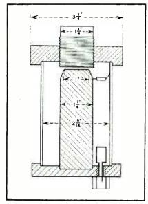
FIG. 2—Mechanical drawing of first model of cavity wavemeter
