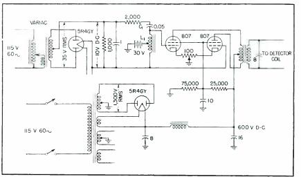
FIG. 3—Schematic diagram of 120-cps oscillator used to drive pickup coils
