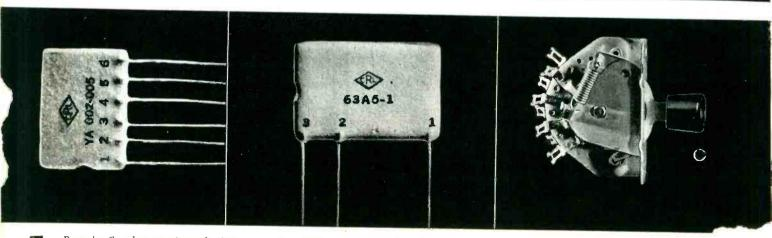
Pentode Couplate consists of plate lead and grid resistors, plate by-pass and coupling capacitors. Minimum soldered connections speed production.
