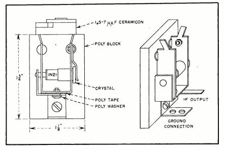
FIG. 7-Simple fixed-tuned mixer for 530 mc
