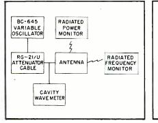
FIG. 3—Block diagram of setup for calibration and schematic circuit of cables to wavemeter
