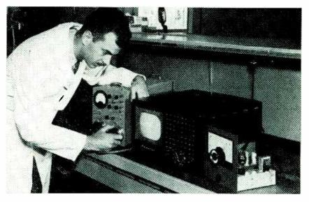
Fixed-tuned converter being tested in conjunction with a standard television receiver. Vernier tuning of the local oscillator is provided
