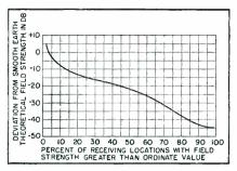
FIG. 6—Curve showing the relationship between the percent of receiving locations and the measured field intensity in db below theoretical for smooth earth
