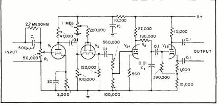
FIG. 3—Fixed station instantaneous deviation control circuit
