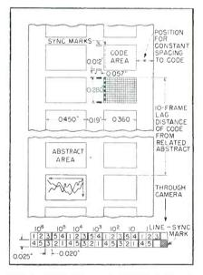
FIG. 1—Arrangement of abstract and code areas on master film, and method of assigning code numbers to squares to accommodate 10,000,000 different subjects
