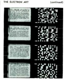
Sample of coded master 35-mm film. Wide dashes in middle are for frame sync, and first vertical row of squares to the right is for line sync to identify the horizontal rows to be paired in searching for a blackout. Each pair of rows is a subject code number, hence six pairs permit coding each abstract under up to six different subject headings
