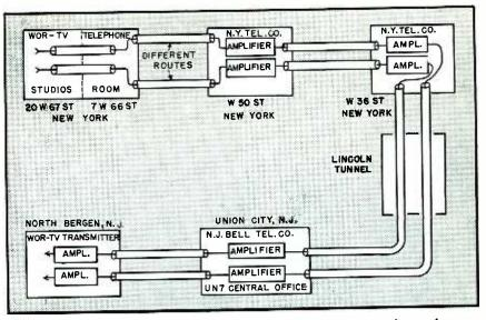
FIG. 6—Simplified diagram of the coaxial cable circuits between studios and transmitter
