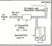
be expected (1.000018). Since the fundamental resonant wavelength is proportional to the physical length of the cavity (unloaded), the resonant frequency will lower 0.0018 percent per degree rise in temperature.
