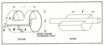
FIG. 6—Mechanical details of the rolled-up line
