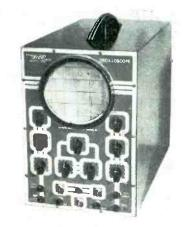
it has a horizontal sweep circuit of 15 to 30,000 cps. Frequency response of horizontal and vertical amplifiers is 50 cycles to 50 kc. It has an input impedance of 1 megohm and 50  $\mu\mu$ f, and a deflection sensitivity of 0.30 volt per inch full gain.
