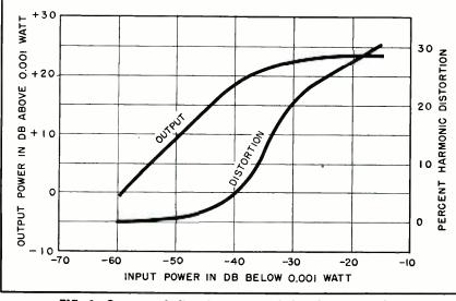
FIG. 3-Output and distortion curves of the clipping amplifier
