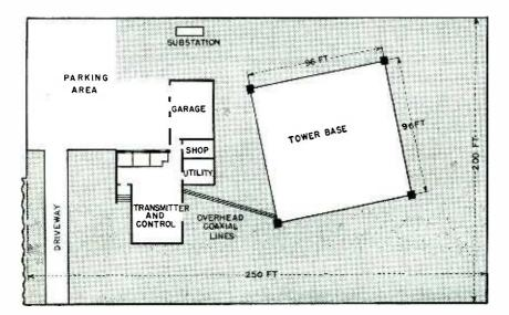
FIG. 2—Ground plan of the North Bergen property showing relation of the tower, transmitter building and power substation
