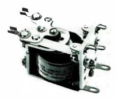
ture and stationary contact assemblies. Coil data: a-c coils, consuming approximately 4 volt-amperes, available up to 220 volts; d-c coils, consuming 1 to 2 watts, available up to 110 volts. Overall dimensions are  $15/16 \times 1\frac{7}{8} \times 1\frac{9}{16}$  inches.
