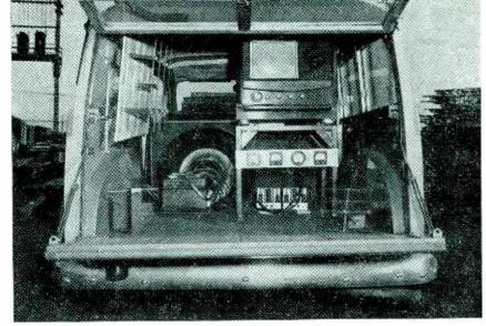
Interior view of the mobile setup used in the Washington field strength measurements. The four meters mounted below the receiver read 450-mc local oscillator injection current and plate current, the receiver afc voltage and the field strength
