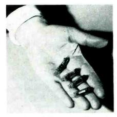
at 1.25 v and 40 ma d-c. Plate voltage ranges from 30 to 67.5 volts, and plate currents, from 0.30 ma to 2.0 ma.
