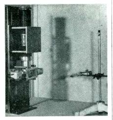
Experimental arrangement used at National Bureau of Standards to expose a nylon thimble chamber to x-rays from a beryllium-window x-ray tube mounted behind a solenoid shutter control which admits definite amounts of radiation to the thimble ionization chamber
