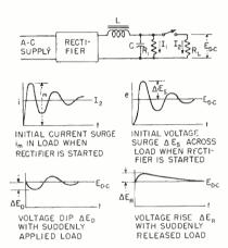
FIG. 1—Basic choke-input filter circuit, and curves illustrating four transient conditions affecting circuit design
