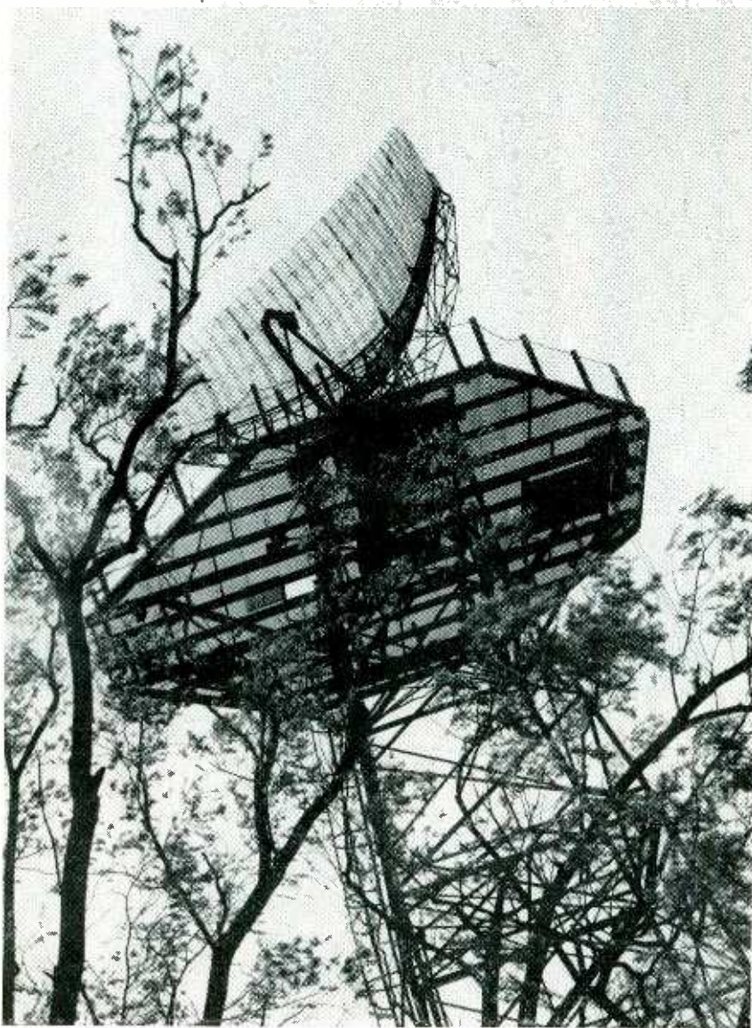
Antenna of CPS-5 search radar, weighing one ton and rotating at 10 rpm. At Berlin it was mounted on a 25-foot steel tower atop a five-story building
