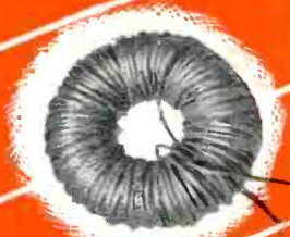
C This sub-miniature (.18 cubic inch) output transformer is intended for hearing aid and other extreme compact service. While the dimensions are only 7/16" x 9/16" x 3/4", the fidelity is ample for voice frequency requirements.
