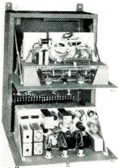
Photograph of Ship's Call Alarm in servicing position. Bottom shelf contains the crystal-controlled receiver
