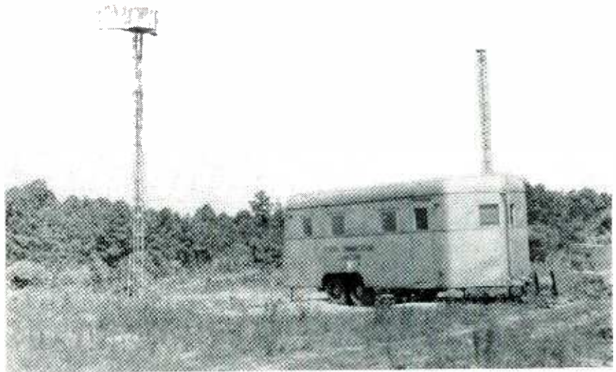
FCC measurement station at Laurel, Md., with 700-mc parabola on tower at left. The 47.1 and 106.5-mc dipoles are stretched between towers
