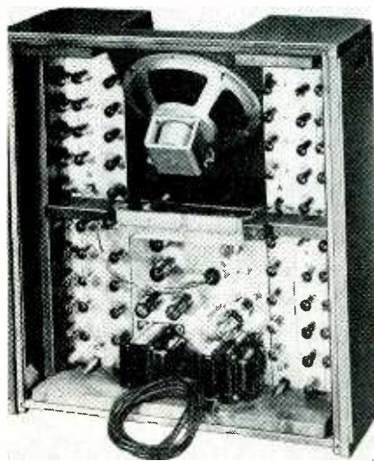
Tone generators and audio amplifier of the Organo are connected to the control elements on the piano by a multiwire cable
