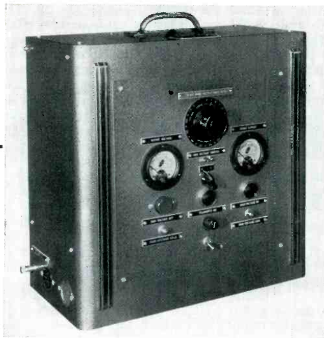
Front view of 30-kv portable power supply. Control panel may be removed and cabled to power supply for remote operation
