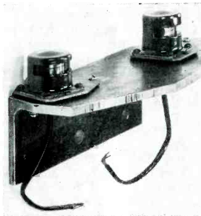
Individual mounting bracket for pair of recording heads that act simultaneously on two sides of a single tape to produce two tracks
