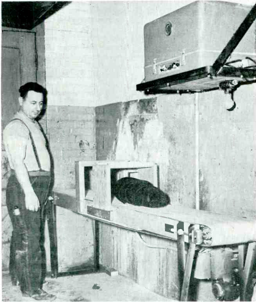
Operator runs bolt of rubber through metal detector coil, shown over conveyor belt housed in wood baffle for protection. Metal detector unit may be seen on shelf at upper right corner of picture
