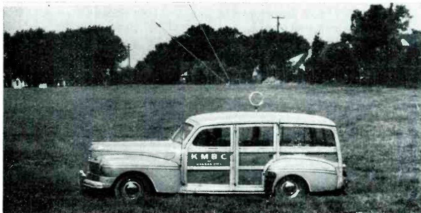
Typical field-measurement car showing loop antenna on roof
