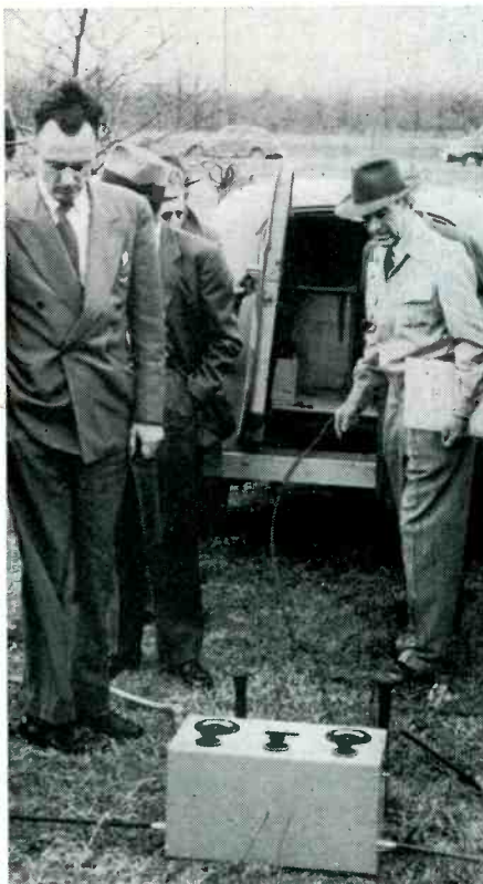
W. M. Barret (right) explains operation of his radio system for geophysical prospecting during demonstration at Grand Saline, Texas. Note insulated antenna wires running along ground in opposite directions from transmitter
