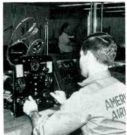
Test setup for checking operation of cabin pressurization instruments and gages
