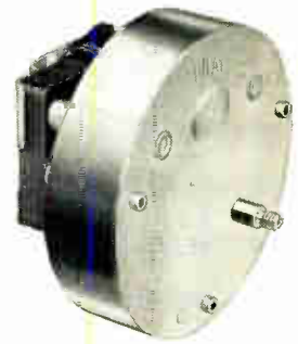
Type 1M9 instrument movement. Designed especially for chart drives but adaptable to most instruments. Terminal shaft speeds from one revolution in 15 minutes to 1 in 30 days. Terminal shaft rotation counterclockwise.
