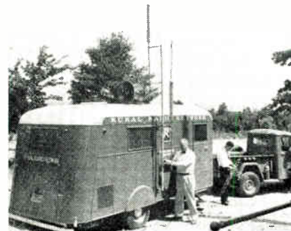
Engineers adjust antennas of Nemo trailer used by Rural Radio Network for remote pickups. The program is broadcast from here on 152.75 mc to the nearest RRN station
