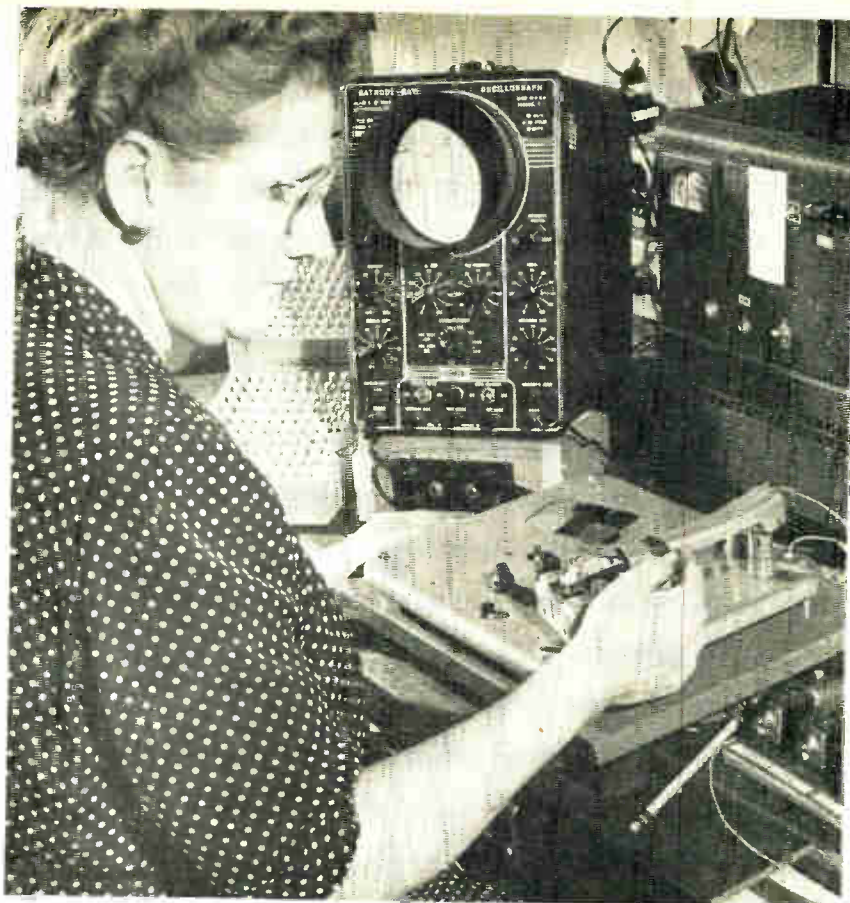
To test each cartridge, it is placed on a vibrating platform which is driven in frequency across the audio spectrum. Oscilloscope and meter show pickup response
