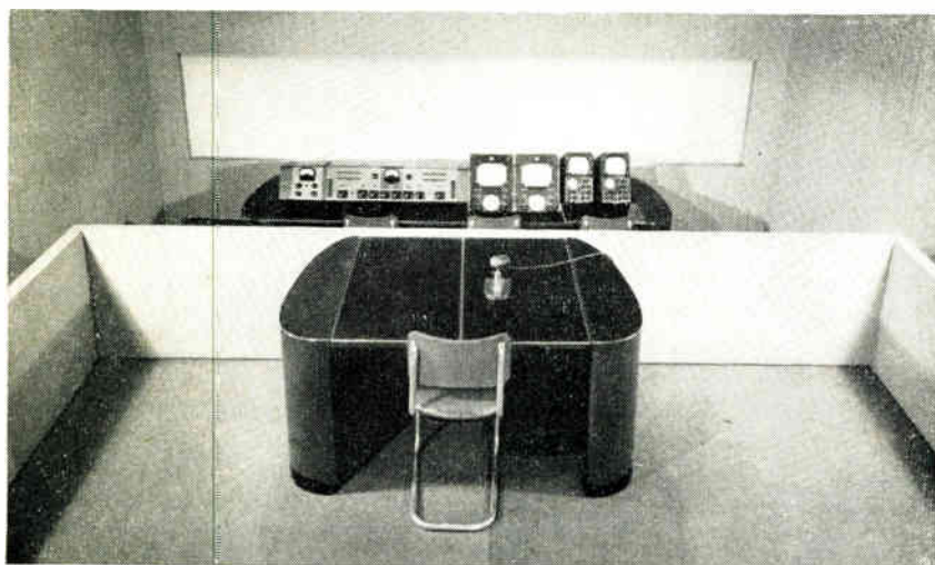
Typical small-studio control room with audio controls at left, video at right. The program director sits at the desk
