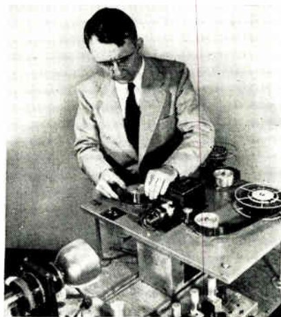
Donald S. Bond, RCA Laboratories, Ultrafax project engineer threads film to be transmitted between the flying-spot scanner (left) and the photomultiplier tube (in light box beneath his left hand)
