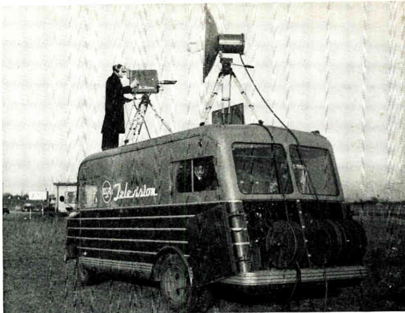
Mobile field unit that can double as initial control room for the small station. One camera and 7,000-mc relay equipment are mounted on the roof
