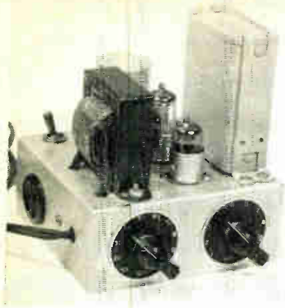
Complete timer chassis. The relay is mounted underneath
