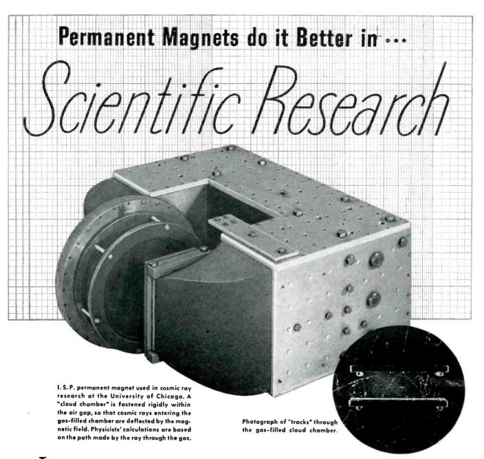
In Cosmic Ray research at the University of Chicago, an I. S. P. permanent magnet helps speed the study of particles unbelievably small—yet with energy that staggers the imagination. U. of C. physicists asked our engineers to furnish this special permanent magnet—with a 6.5 inch air gap—to make their studies possible at high altitudes.
