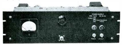
Continuously Adjustable and Regulated 600—1500 V.D.C at 0-1 Milliampere.
