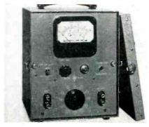
meter model 404A is designed for a-c measurements from 2 cycles to 20 kilocycles at voltages ranging from 0.001 to 300 volts. Input impedance is 10 megohms shunted by capacitance of approximately 20 picofarads.
