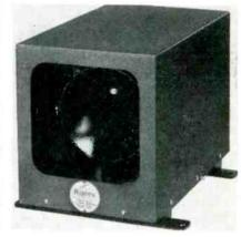
any change in frequency or reduction of light intensity sounds the alarm. Lens mountings have micrometer adjustments to facilitate focusing on the phototube. The unit is weather-tight and rust-proof.
