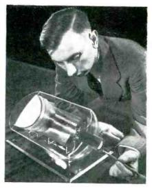
Cutaway view of the image amplifier tube. Its principle of operation is reminiscent of the Snooperscope and Sniperscope used for infrared viewing during the war
