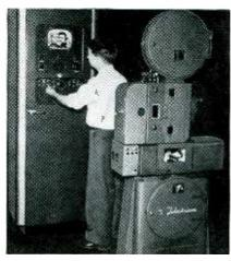
drive mechanism make it possible to project 35-mm pictures directly on to the pickup tube of a television film camera for conversion to video signals. Monitor and change-over control are housed in a standard cabinet rack.
