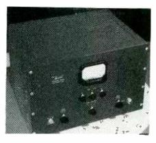
milliwatts down to a few microwatts. The unit requires 115 volts, 60 cycles for operation. Weight is 45 pounds. Descriptive literature is available.
