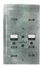
put voltage is continuously adjustable over a range of less than 600 to more than 1,500 volts by the operation of a control knob on the front panel. The unit is built for low-current devices such as Geiger tubes.
