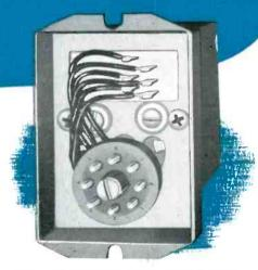
View of base assembly of dust-tight relay mounting showing terminals brought through Neoprene gasket. Note radio-type plug and flanges for securing to chassis.
