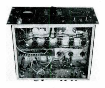
Bottom view of 64 scaler, showing simplicity of wiring. Arrows point to sockets of plug-in units
