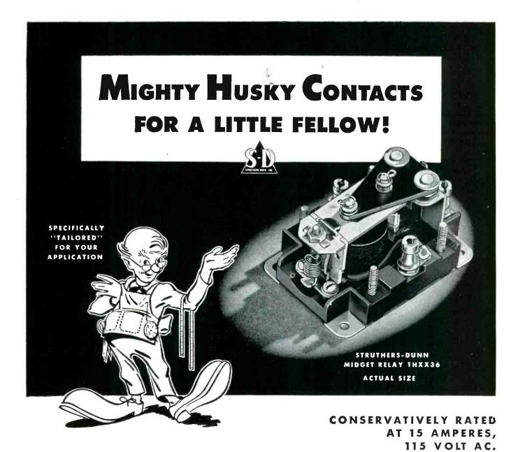
This little relay, only 1% x 2% x 2% is made for trouble-free performance on a long list of heavy-duty control applications. Single-pole, single-throw, double-break 3% diameter fine silver contacts. Underwriters approved.
