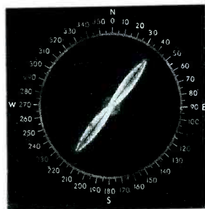
FIG. 3—In this typical indicator pattern, propeller tips serve as pointers to indicate bearing. This pattern has 180-degree ambiguity, necessitating auxiliary means for determining sense
