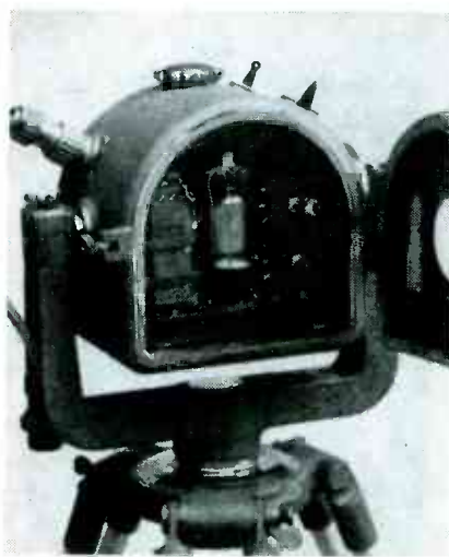
Light and sound pickup is mounted on an antivibration chassis
