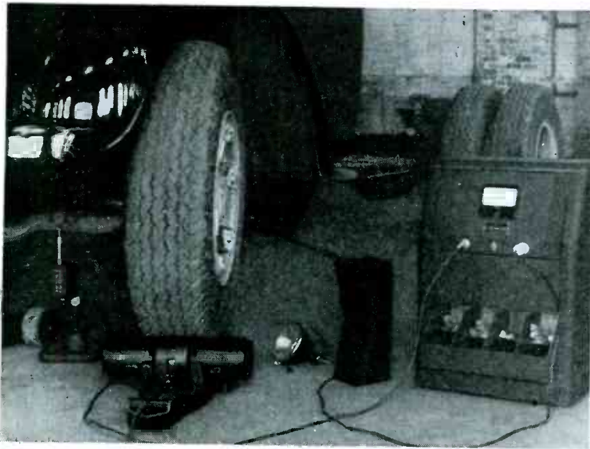
Vibration pickup, wheel spinner, stroboscope lamp and electronic amplifier unit of the truck wheel balancer
