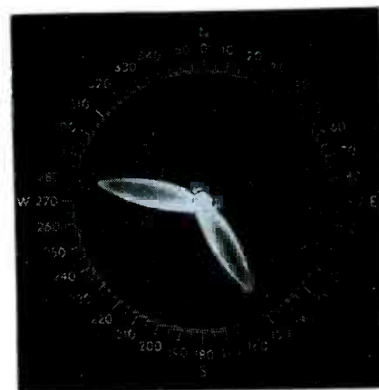
FIG. 4—Throwing a sense switch folds back propeller tips form arrowhead pointing in true direction of signal. This sense pattern resolves the ambiguity of Fig. 3
