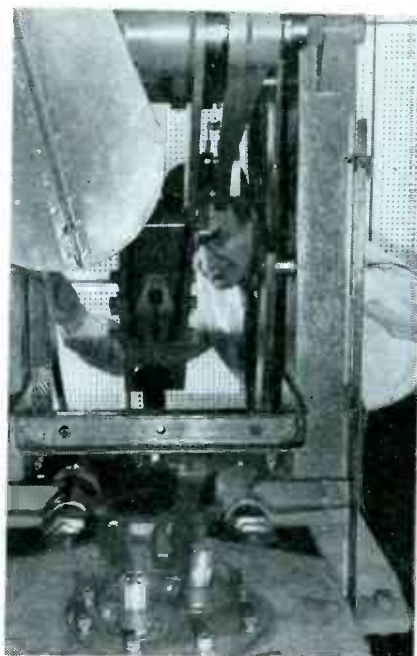
Tests at RCA Labs. indicate that special tubes withstand repeated impact shocks of 100g for extended periods
