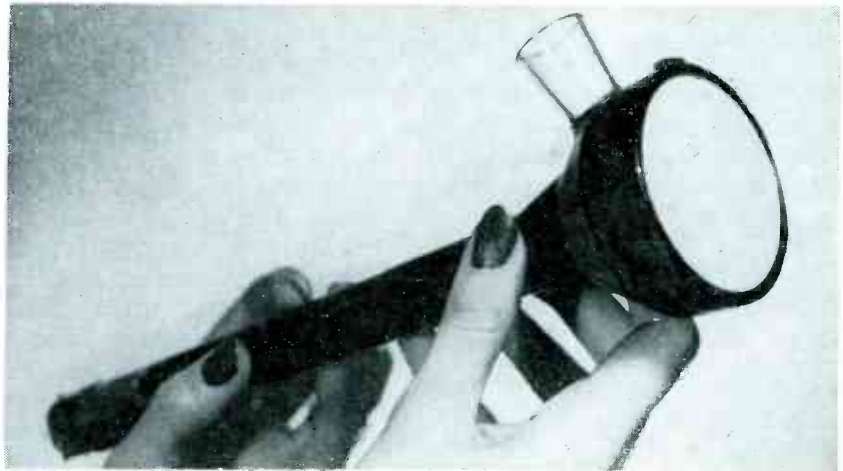
Special 2.5-inch diameter c-r tube developed for use in projection box
