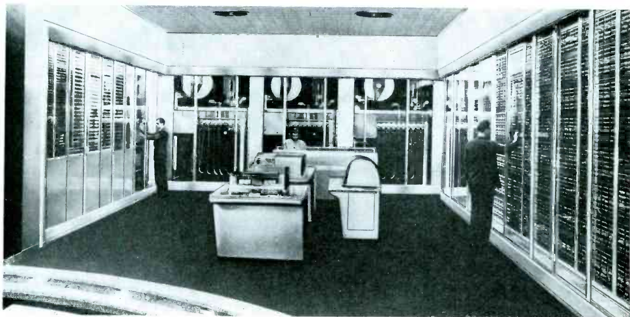
Electronic calculator, put into operation from punched cards, uses punched tapes for slowly moving computations, relays for faster operations, and vacuum tubes for high-speed manipulations. Computing elements are air-conditioned behind glass panels
