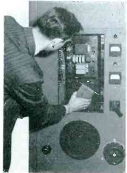
A chemist places cell in position for an x-ray comparison test
