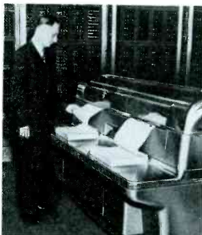
Computational results are printed as obtained, or can be stored on punched cards for later reference
