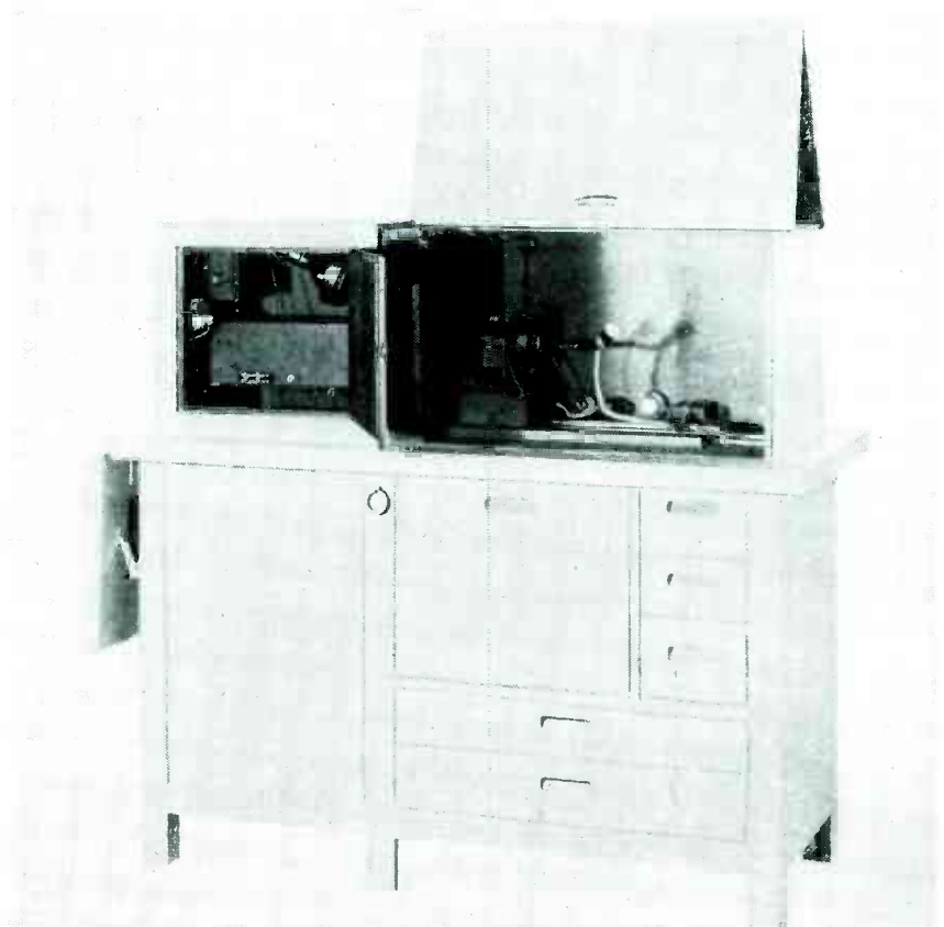
Light-tight console accommodates all shapes of cathode-ray tubes
