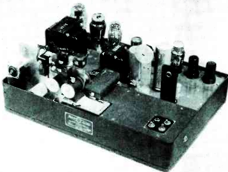
Precision electronic chronograph used to measure time interval between radio signals corresponding to passage of airplane through first and second equisignal beams
