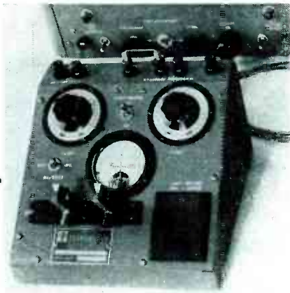
Panel controls and contact jigs of the bridge unit and accessory electronic unit
