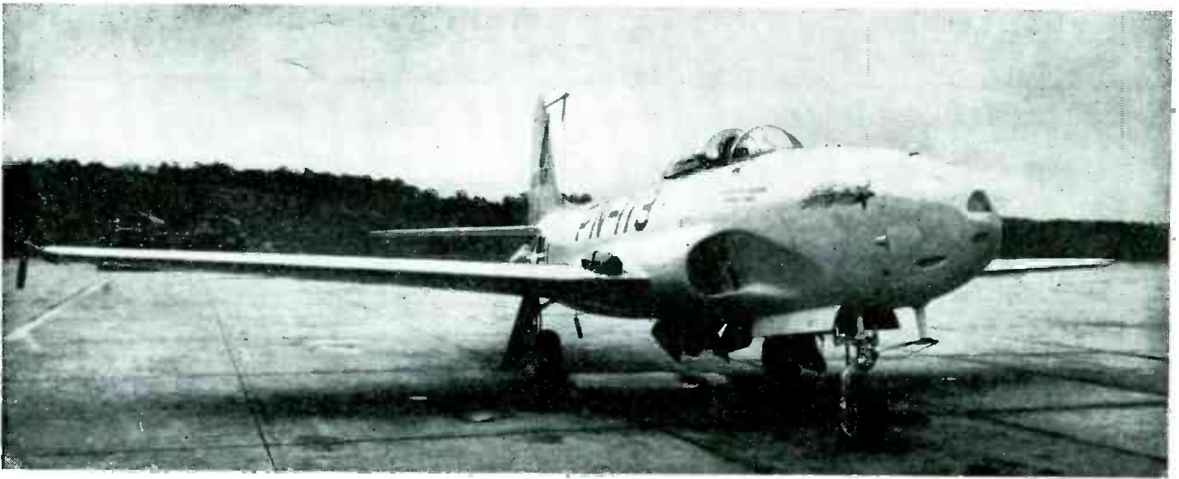
One of the P-80 jet-powered airplanes used in trials of new AAF speed course. New AAF streamlined localizer receiver antenna, a part of the airborne speed-measuring equipment, is installed beneath the nose
