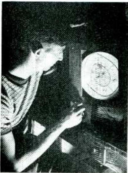
In the deflection test, the test pattern from the monoscope shows vertical and horizontal linearity, contrast, resolution, definition, and transient interferences
