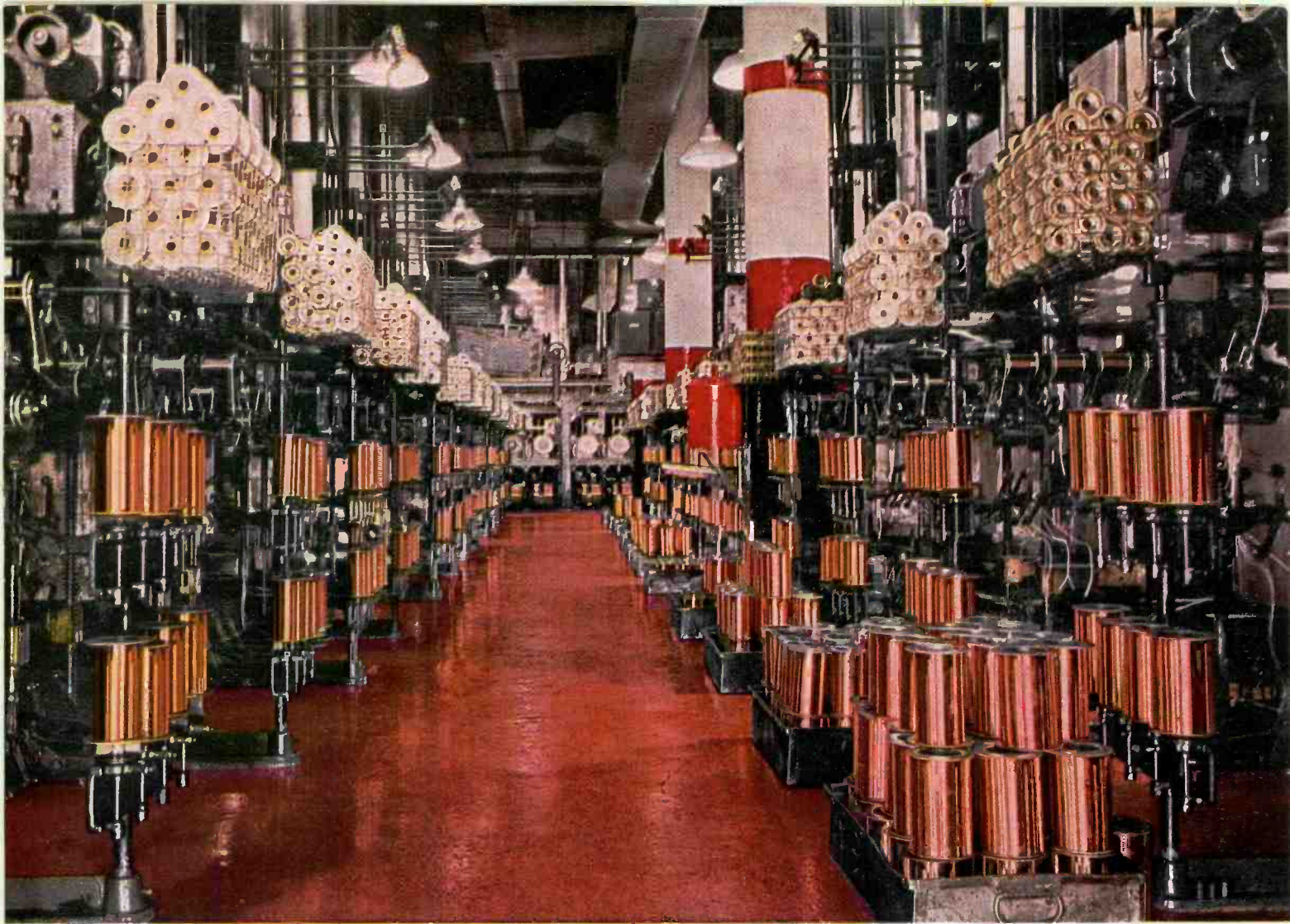
Section of the Belden enameling department, where Beldenamel Magnet Wire is produced.
