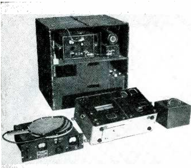
Control equipment includes the RBF-1 converted f-m receiver and loop at left, modified NK-2 recorder and the keyer. The BC-463A transmitter is at the rear
