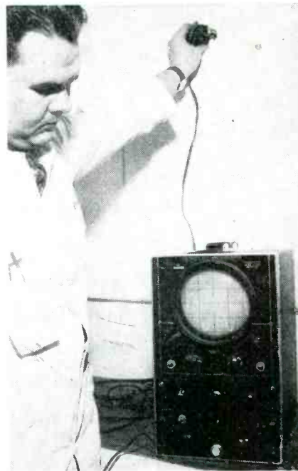
Reversal of polarity shown on the scope screen indicates location of faults in screening
