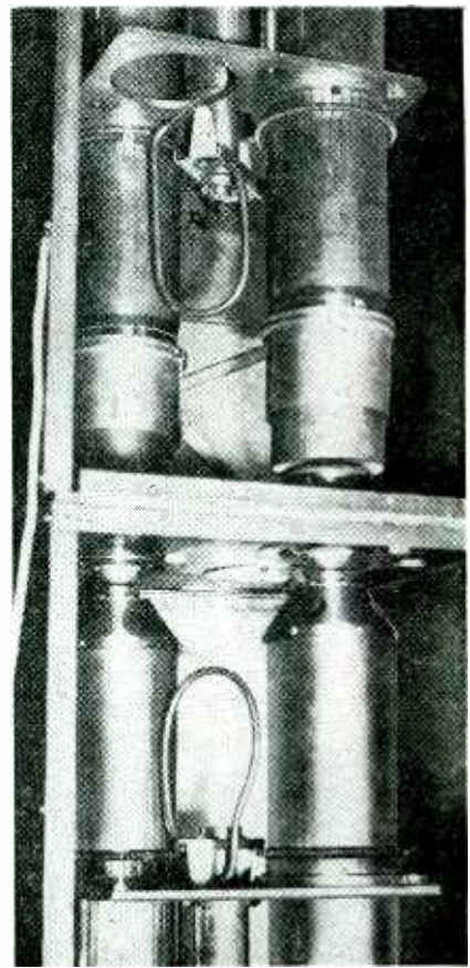
FIG. 3—13-kw push-pull stage, anode tank at top and cathode tank at bottom
