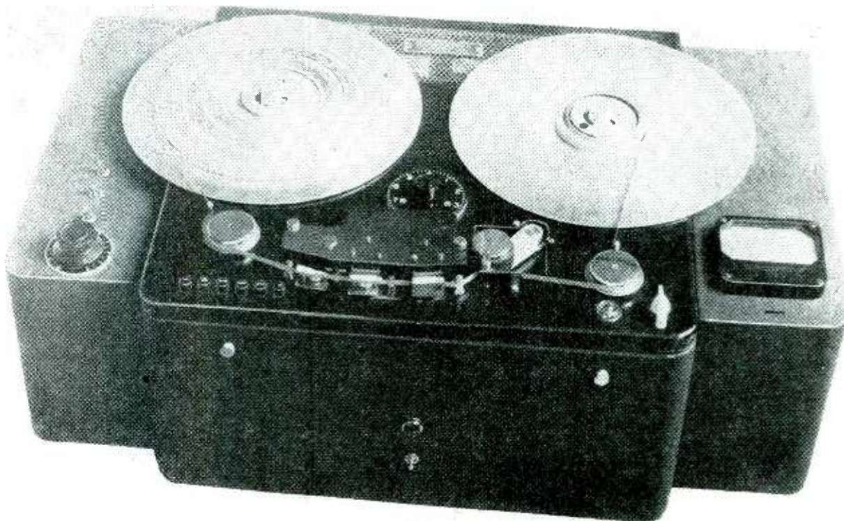
Initial production model of the magnetic tape recorder. Tape runs from left to right. The recording, erasing, and playback head is front and center
