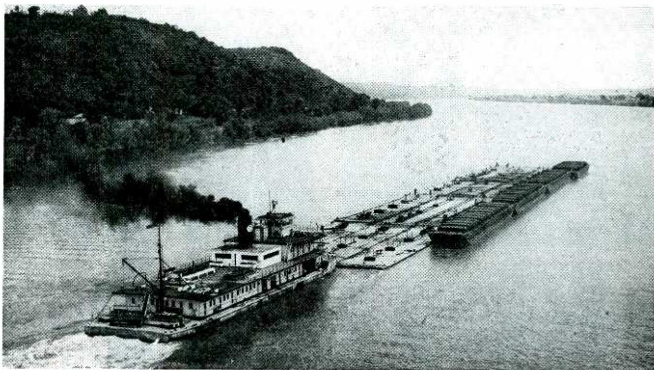
Radar-equipped, the Standard Oil towboat SOHIO SOUTHERN, pushes 12 barges containing 15,750 tons crude oil and four empty barges up the Ohio River
