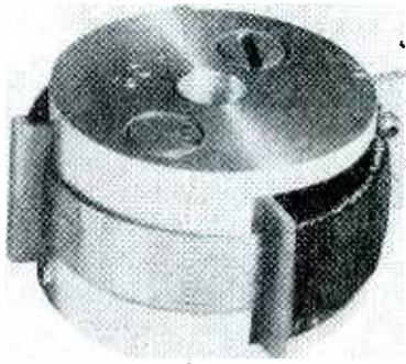
FIG. 2—Typical recording head removed from the assembly
