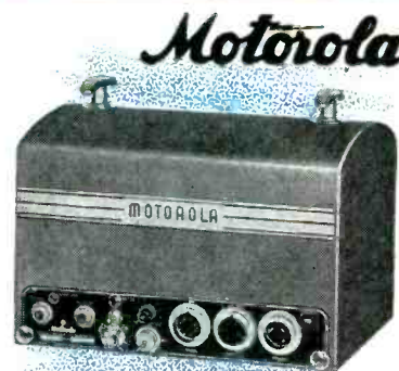
5516's power both driver-doubler and final of Motorola's Model FMTRU-30D.
