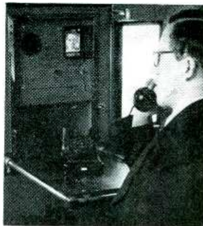
Telephone position includes lighting, iconoscope (behind round dark opening), and kinescope (in recessed box)
