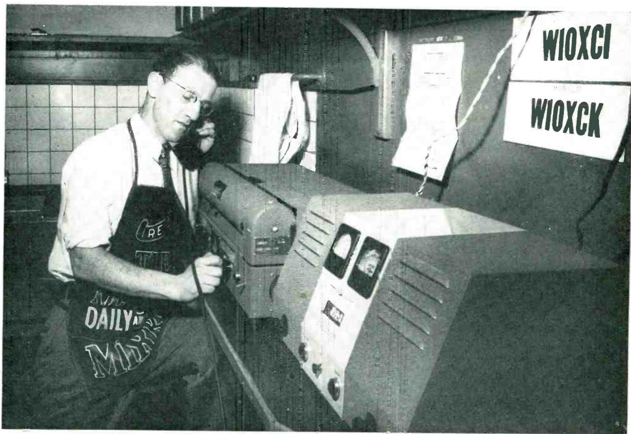
Darkroom used as control point for the experimental picture transmission system. At a warning signal from the mobile transmitter, the picture apparatus is connected and the control man refrains from using his transmitter until conclusion of the picture
