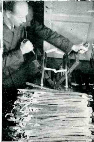
Rectangular copper conductors, insulated with Natvar Varnished Fibreglas Tape, are wound into coils. They are then formed for installation in locomotive motors.
