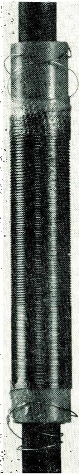
FIG. 5—Blown up to show the three different pitches formed in the winding process, this oscillator coil is used to track with the r-f coil shown in Fig. 3
