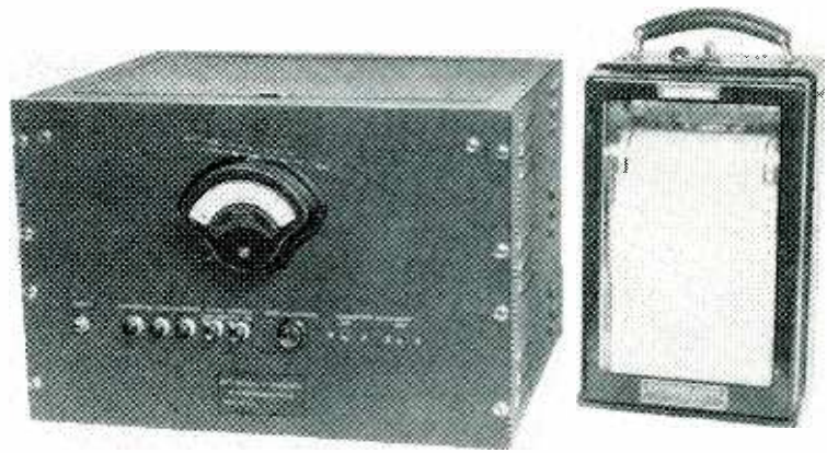
Indicator and recorder for converting pulse signals to a meter reading or permanent record. This unit can be remotely located from transmitter-receiver equipment
