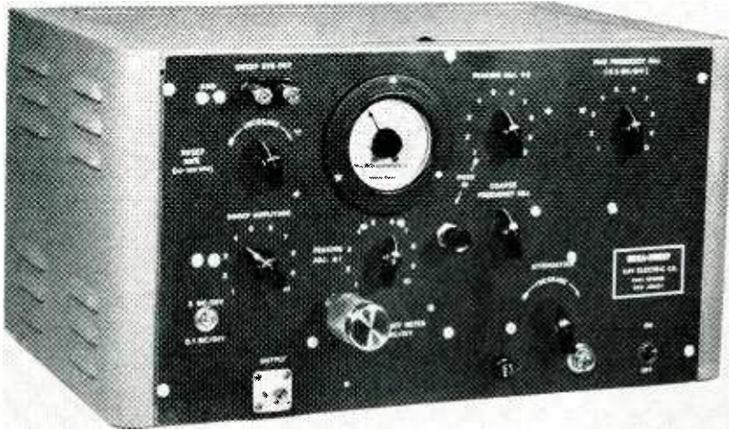
Controls for frequency tuning and sweep adjustment are on front panel of the wide-range sweeping oscillator. There is also a precision tunable resonant cavity for frequency measurement
