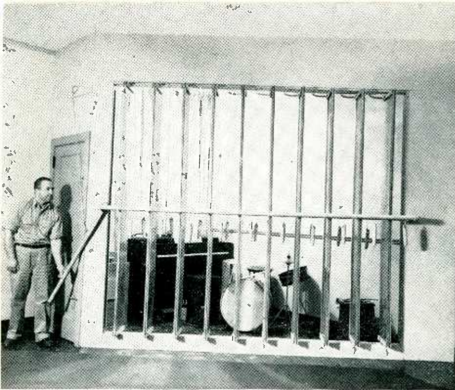
Movable panels between audience and talent permitted response to be cut off at 5,000 cycles. Panels were concealed by a curtain during actual tests
