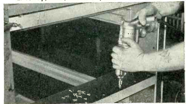
The complicated assembly of the drawer of the ICEBERG REFRIGERATED LOCKER . . . made without driver skids to injure work or hands, thanks to Phillips Screws. Most of the thousands of Phillips Screws used in this assembly are Type "A", self-tapping, and are power driven up, down, and sideways.
