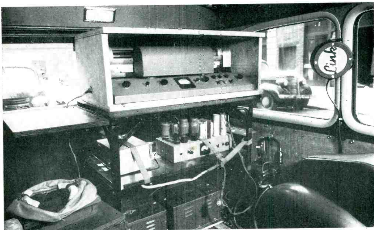
Interior of the Jeep station wagon. Standard mobile f-m communications equipment is on the floor. Immediately above are the dynamotor and picture frequency standard, with the Scundphoto machine in a lead-lined box on top of the table
