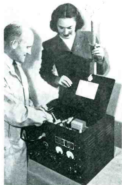
Designed for Coast Guard by G-E engineers, this microwave beacon acts as a lighthouse for radar-equipped ships
