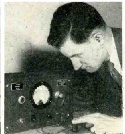
Thickness of a paint spot is measured with the electronic micrometer by its designer M. L. Greenough of the National Bureau of Standards electronic instruments laboratory
