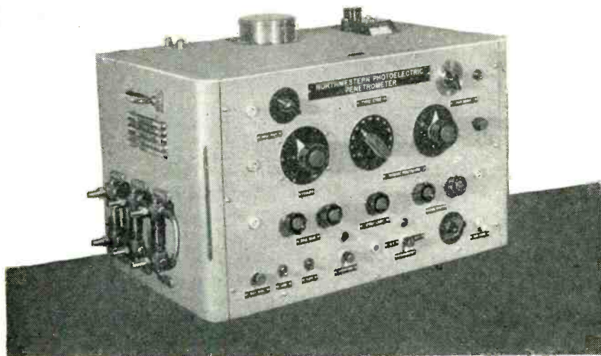
External view of the photoelectric photometer, or penetrometer. Smoke manifold is at the left
