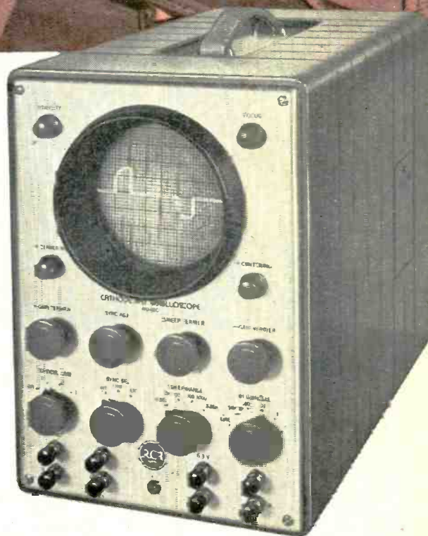
The new RCA WO-60C oscilloscope as used to adjust the ignitron circuit of a resistance welder.
