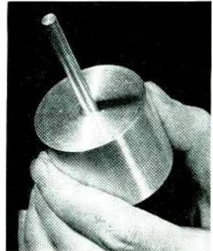
Fig. 1—Rod and cylinder used to illustrate electrical method of solving thermal problems
