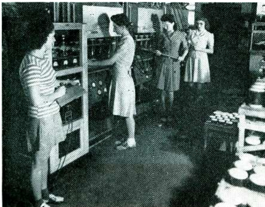
Steps in the processing of type 3BP1 cathode-ray tubes. From left to right, the operators are recording test results, preparing tubes for evacuation, using high-frequency heat to drive off occluded gas from elements during exhausting, and connecting heater, cathode and other tube elements for test. Because of heat, girls wear shorts at the Dobbs Ferry plant of North American Philips
