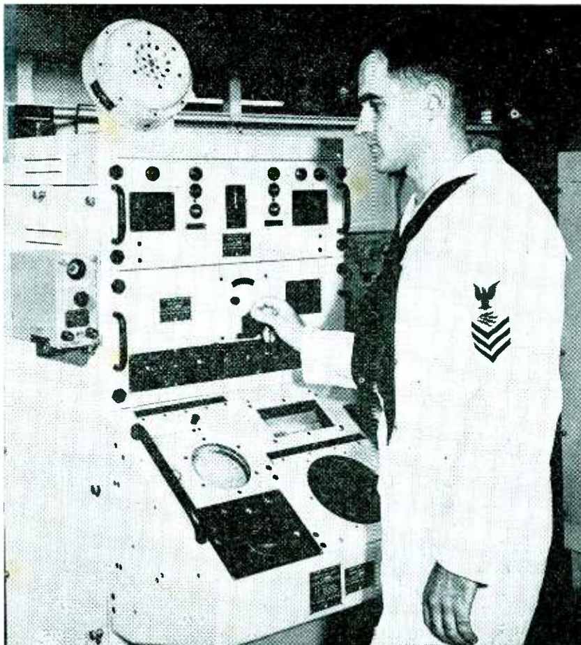
Control console of representative modern echo-ranging sonar, showing operator tuning the equipment. Training handwheel is at lower right of slant panel on which is the neon-type indicator
