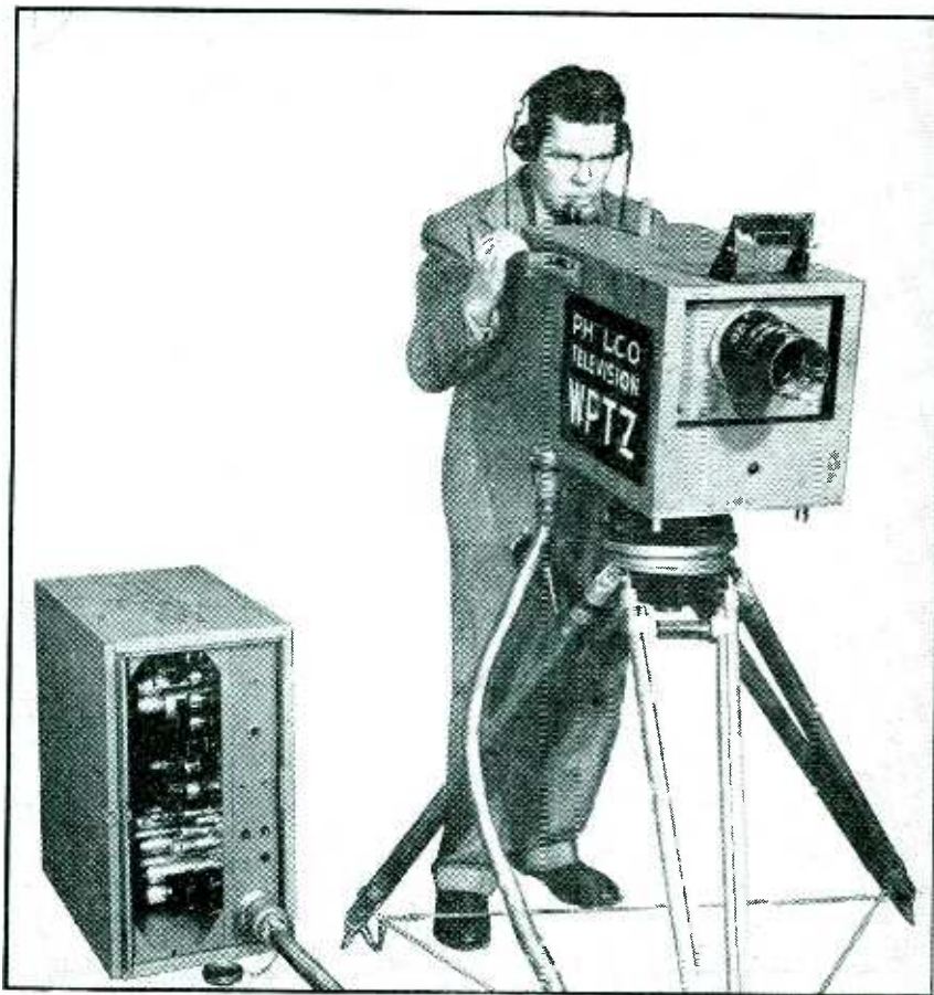
New 35-pound television camera, connected by cable to suitcase-type portable camera auxiliary unit
