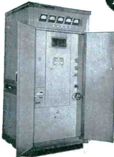
1 KW FM TRANSMITTER
