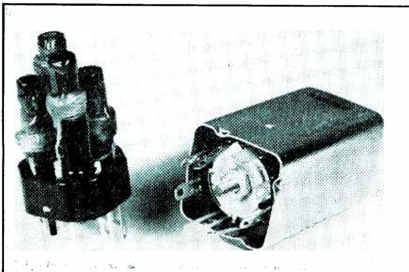
FIG. 2—Composite i-f transformer for 455 and 8.3 mc. The silvered mica discs show at the bottom of the shield can
