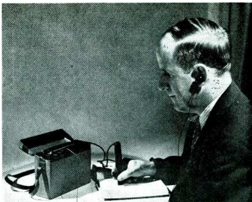
To read a printed page, a blind person moves the scanning stylus along each line of type. The electronic reading aid converts the shape of the letters into sounds
