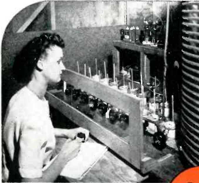
Checking mica capacitors for current carrying ability on high frequency.
