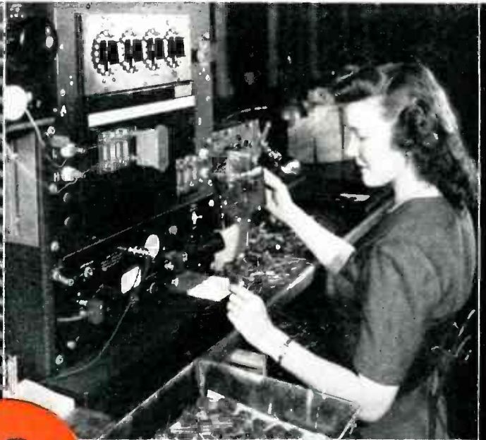
The above operator is shown checking a capacitor on a precision bridge.
