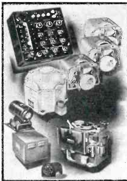
Automatic units controlled by the formation stick in the C-1 electronic autopilot
