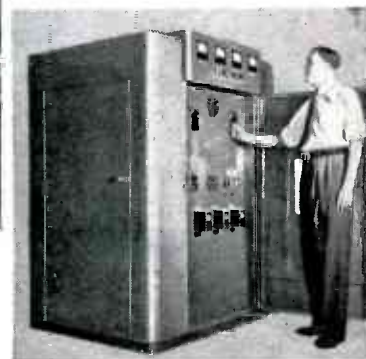
Up to 50,000 BTU of heat per hour can be delivered to the work through electronic platens from this RCA 15-kw generator. Operating cost (total) is only 35¢ per hour. Higgins uses this type of unit.
