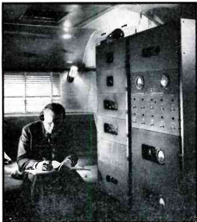
FIG. 7—Interior of a trailer, showing the operator talking to men at other points of the network via farmer's phone line
