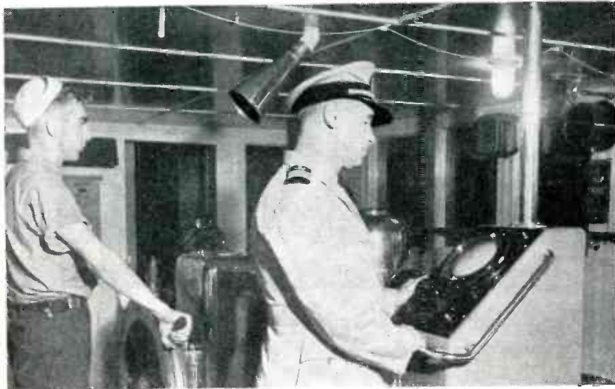
In the wheelhouse of the American Mariner, Captain Joseph Masse studies the screen of the cathode-ray tube in the General Electric radar navigator for commercial shipping. On the Great Lakes alone, more than 4,000,000 gross tons of cargo space were lost in 1943 because of the hazards of navigation through fog
