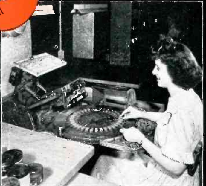
The above picture shows an operator color coding capacitors on special equipment used for this purpose.
