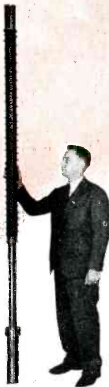
2,000,000 volt direct current precision radiographic tube, type VM
