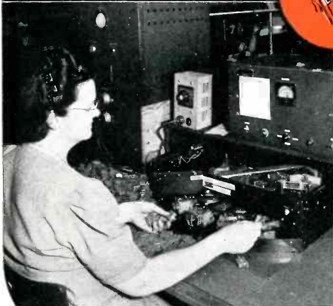
A view of the "merry-go-round" automatic checking equipment used for dielectric strength test.
