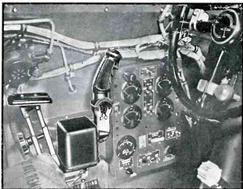
Installation of formation stick in B-17G bomber. Autopilot release switch is clamped on a spoke of the control wheel, 1½ inches in from the rim, and is pressed in case of autopilot damage by enemy fire, to restore all manual controls
