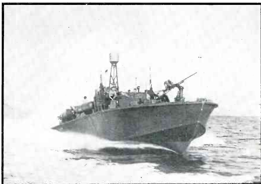
FIG. 4—A microwave search and warning radar on a PT boat. The dome structure houses the revolving parabolic reflector, or dish. Such radars were useful not only to warn of nearby air and surface units, but permitted accurate navigation among blacked-out ships and inside enemy harbors
