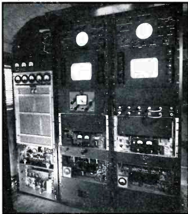
FIG. 8—Another view inside a trailer, showing one of the transmitters and the two rack-mounted monitor units
