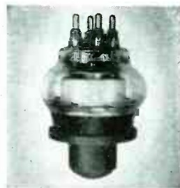
The ML 880 is a radio oscillator tube for use in transmitters, and has a maximum output of 60KW.
