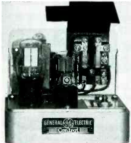
Typical of the small control devices mentioned is this general-purpose photoelectric relay
