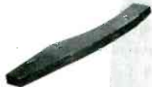
Forming Dies of Laminated INSUROK, shown here through the courtesy of Republic Aviation Corporation.
