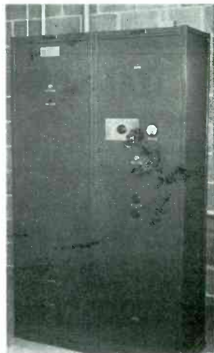
Unattended crystal controlled receiver for the radio link
