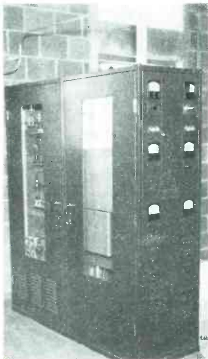
Complete unattended remote controlled transmitter
