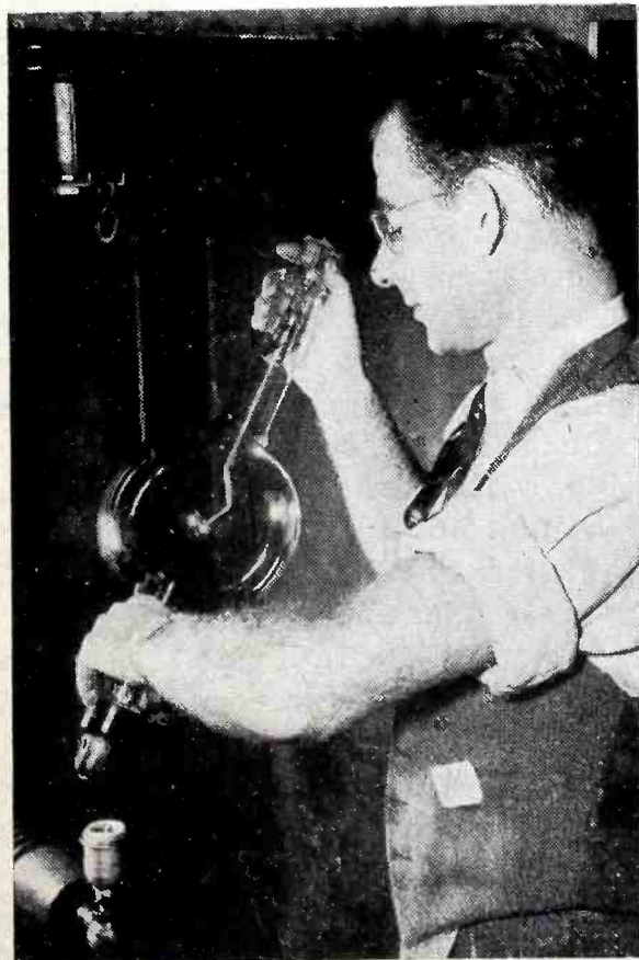
Installing a 150-kv radiation-cooled deep therapy tube in a lead-protected testing chamber. The operator carries a piece of x-ray film (clipped to his vest pocket) that is developed and replaced at regular intervals as a check on the system of x-ray protection
