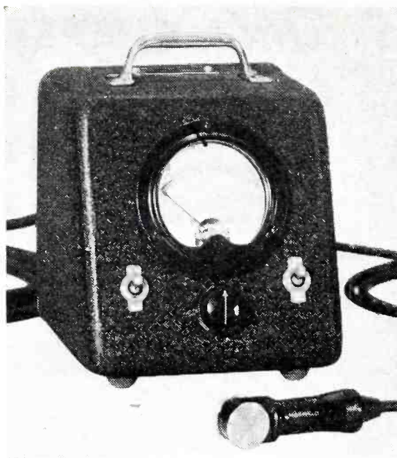
Fig. 2—Thickness gage for measuring paints, lacquers, and nonmagnetic babbitt linings on steel bearing shells
