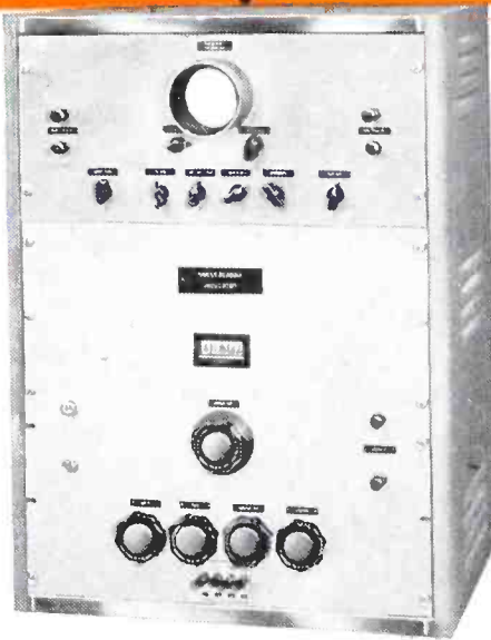
(C) The UTC oscillator is direct reading, where the frequency desired is set as in a four digit decade box, and is accurate within 1 cycle at 1,000 cycles. The range is 10 cycles to 100 kc. Accuracy of this type is essential with filters having sharp attenuation characteristics. This instrument is augmented by a UTC harmonic analyzer for the output measuring device.
