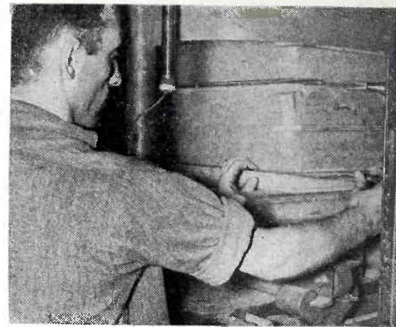
Mounting sheets of Pregwood (encased in thermal insulation) in an electrostatically heated press. Clips connect to copper plates on each side of the material to be heated
