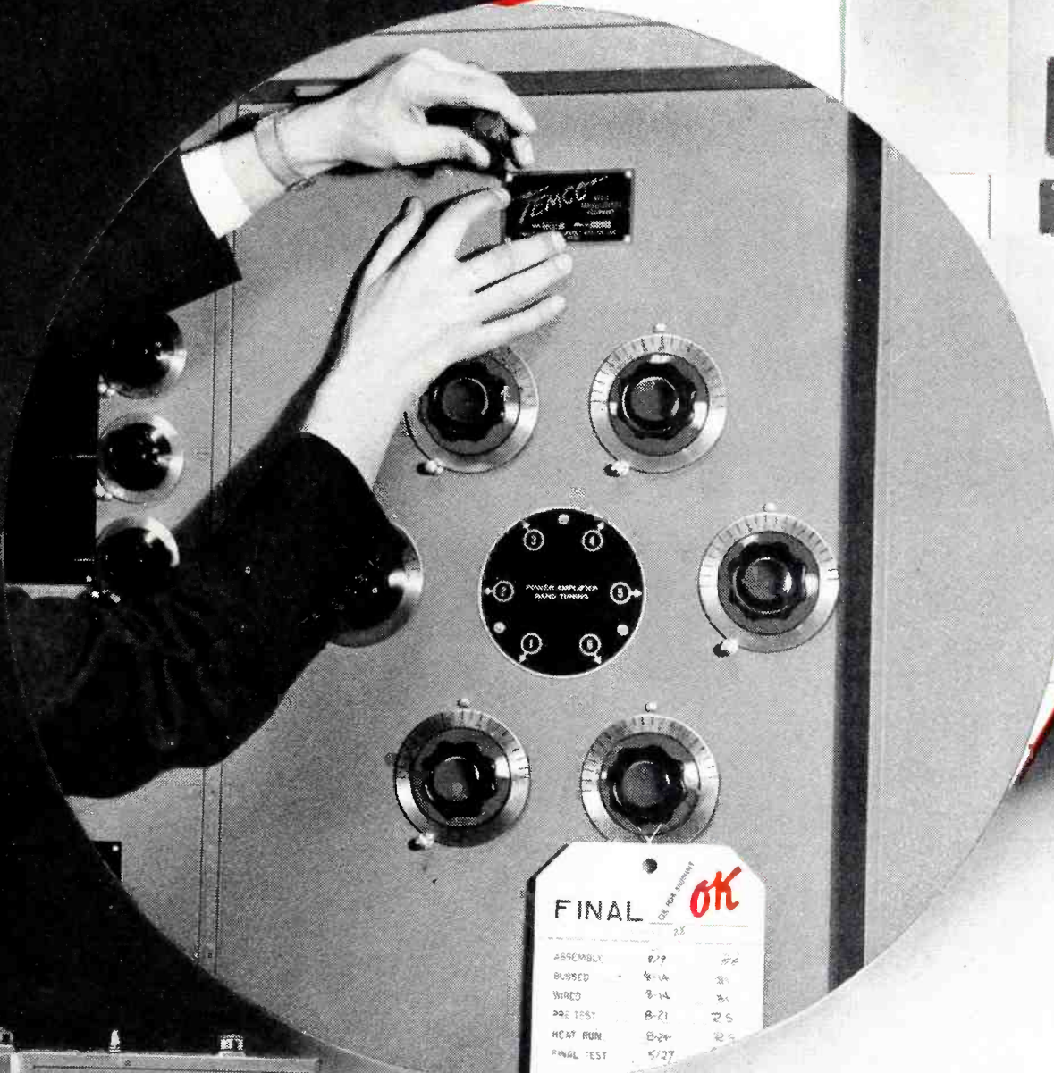
Above: TEMCO Model 1000 AG-CW 1000 watt radio telegraph transmitter with pretuned tank circuits for 6-frequency operation with motor driven frequency selection.
