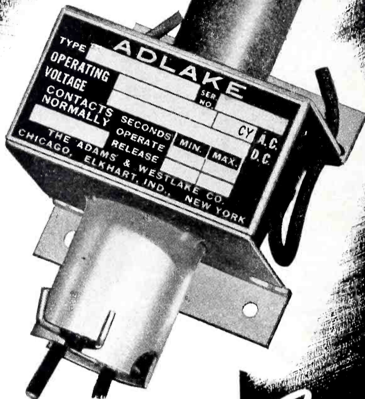
Adlake Relay No. 1040—(for A.C.) 5½" high, 2½" wide, 2⅜" projection. For panel mounting. Contact normally open or closed. Quick or time delay action. Contact protected by metal armor.
