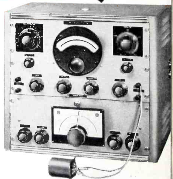
(D) The UTC Q meter is a unique device which has helped considerably in the development of the special core materials used in our filters. It is also of importance in maintaining uniform quality in our production coils. The Q is read directly and covers entire range of possible Q factors over entire audio frequency band.
