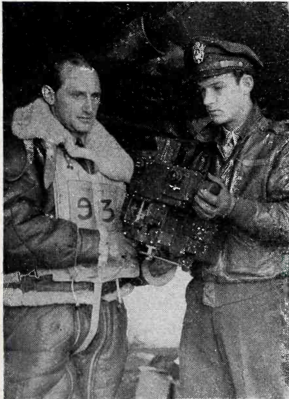
Shown here is the Sperry computing gun sight, a model of scientific precision, used on Flying Fortresses. The gun sight makes corrections for the factors such as plane and wind velocity which might otherwise cause a gunner to miss his mark
