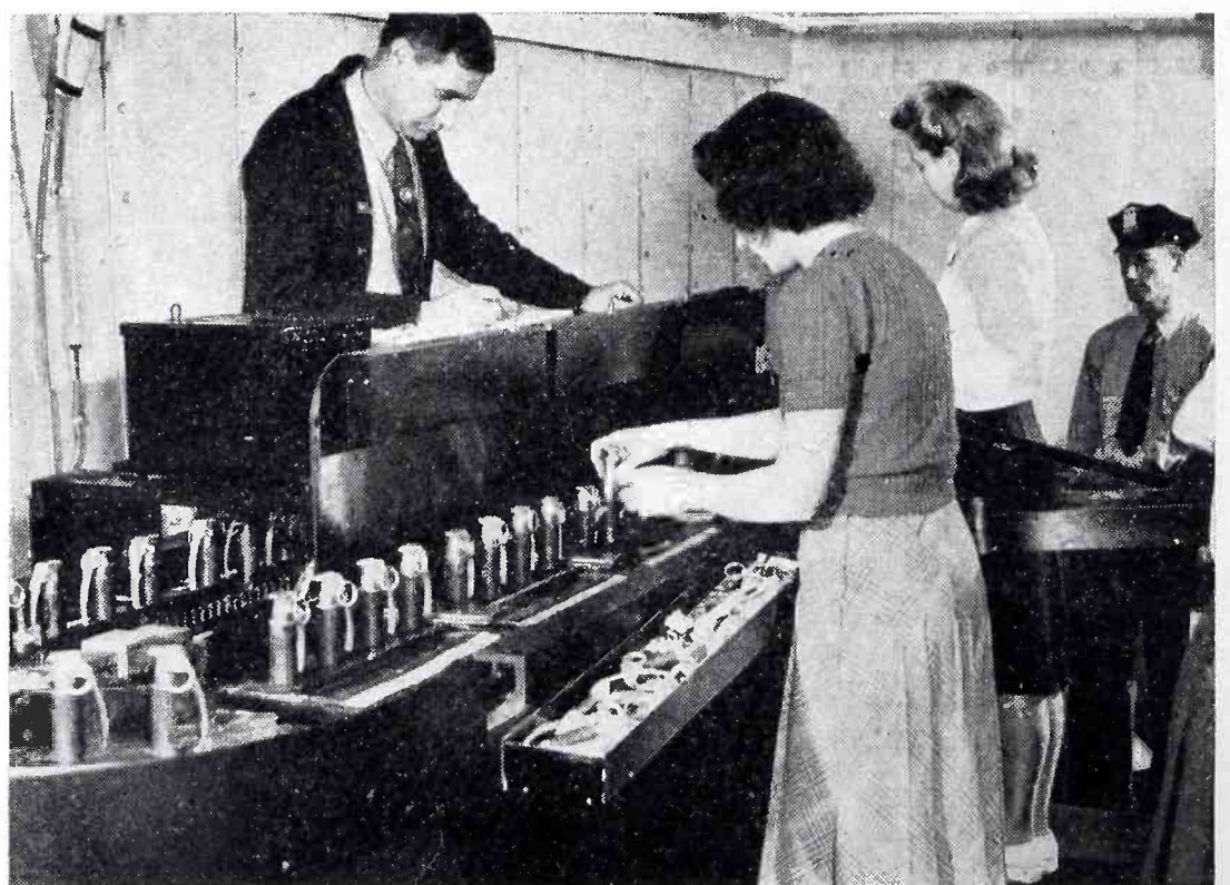
Hand-grenade fuses to be checked for powder content are placed in metal containers on a movable belt that takes them into an x-ray machine. The x-rays fluoresce a screen that is constantly watched by a phototube to detect a change of intensity caused by an insufficient charge of powder
