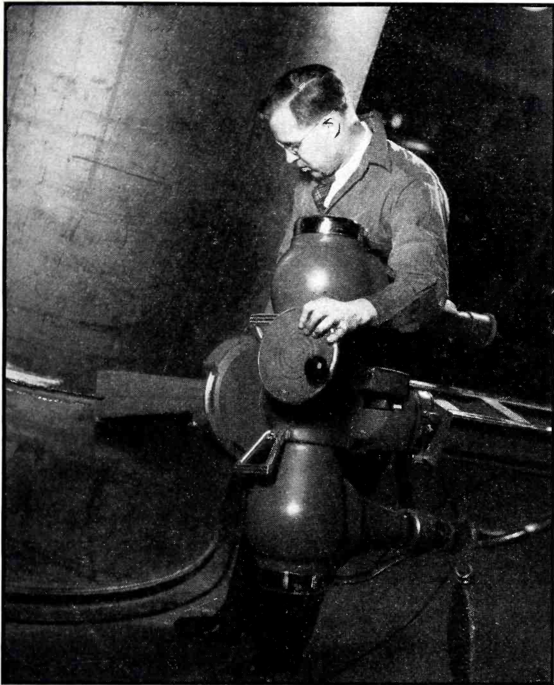
Using a 220-kv portable industrial x-ray machine for radiographic inspection of a weld in a steel transformer tank
