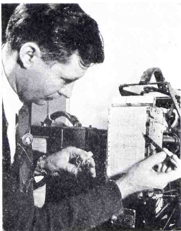
A defective fuse is red-painted by the x-ray machine, and is also detected by a long line on the meter graph. A bell and light warn the operator when the dud intercepts the x-ray beam
