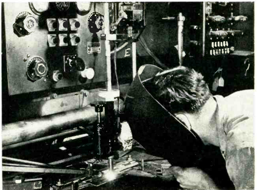
Automatic helium-shielded arc-welding equipment in use. The electronic control panel at the upper right controls arc length, while the main control panel at upper left handles all the other welding operations. The slanting tube at lower left feeds the filler wire into the arc. The tungsten starting electrode and the helium gas nozzle are perpendicular to the work, which is clamped to a moving bed
