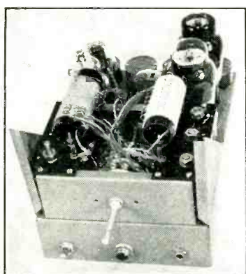
Series 20, 4 channel 1600-6000 KC, 20 watt transmitter.
