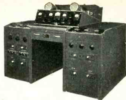
The test desk resembles a control console used by broadcast stations and provides quick testing of cathode-ray tubes
