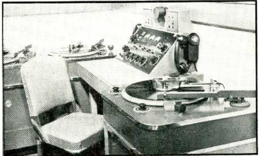
One of the transcription recording rooms. It can handle three transcribed programs simultaneously with only a single operator. Electromagnetic brakes hold each transcription stationary with the pickup in the selected position, with the turntable rotating continuously and the record slipping, so the operator can start all three programs at the same time by releasing the brakes
