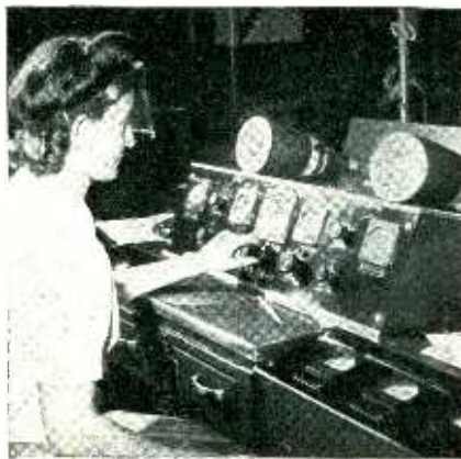
Production testing of cathode-ray tubes at a special desk that contains the necessary power supplies, controls and meters
