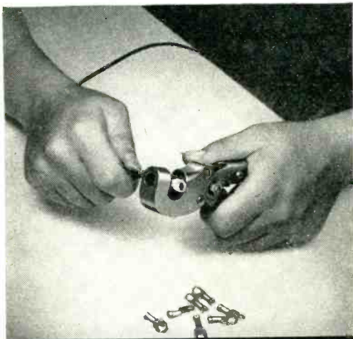
For small wire connections . . . Simply indent the HYLIN connector to the wire with the Burndy HYTOOL (pliers). A quick, simple operation requiring no skill.
