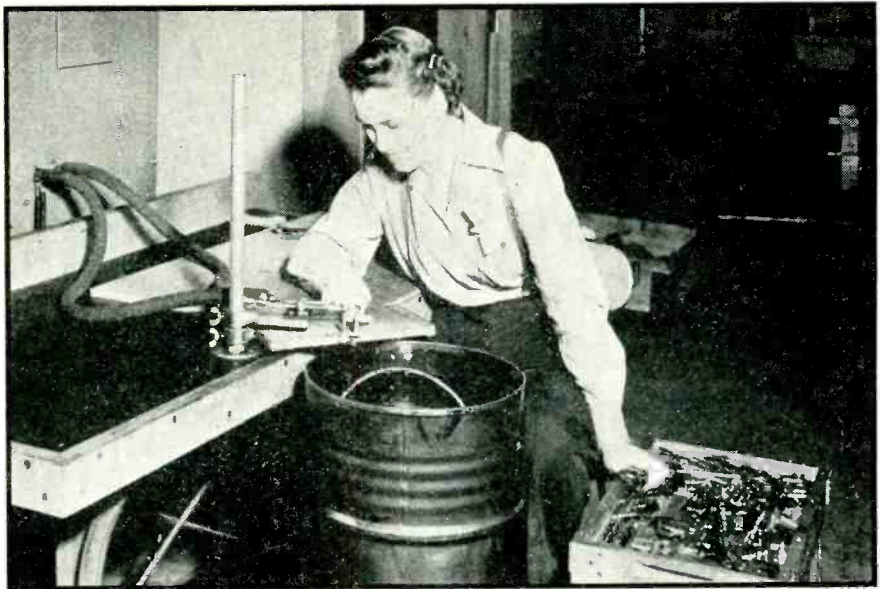
With the work coil, quenching barrel and stock box conveniently positioned in front of the operator, localized hardening is achieved efficiently with no excess heat to create discomfort. The spark gap type heating unit being used here is made by Lepel High Frequency Laboratories, New York City
