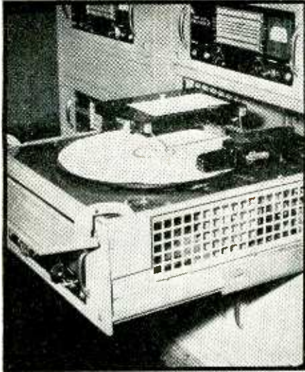
One of the two turntable drawers in each Memovox unit. Switching between turntables is automatic. Each turntable can emboss a one-hour program on one side of its flexible plastic disc, hence the units can run unattended for two hours at a time
