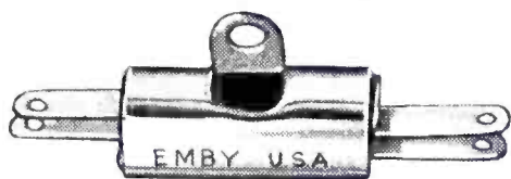
DL —Input 10 volts ac. Full wave bridge. Continuous dc 35 ma. Mounted in aluminum case with mounting extensions. Actual size.
