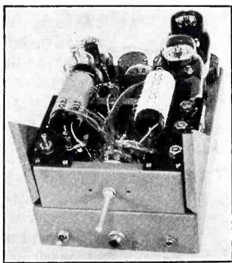
Series 20, 4 channel 1600-6000 KC, 20 watt transmitter.
