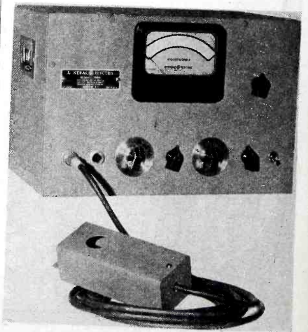
General Electric time interval meter, with phototube and preamplifier in separate housing
