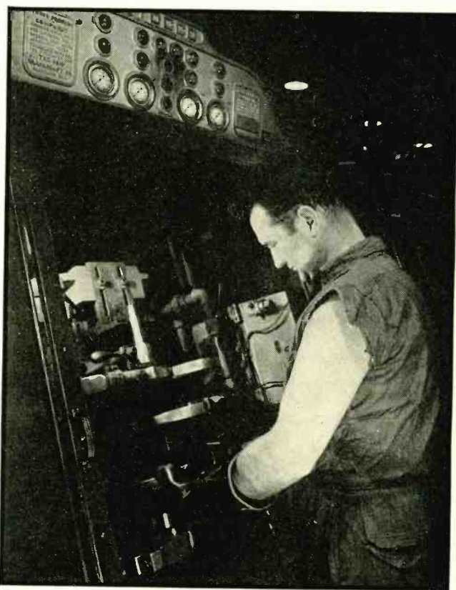
CRANKSHAFTS —This Ohio Crankshaft Company machine, powered by Westinghouse generators, hardens bearings in four seconds by inducing current into them from a collar constituting a single-turn coil. Distortion of the shaft is minimized as resulting heat is closely confined to the bearings
