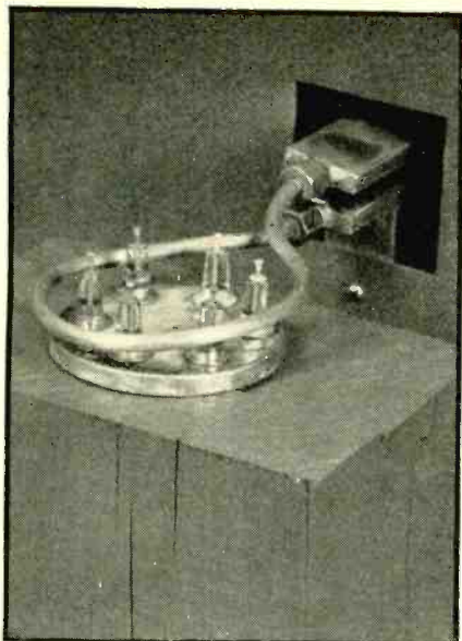
TRANSFORMERS —By wrapping short lengths of solder around terminals and then heating all of them at once by means of power induced from a single-turn coil RCA avoids the necessity for applying a soldering iron to each individual terminal
