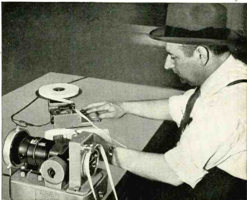
T. R. McElroy, world's champion telegraphist and outstanding wireless operator of all time, operating a development model of the new perforator in conjunction with Tape Transmitter, Model XTR-442.
