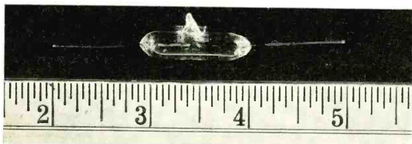
FIG. 3—Photograph of gas discharge tube used in making timing traces
