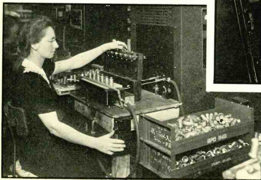
CRYSTALS —Here high frequency heat takes the place of gas heat in a G-E plant, soldering a protective shell to a base without overheating a frequency control unit mounted inside
