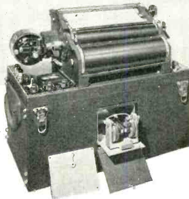
This Alden recorder was specially designed to produce facsimiles up to 8" width.
