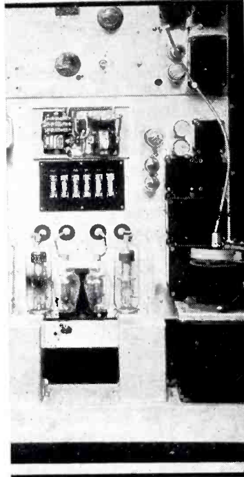
Front view of power supply units. The filament voltage control Variac at the lower right is operated through flexible shafting from the front panel
