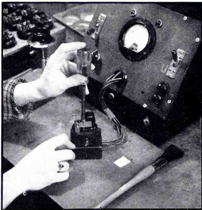
Third step in adjusting relay. Setting spring for drop-out at indicated current
