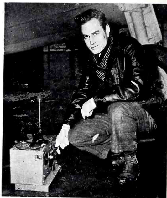
Edwin C. Tracy, RCA Victor Division employee, developed this special electronic oscillator for testing radio equipment in fighting planes
