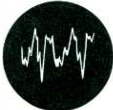
G-392 cycles per second as produced by a single reed of an accordion. Complex wave form is the result of reed being driven to a high amplitude, producing many harmonics or overtones.
