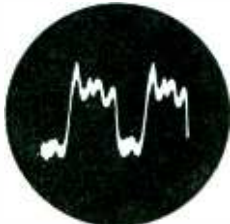
E-392.6 cycles per second as produced by the D string of a violin, with first finger in position. Since the entire body of the violin resonates, the tone is rich in harmonics and wave form will vary greatly from note to note.
