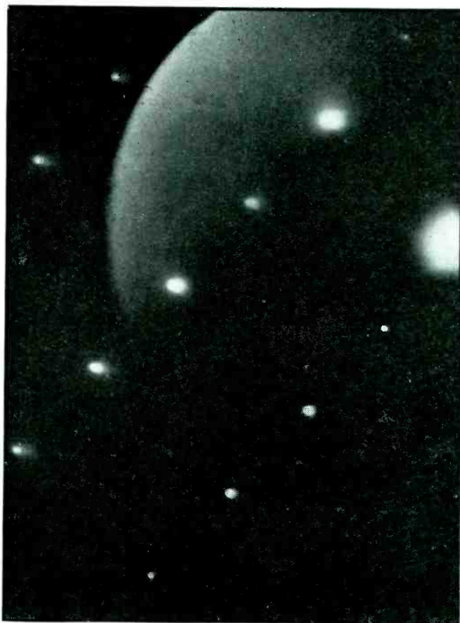
Diffraction pattern of a single silicon crystal permitting determination of lattice constants to within three-tenths percent
