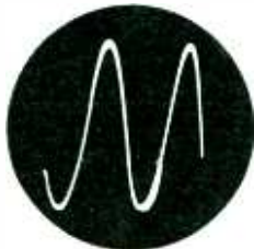
Sine waves of a tuning fork, A-440 cycles per second. Note the pure wave form absolutely devoid of harmonics. If secondary waves are superimposed on the fundamental wave, we have the harmonics or overtones which distinguish voices or instruments.
