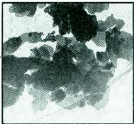
Lead arsenate. Good insecticide particles are in thin, small plates. \times 27,500
