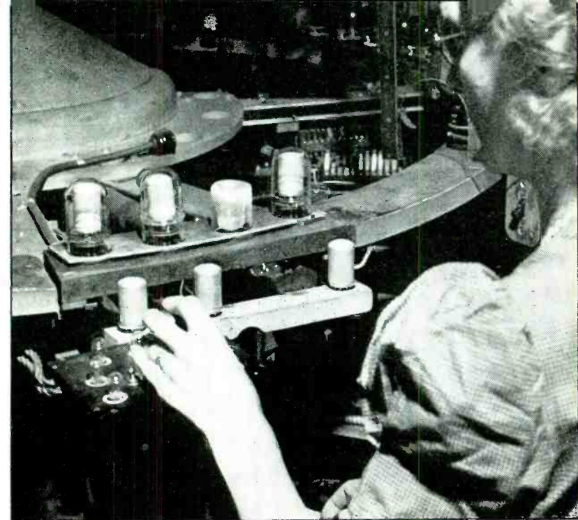
5 (Right) After completion of the exhaust, the tubes are aged 20 minutes in this rack at varying over-voltage and over-current conditions. By watching the lamps, the operator can tell the condition of each tube during the aging period
