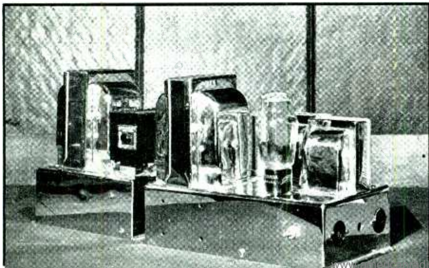
Fig. 5—Power supply which contains a high voltage supply and a CuO rectifier for the tube heaters
