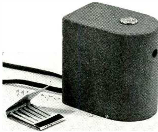
Fig. 10 — External view of a self-contained a-c operated phototube relay using the multiplier phototube
