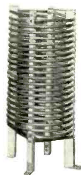
ES-675768 RF Isolation Coil for by-passing phase monitor sampling lines around tower insulator.
