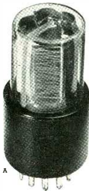
Fig. 1—The new phototube structure: A, external appearance; B, section showing glass barrier; C, the element structure viewed from the top
