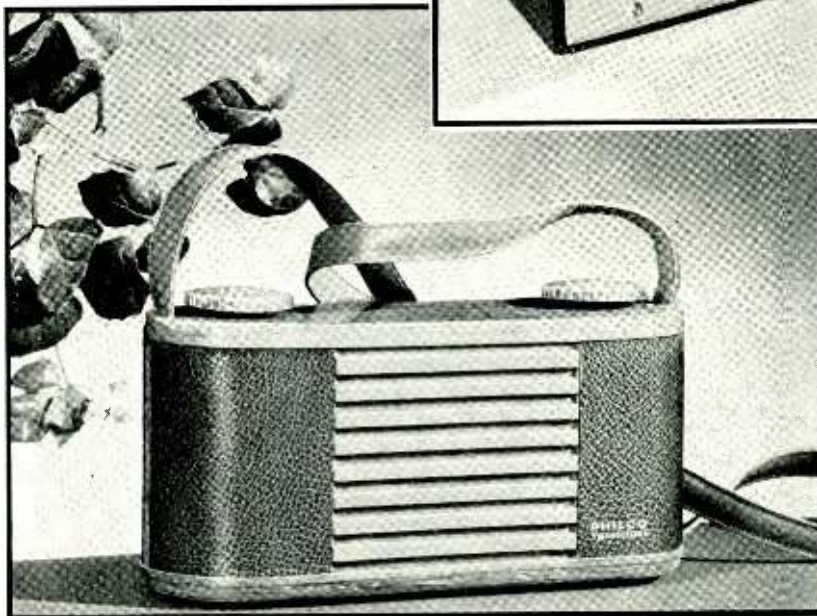
The antenna of the Philco set is contained in the shoulder strap. A low impedance loop is used to avoid dielectric losses in the body of the user
