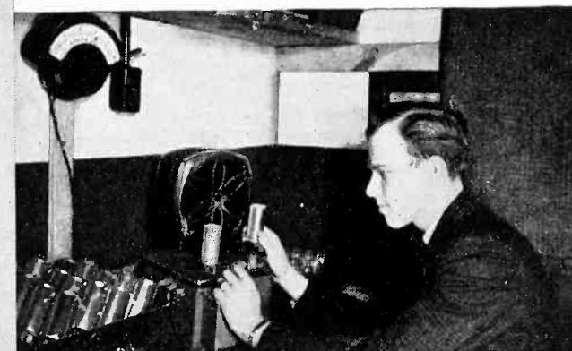
Every Mallory-built Vibrator is tested for noise in a sound-proof room under actual set-operating conditions. This has been established as the only practical and conclusive test of the noise factor.
