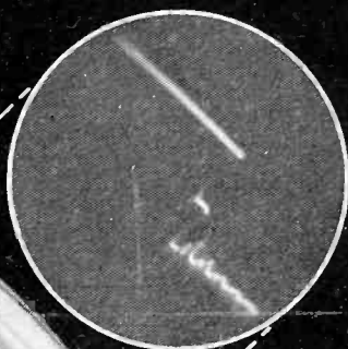
Photograph of a high-speed transient taken with the 326C tube. Fundamental frequency of oscillation is 1 megacycle, with 3 megacycle component showing. Vertical line (right) represents a spotspeed of 63 Km/sec. on screen of tube.
