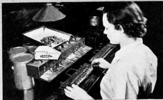
Progressive assembly of internal mechanism. All parts are checked for thickness, being placed in order in this "trolley", where they travel to the next operator in the assembly line.
