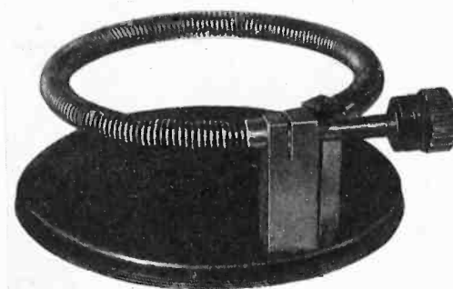
This multiple scale may be applied to complete circles or even to spirals. This feature considerably broadens its field of application
