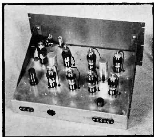
Fig. 7—Rear view of the shading-signal generator. Eight double-triode tubes are used to develop the correction signals to remove the dark spot
