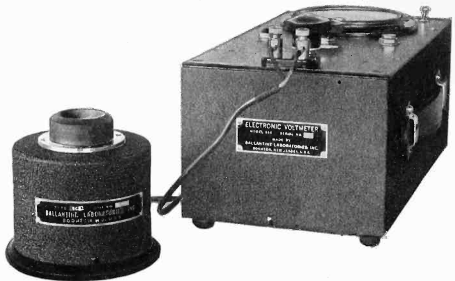
Fig. 1—The artificial ear, shown above, consists of the acoustic chamber, a pressure-operated microphone and an electronic voltmeter to measure the microphone voltage
