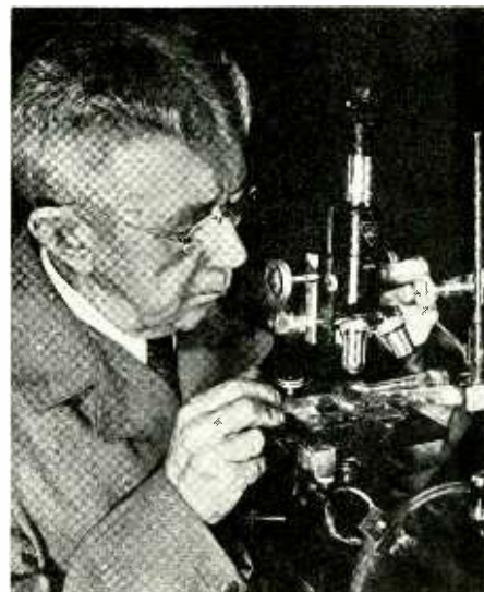
Microscope fitted with ultra-violet "death-ray" tube
