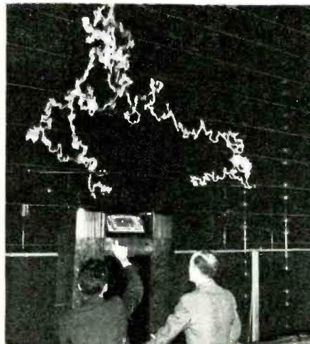
Receiver set up in Steinmetz Hall for artificial-lightning noise studies
