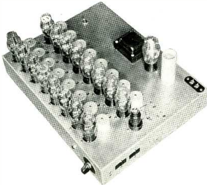
Fig. 2—Top of chassis showing arrangement of tubes and parts. The outputs of the 15 beat oscillators and the master oscillator are mixed in the 6L7 (metal tube)
