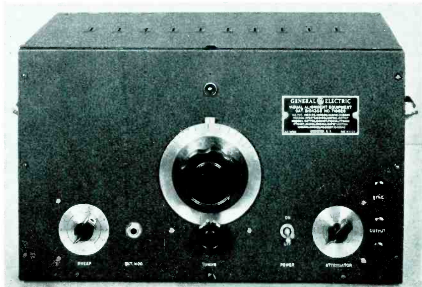
Fig. 4—Oscillator and frequency modulator. The pyramid wave acts on the control tube to vary the frequency in the oscillator
