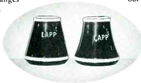
Left, early Lapp Compression Cone. Right, curved side compression cone—same dimensions, wall thickness and weight—twice the compression strength of the straight side cone—the design used in all footing and guy insulators (see below) since 1932.
