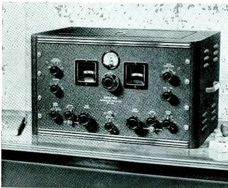
The new and improved Hammarlund Super-Pro Receiver. New features include a variable-selectivity crystal filter, a noise limiter and an "S" meter
