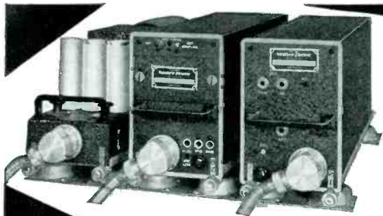
Western Electric 1A Radio Altimeter instantly indicates the distance of an airplane above the terrain underneath by timing an ultra high frequency wave sent straight down from the plane and reflected by the ground.
