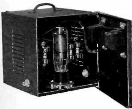
Small portable single-phase rectifier for supplying 250 watts D.C. at 115 volts
