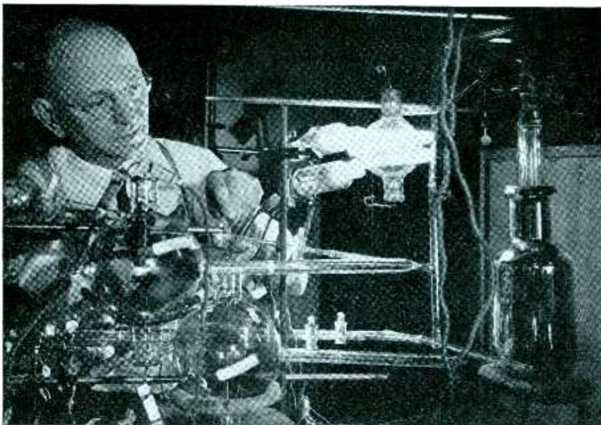
Thorough evacuation in which the tubes are freed from contaminating gases is an essential operation in the manufacture of gas filled as well as vacuum tubes. Mr. W. A. Ruggles is shown operating the gas purification system used in conjunction with exhaust equipment in the Research Laboratory of the General Electric Co.
