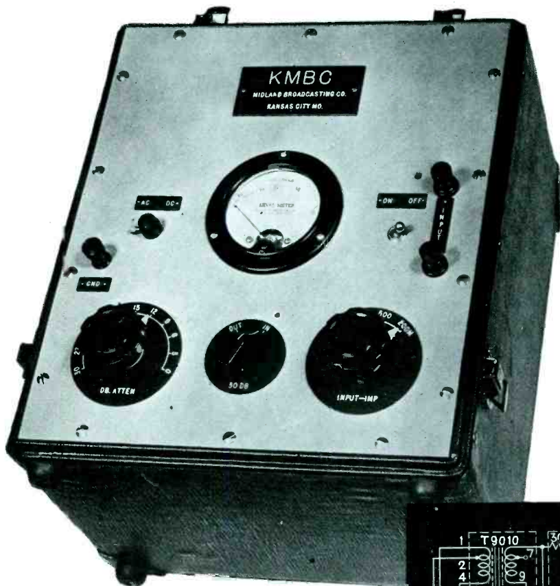
Fig. 2—Above, level indicating meter with a range from -65 db to 12 db, and with input impedances of 50, 200, 500, or 200,000 ohms
