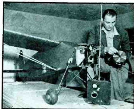
This model airplane, built in California, will take off, maneuver in the air, and land, in accordance with radio signals emitted from a portable transmitter
