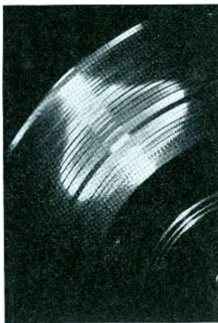
Fig. 2—Example of the use of response patterns. The cutter alone produced a pattern (below) having poor high frequency response. With some equalization (upper right) the highs were brought up. Attempts to introduce more equalization produced on objectionable peak (right) in the middle-frequency range, due to improper shape of the equalizer curve
