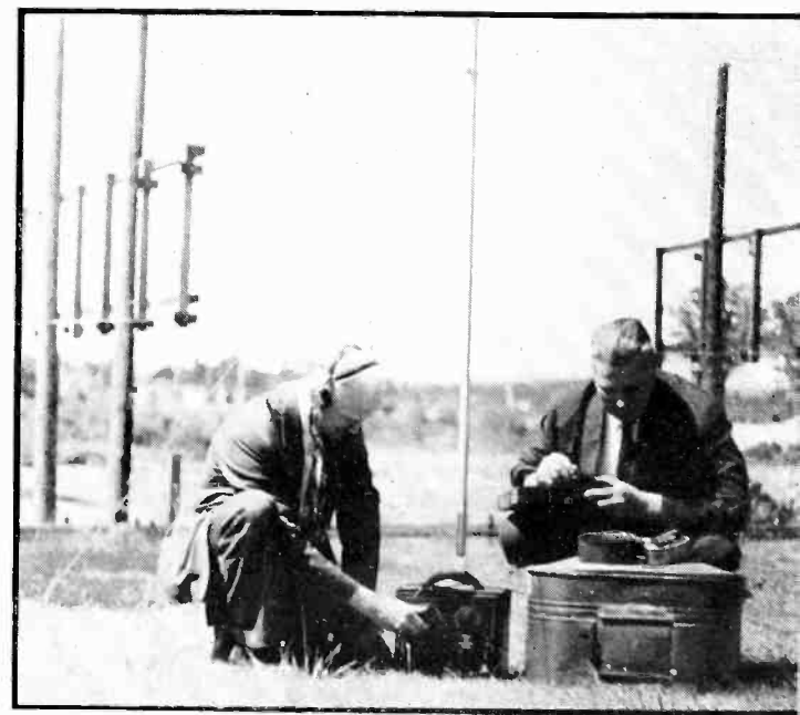
H. O. Petersen and H. H. Beverage with field strength measuring set, a Radiola and the first h-f signal generator in a wash boiler
