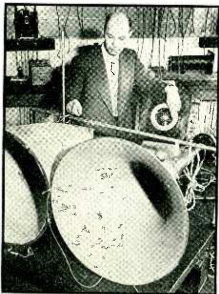
A source of high intensity sound sent from an airplane through the horn on the right is received after reflection from the ground. The delay between sending and receiving, which measures the height of the airplane, is indicated directly on a meter. Lieut. L. P. Delsasso of University of California is the inventor
