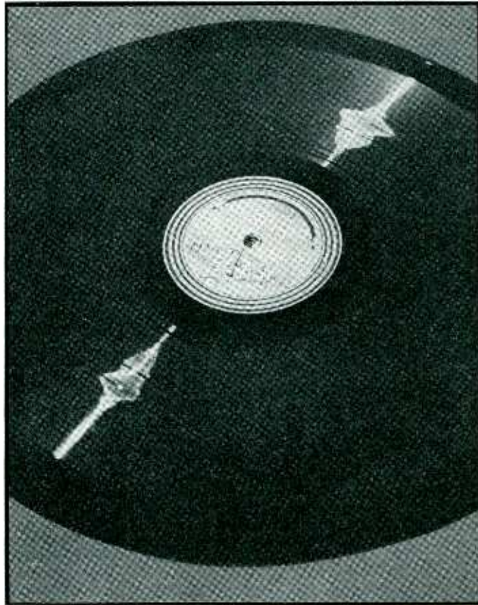
Checking frequency response is an important part of the new recording techniques. Above, "Christmas Tree" patterns on a Rangertone frequency-run record adjusted for a peak at 2000 cycles (see text, page 10)
