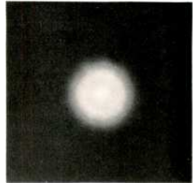
Pattern secured from transmission of electrons through film about 10^{-6} cm. thick
