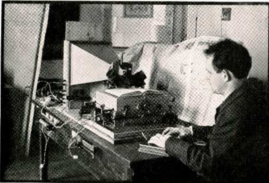
This device enables blind persons to read any book. A phototube slowly scans each line, the impulses being transmitted to a special desk, where the blind person interprets them by his sense of touch. The device was developed by the Ukrainian physicist, A. G. Goldman
