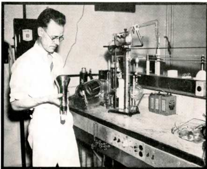
Mr. Farnsworth with two pick-up devices. The image dissector in his left hand produces an electron picture from the visual image focussed on it
