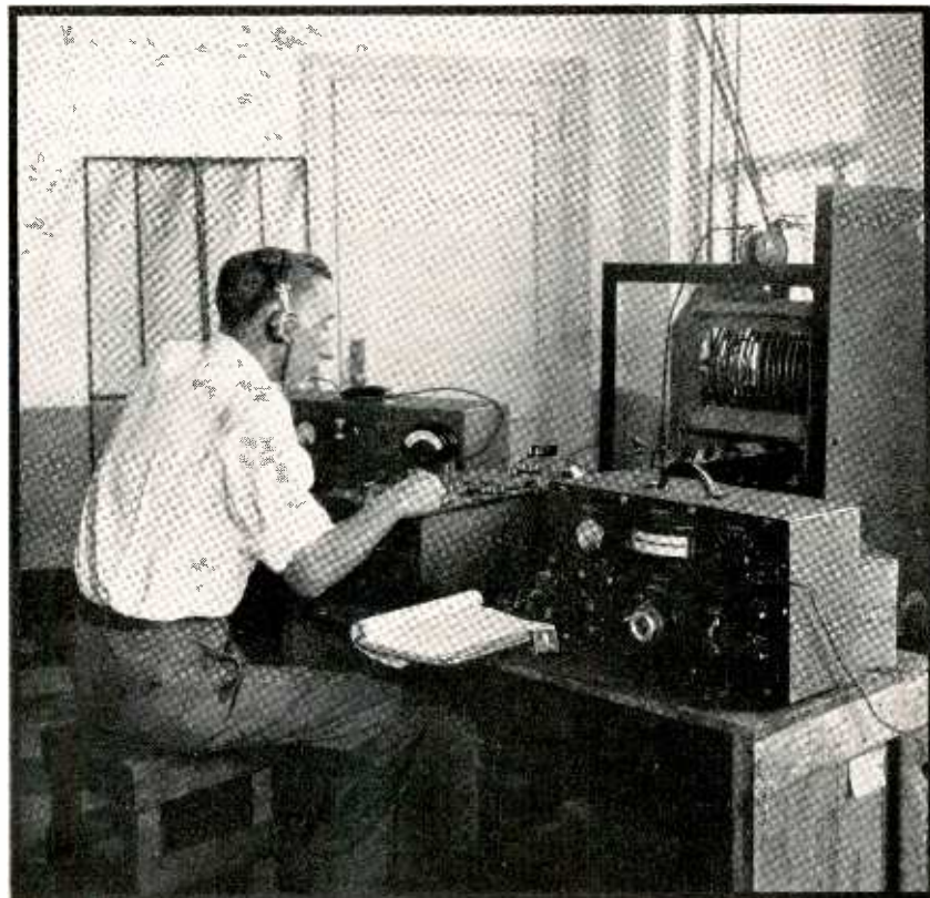
Measuring terminal impedances of lines and antennas
