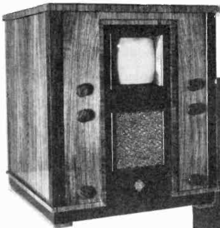
Above—Telefunken receiver — 180 lines, image 9.0 by 10.2 inches
